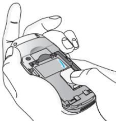
Locate the SIM card socket in the back of the phone.
