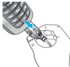
Disconnect the travel adapter from the phone by pressing its side buttons as shown in the diagram.
