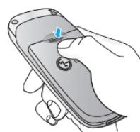
2. Then push the bottom of the battery into position until it clicks.
