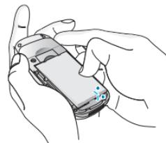
1. Position the lugs on the top of the battery into the retaining holder.
