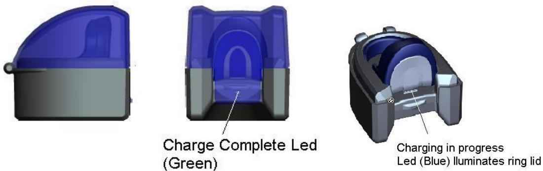
With the charger lid open, the ring is inserted straight down from overhead with the ring lid facing toward the front of the charger. A blue led will illuminate the ring lid if installed properly and charging is in progress. A green led will light at the front of the charger behind the charger lid snap.
