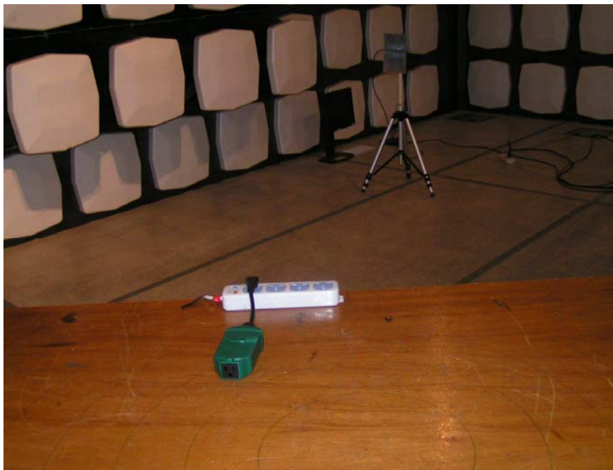
Field Strength Emissions Test Set-up – Rear View (Above 1GHz)
