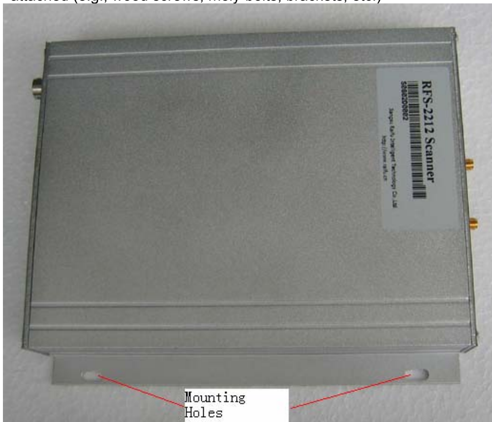
Figure 2.10 - View of the Reader showing mounting holes
