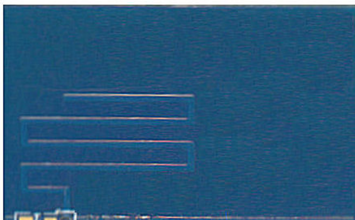
Figure 4. Part of 802.15.4 and BLE PCB with meander-like antenna (scale around 4:1)
