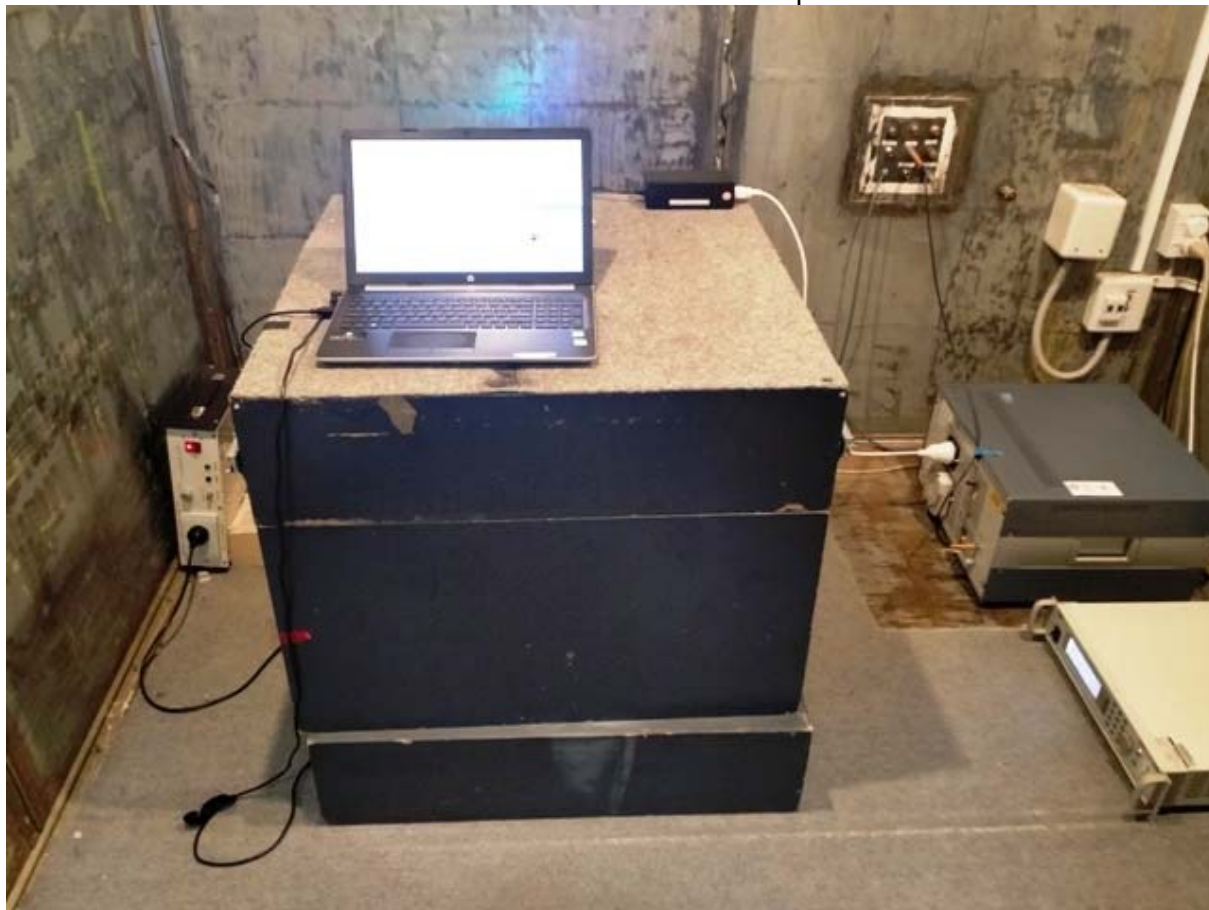
Conducted emissions test setup
