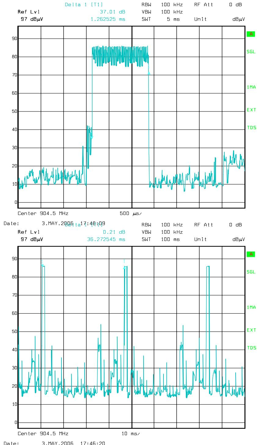
That gives a maximum of 3 transmissions in a period of 100 ms so the duel time correction factor for spurious measurement is  $20\log(3 \times 1.26/100) = -28.45 \text{ dB}$ .
