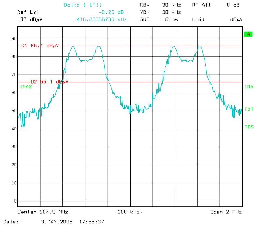
The 20dB bandwidth of each hopping channel is **417 kHz** (greater than 250 kHz and less than 500kHz)
