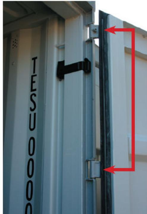
Place the CSD between these two possible locations, between the top and second hinge but not directly touching the hinges.
