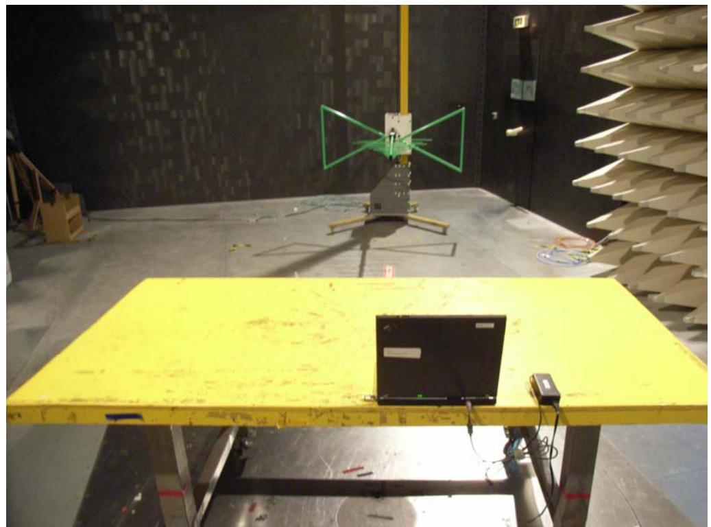
For radiated emissions from 3GHz to 5GHz
