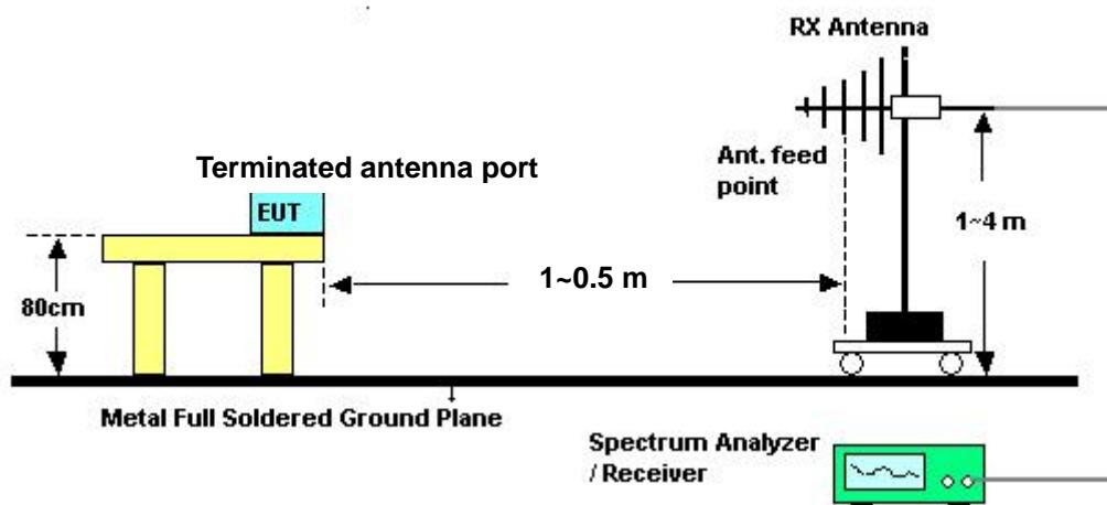
**For conducted emissions above 960MHz (Conducted antenna port measurement)**
