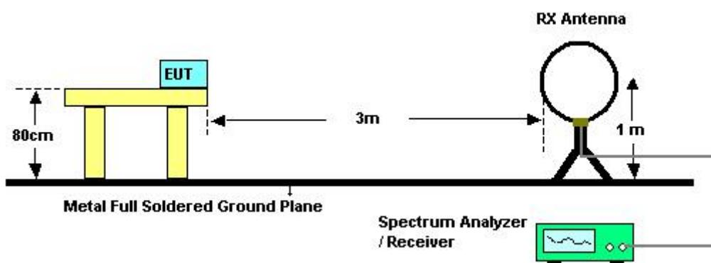
**For radiated emissions from 30MHz~960MHz**
