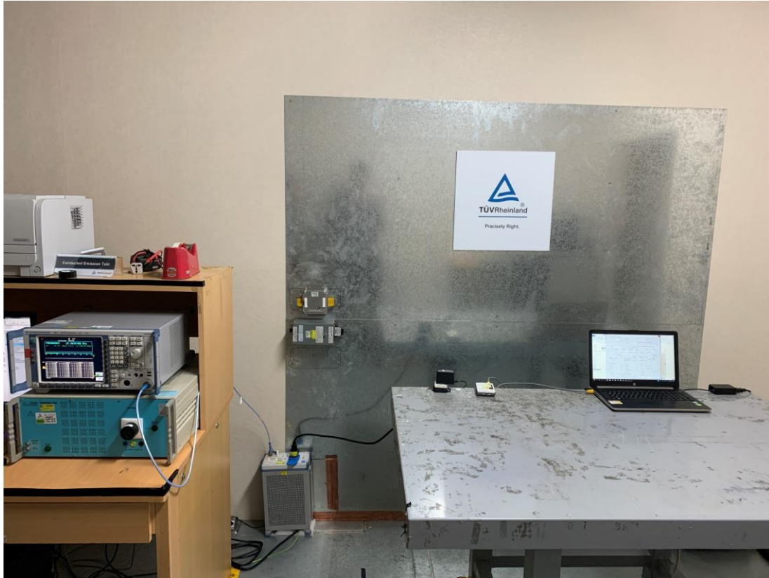
Photograph 10: Set-up for AC Mains (Back View)
