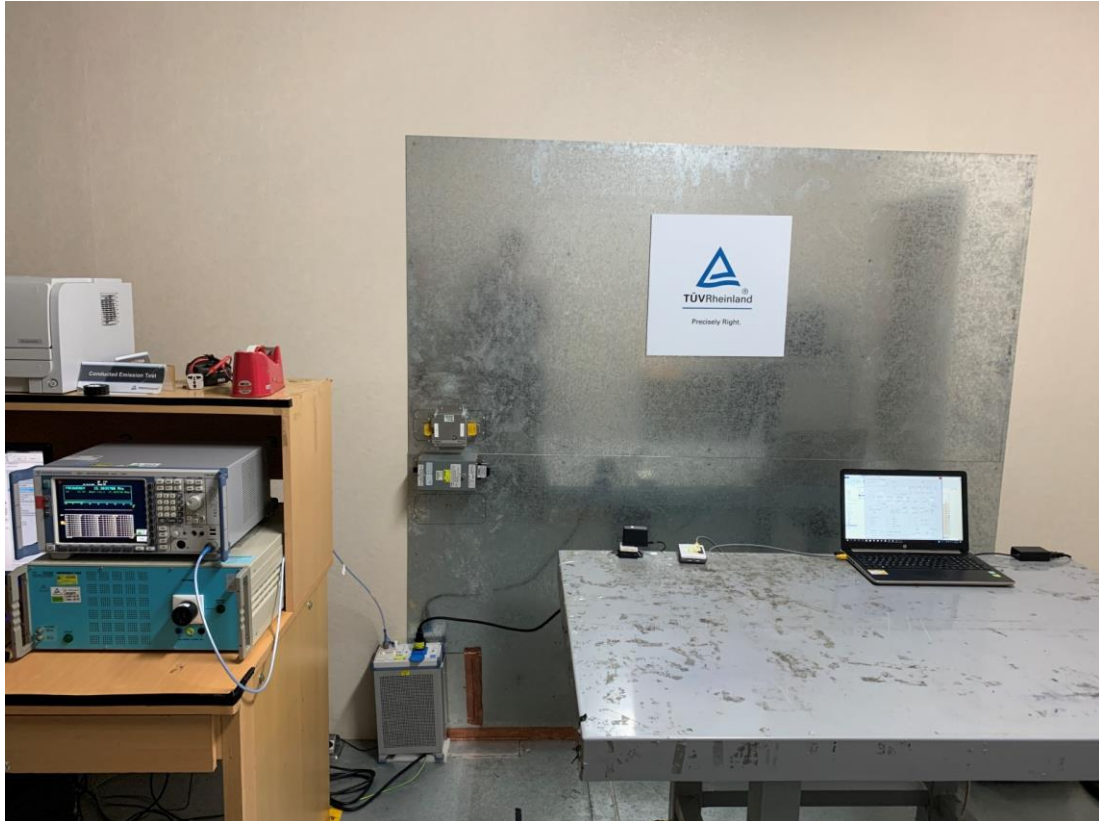
Photograph 10: Set-up for AC Mains (Back View)
