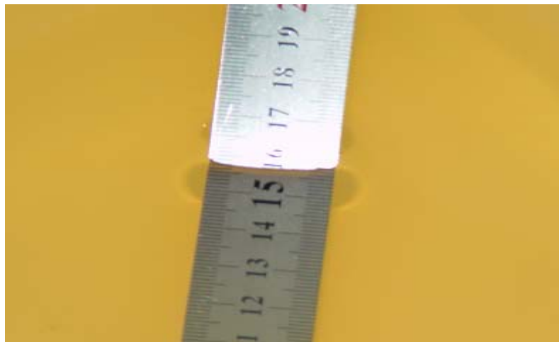
Fig40: Liquid depth for SAR Measurement
