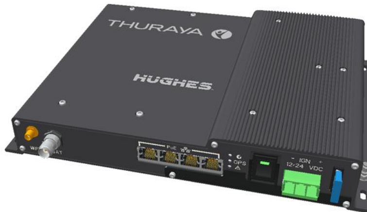
Figure 1-2. Below Decks Unit (BDU)
