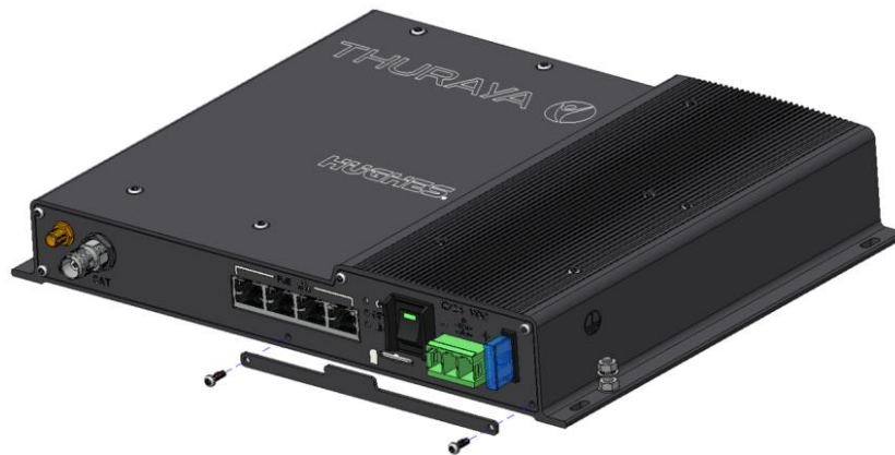
Figure 1-3. Fitting the SIM card Cover
