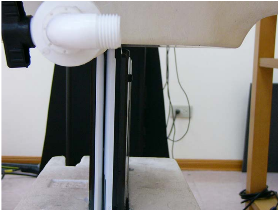
Fig.8 Right side of Notebook is paralleled with flat phantom, turn the panel outside and close it, right side is contact with flat phantom.
