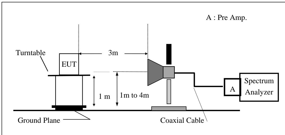
(C) Substituted Method Test Set-UP
