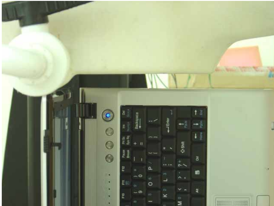
Fig.6 Right side of Notebook is paralleled with flat phantom, and spacing between EUT and Phantom-in contact 15mm.
