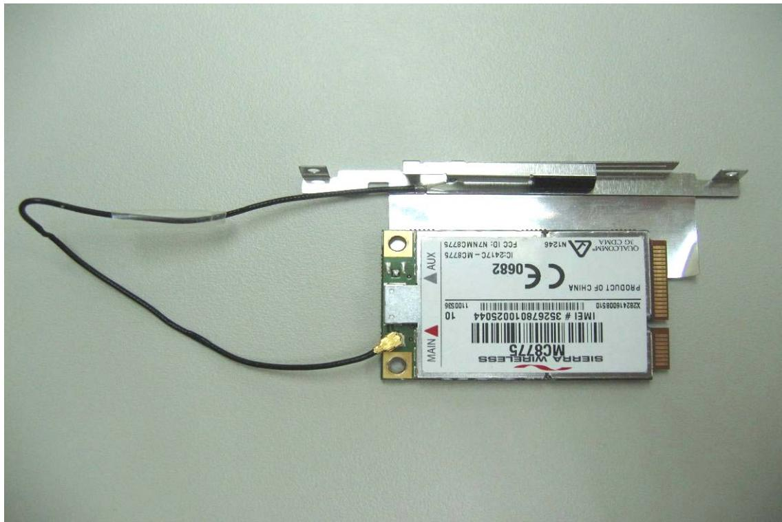
*Internal of EUT - 6 (GSM)*
