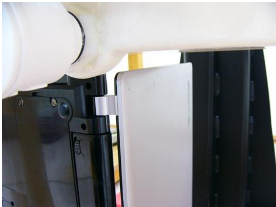
Fig.5 Photo of the right side of the LCD of Notebook is vertical with flat phantom and spacing between EUT and Phantom- in contact 15mm.
