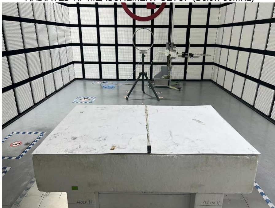
RADIATED RF MEASUREMENT SETUP (Below 30MHz)
