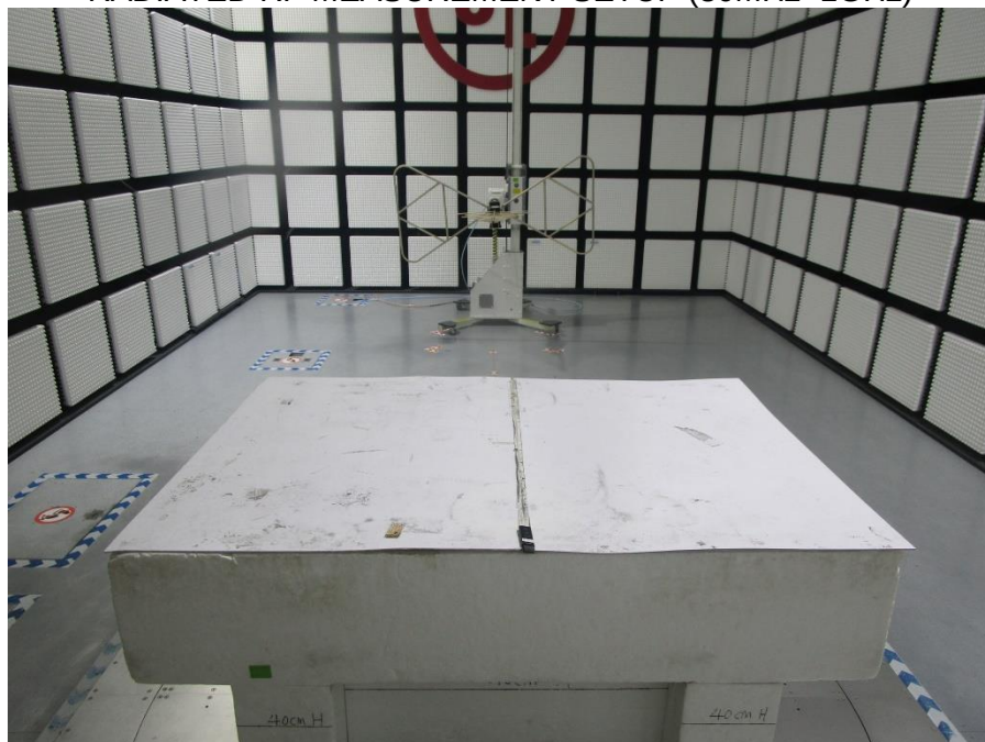
RADIATED RF MEASUREMENT SETUP (30MHz~1GHz)
