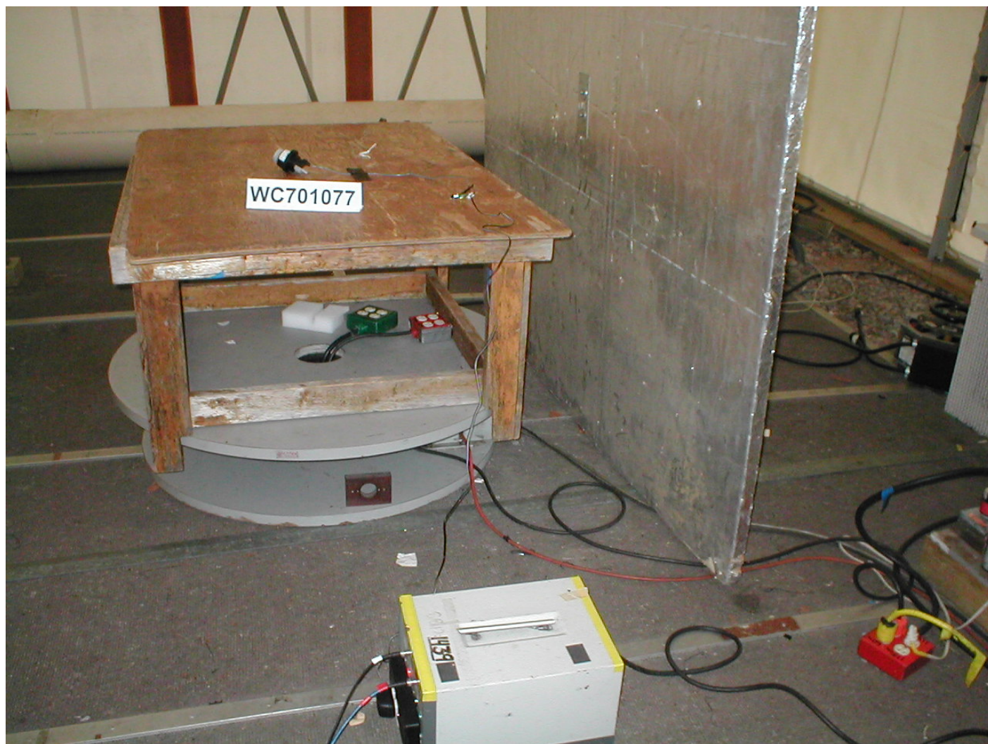
Test-setup photo(s): Conducted Emissions 150 kHz - 30 MHz
