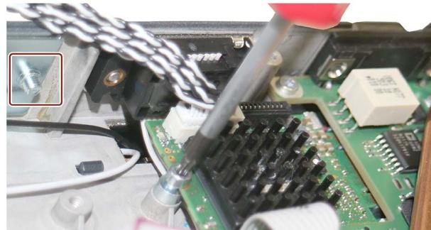
6. Place the interface board from the inside to the enclosure opening - interfaces pointing outwards and hold it with one hand.
