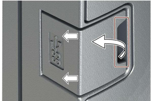
2. Turn the cover cap horizontally so that the fork lugs point downwards as marked in the figure.
