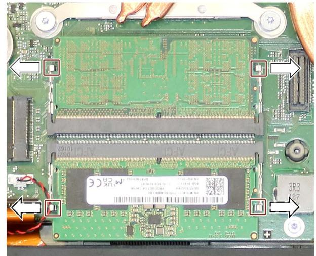
3. Pull the memory module evenly out of the slot in the 30° inclined position without tilting it.
