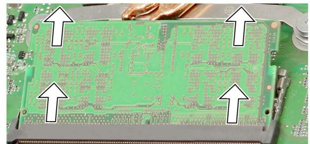
5. Push the memory module into the slot as far as it will go.
