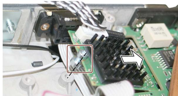
3. Use the locking screw to push the M.2 module into the slot (arrow) until the screw is above the thread (dashed line).
