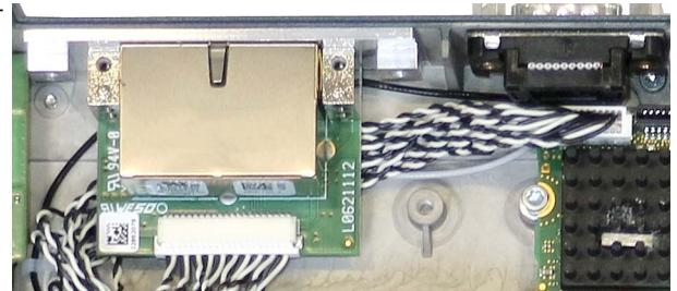
7. Screw the interface board tight from the outside (outer screws).
