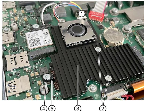
6. Pull the M.2 module in the 30° inclined position to the left out of the slot, evenly without tilting. Leave the thermal pads ⑥ on the motherboard.
