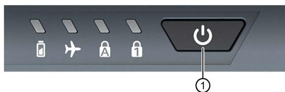
The on-off button (Power Button) ① has the following functions:
