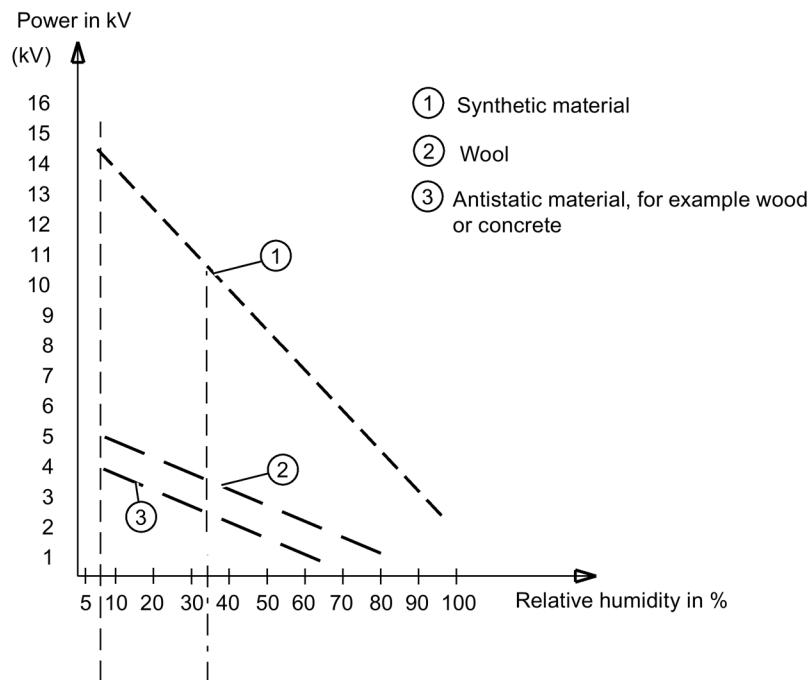
Figure 11-1 Electrostatic voltages which an operator can be subjected to
