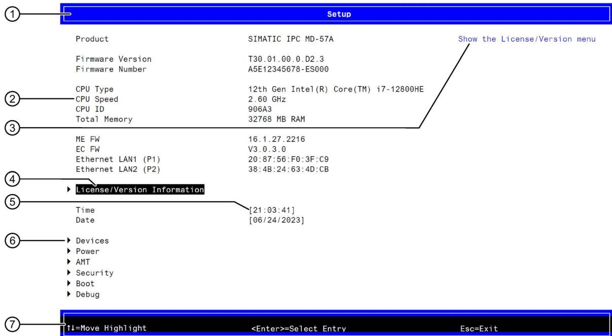
① Header The header shows where you are currently located in the BIOS, e.g. in the "Setup" menu.
