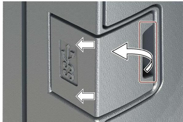
2. Insert the USB dongle into the recessed USB port.
