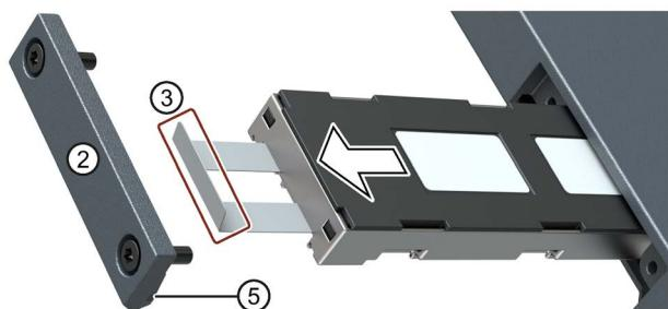
4. Push the new slider with the plug contacts (see marking) into the slide-in module until the slider audibly clicks into place.
