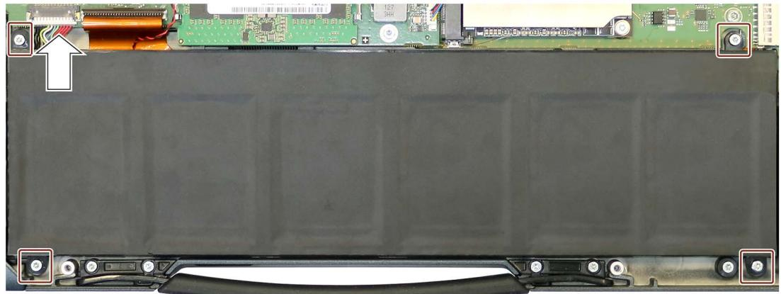
1. The connector above the battery marked with the arrow is already disconnected.
