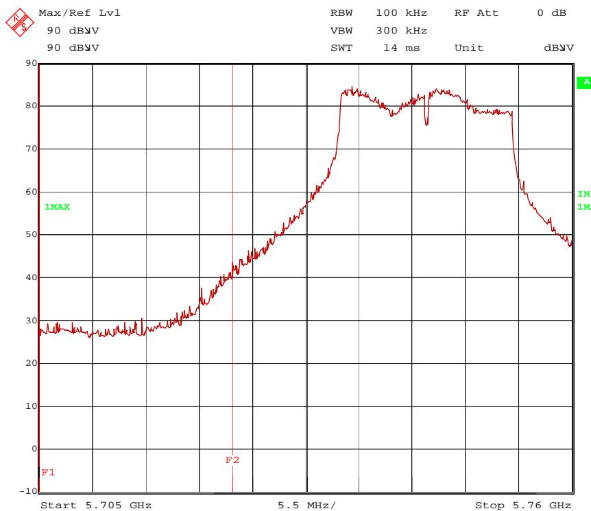
160308\_#7\_n40\_ch149\_BandEdge2\_-6dB\_90°.wmf: Band-edge compliance on channel 149 in n40 mode, BAT-ANT-N-MiMo-18N-IP65 antenna, Plot > 10 MHz to the band-edge
