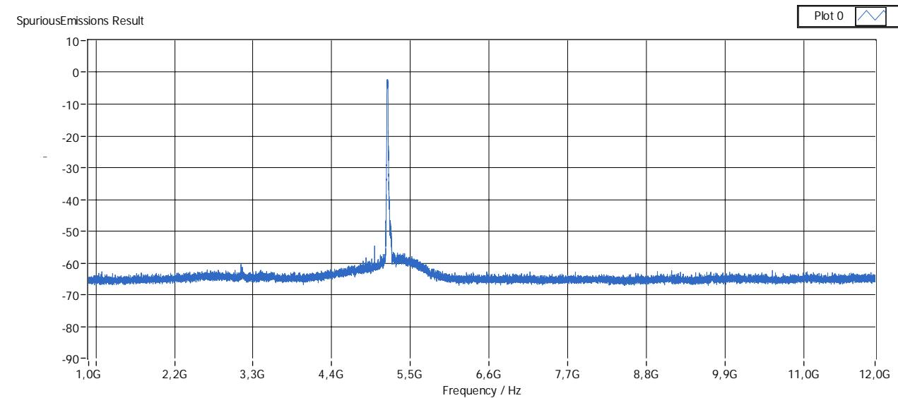
EWLAN 2\_SpurEmiss12-26G\_a\_36.emf: conducted spurious emissions (operation mode 1):
