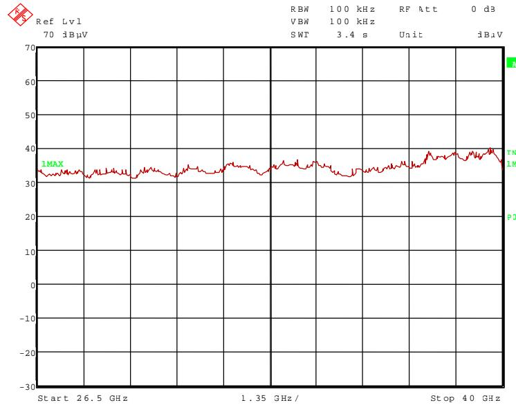
No frequencies were found inside the restricted bands during the preliminary radiated emission test.
