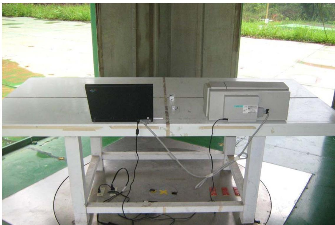
**RADIATED RF MEASUREMENT SETUP**
