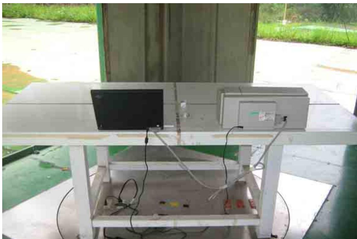
**RADIATED RF MEASUREMENT SETUP**
