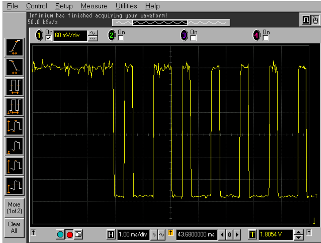
Figure 3 showing 400 \mu Sec bit length (Waveform is inverted)
