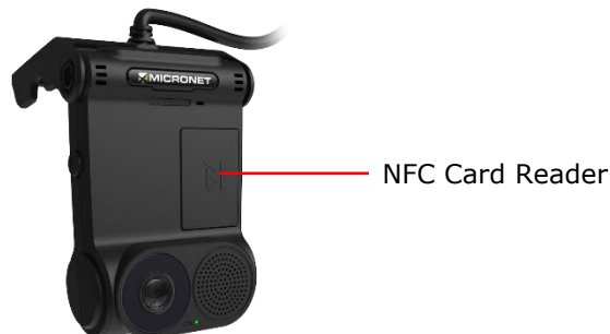
Figure 4: SmartCAM™ NFC Proximity Reader Area
