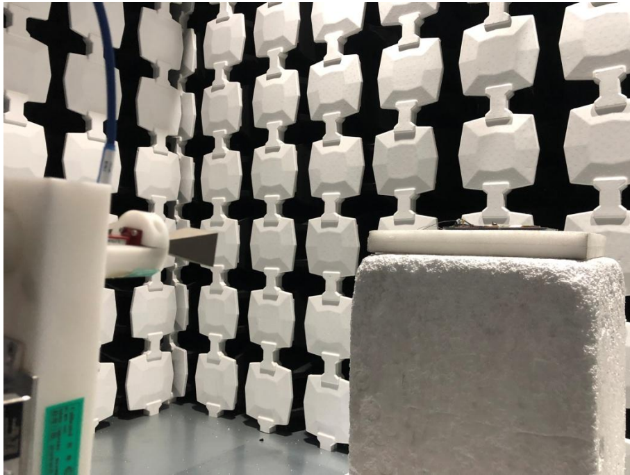
Description: Radiated Emission Test Setup (Above 18GHz)
