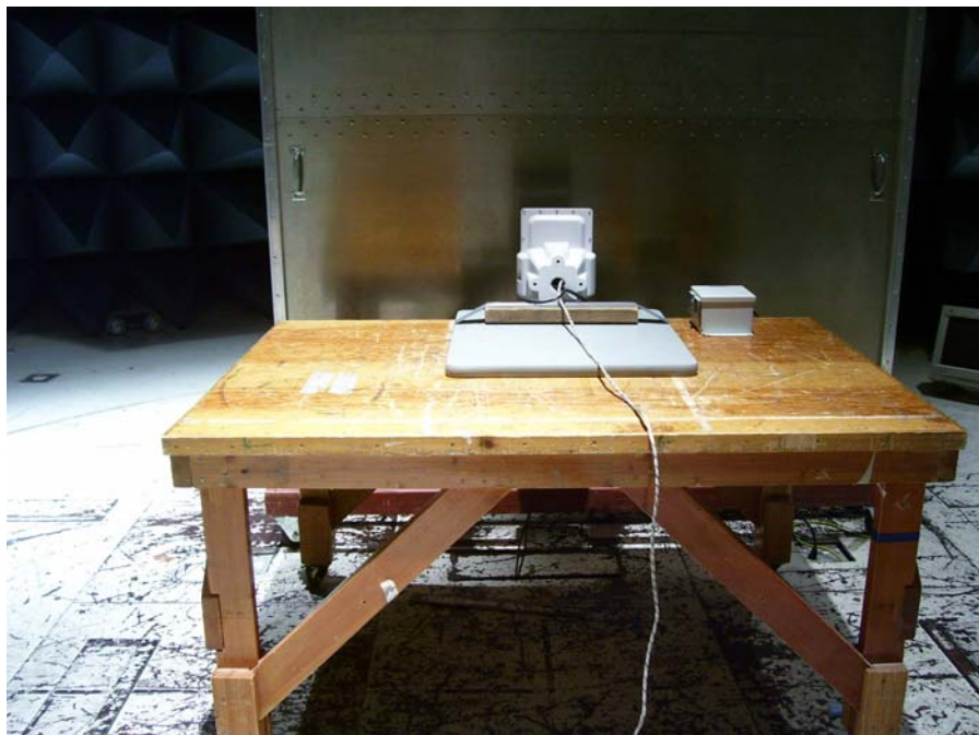
Photograph 5. Conducted Emissions Test Setup, EW 5301 CEV w 24V AC PSU (Front)
