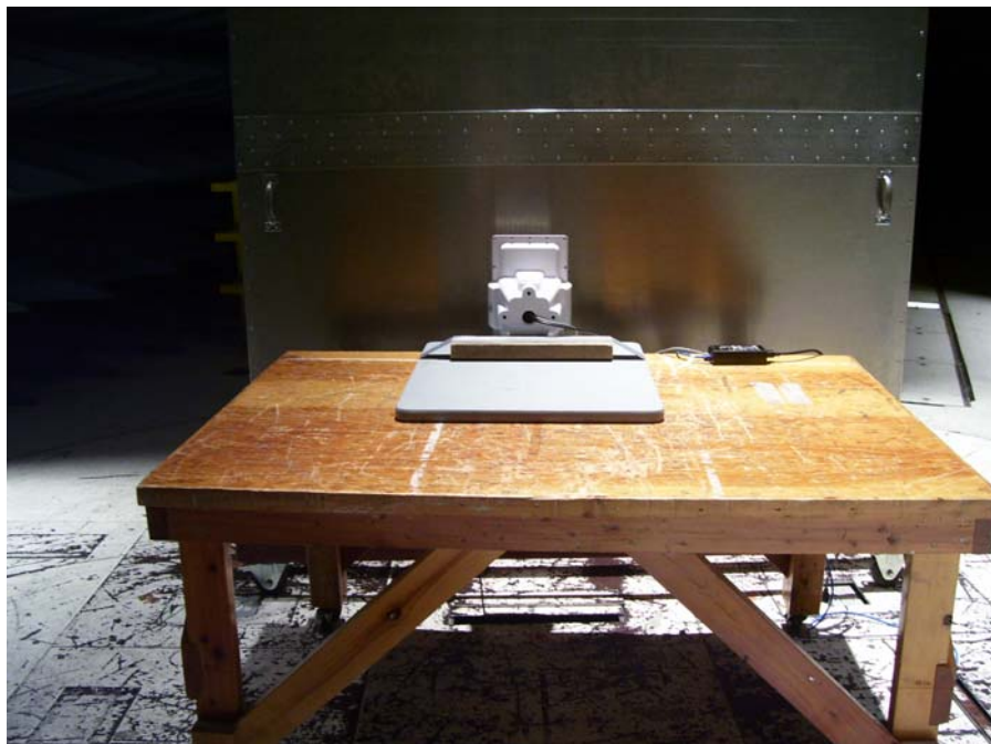
Photograph 3. Conducted Emissions Test Setup, EW 5002 CEV w 48V DC POE PSU (Front)
