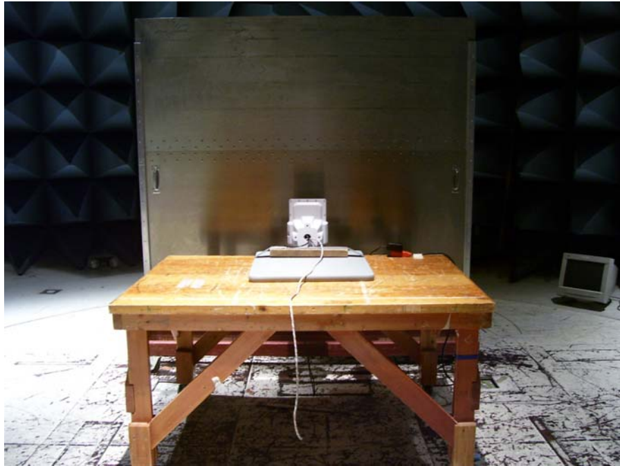
Photograph 4. Conducted Emissions Test Setup, EW 5301 CEV w 12V DC PSU (Front)
