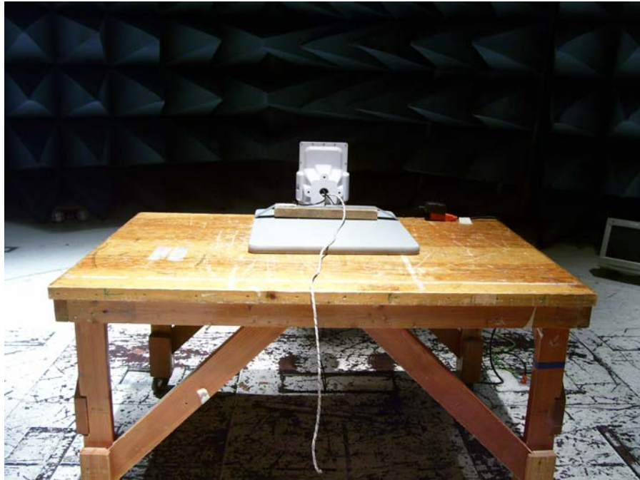
Photograph 8. Radiated Emission Test Setup 30 MHz - 1 GHz, EW 5301 w 12V DC PSU (close-up)
