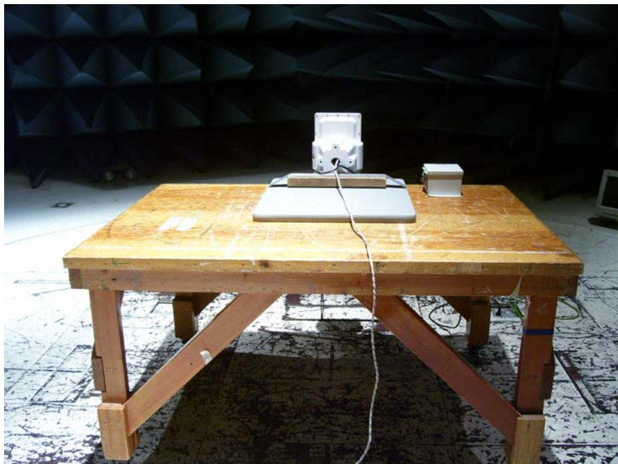
Photograph 9. Radiated Emission Test Setup 30 MHz - 1 GHz, EW 5301 w 24V AC PSU (close-up)
