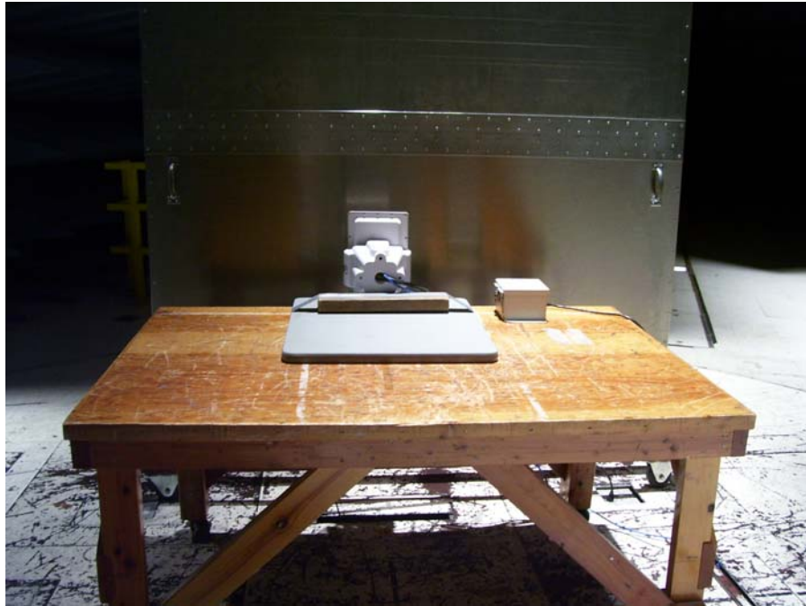
Photograph 2. Conducted Emissions Test Setup, EW 5002 CEV w 24V AC PSU (Front)
