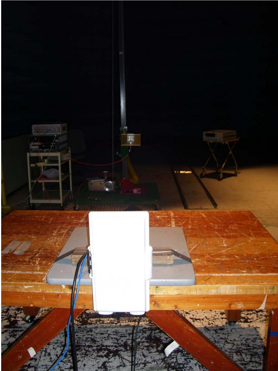
Photograph 11. Radiated Emission Limits Test Setup 1 - 5GHz, EW 5002 w 48V DC POE PSU (Back)
