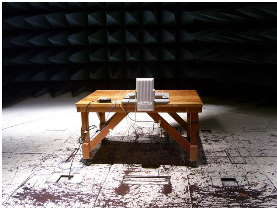
Photograph 7. Radiated Emission Test Setup 30 MHz - 1 GHz, EW 5002 w 48V DC POE PSU (close-up)
