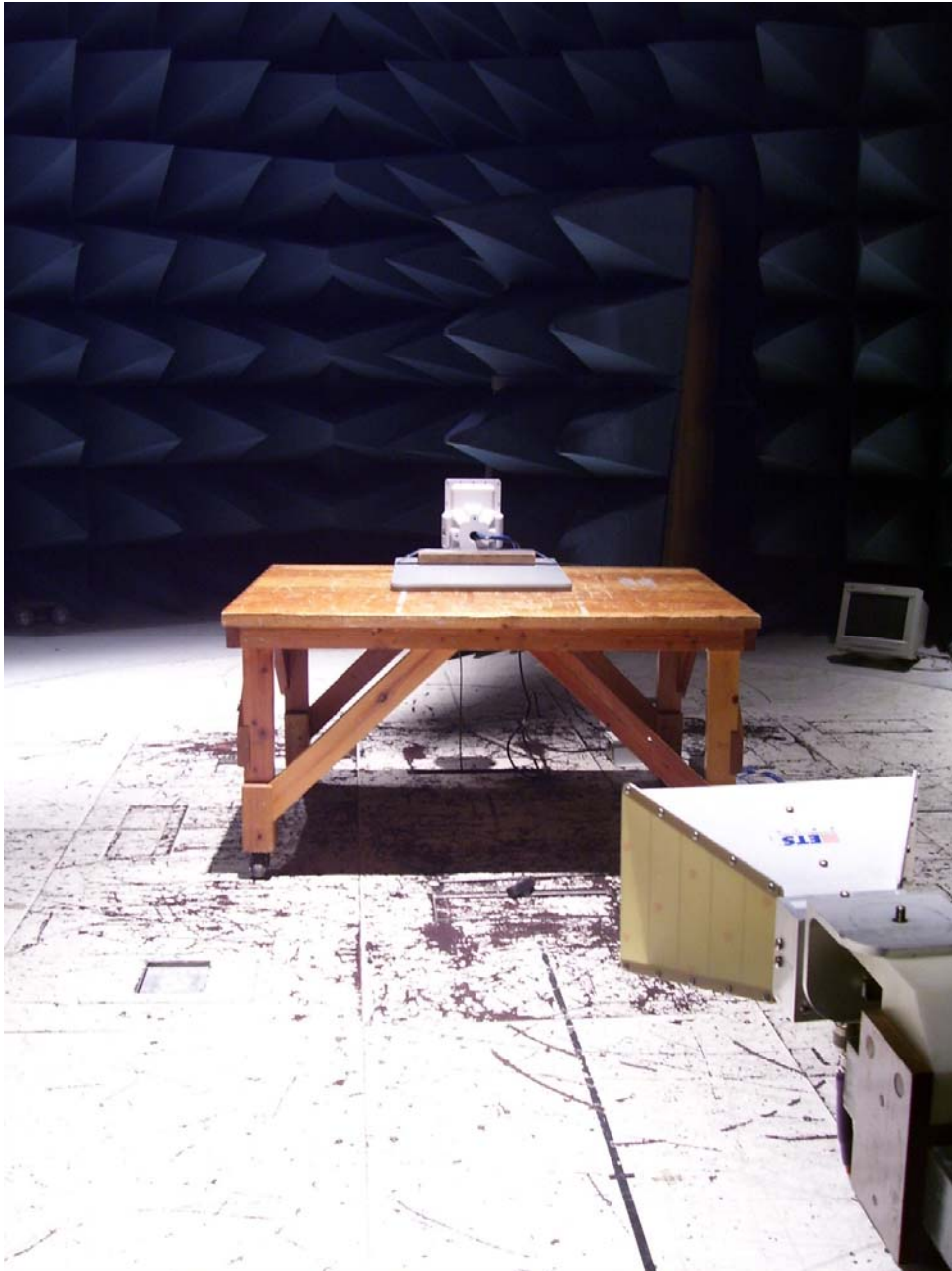
Photograph 10. Radiated Emission Limits Test Setup 1 - 5GHz, EW 5002 w 24V AC PSU (Front)
