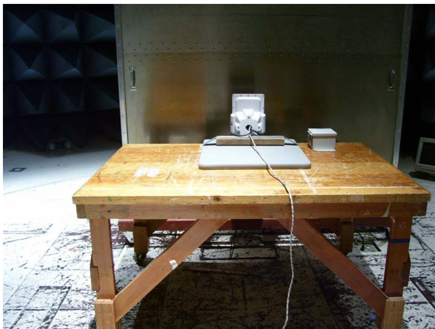
Photograph 15. Conducted Emissions Test Setup, EW 5301 CEV w 24V AC PSU (Front)
