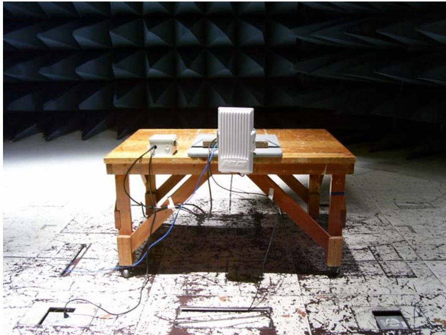
Photograph 6. Radiated Emission Test Setup 30 MHz - 1 GHz, EW 5002 w 24V AC PSU (close-up)
