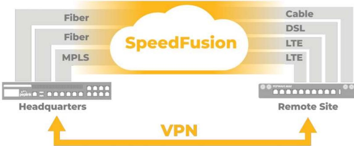
Pepwave bandwidth bonding SpeedFusion™ is our patented technology that enables our SD-WAN routers to bond multiple Internet connections to increase site-to-site bandwidth and reliability. SpeedFusion functionality securely connects your Pepwave router to another Pepwave or Peplink device (Peplink Balance 210/310/380/580/710/1350 only). Data, voice, or video communications between these locations are kept confidential across the public Internet.
