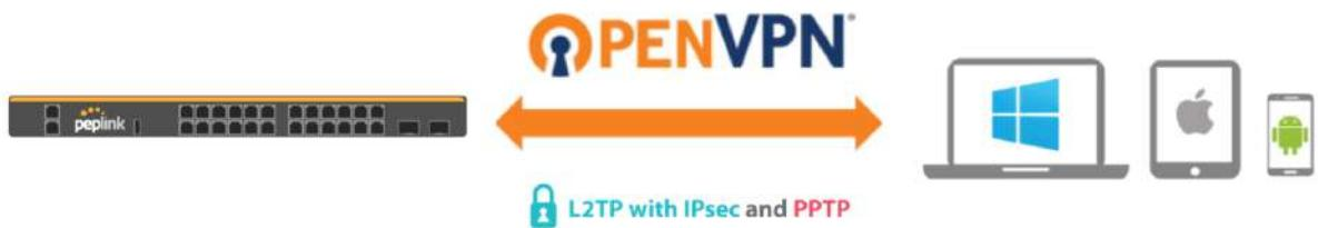
Use OpenVPN or L2TP with IPsec to safely and conveniently connect remote clients to your private network. L2TP with IPsec is supported by most devices, but legacy devices can also connect using PPTP.
