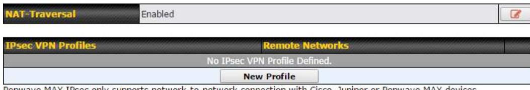
A **NAT-Traversal** option and list of defined **IPsec VPN** profiles will be shown. **NAT-Traversal** should be enabled if your system is behind a NAT router. Click the **New Profile** button to create new IPsec VPN profiles that make VPN connections to remote Pepwave, Cisco, or Juniper routers via available WAN connections. To edit any of the profiles, click on its associated connection name in the leftmost column.
