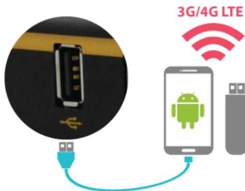
For increased WAN diversity, plug in a USB LTE modem as a backup. Peplink routers are compatible with over [200 modem types](#). You can also tether to smartphones running Android 4.1.X and above.
