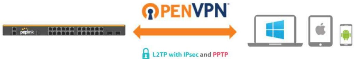
Use OpenVPN or L2TP with IPsec to safely and conveniently connect remote clients to your private network. L2TP with IPsec is supported by most devices, but legacy devices can also connect using PPTP.
