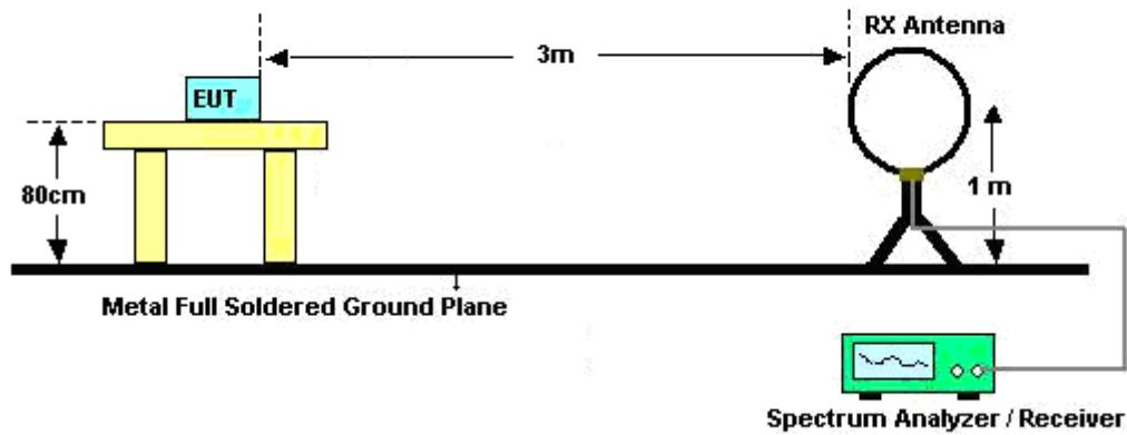
For radiated emissions from 30MHz to 1GHz
