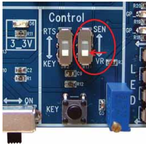
< Figure 7-1-4-(2)-① VR / SEN selection switch – Select VR >
