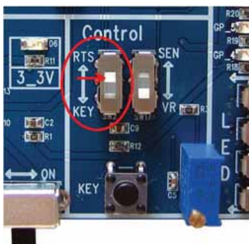
< Figure 7-1-4-(1)-② KEY / RTS selection switch – Select RTS >
