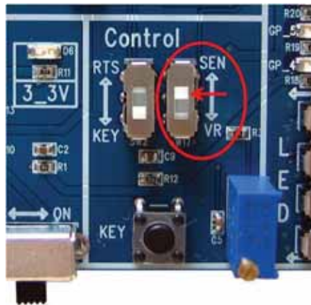
< Figure 7-1-12-② Set-up for using ADC port as extension port >
