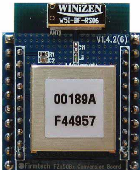
< Figure 7-1-12-⑩ 2.54mm(100mil) Mounting Convertible Board >
