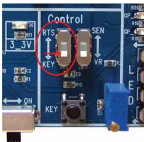
< Figure 7-1-4-(1)-① KEY / RTS selection switch – Select KEY >
