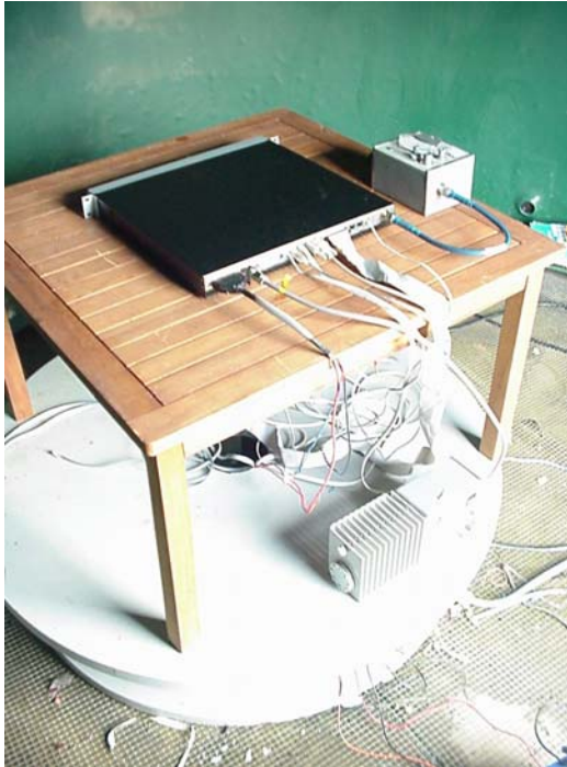
Radiated emissions test set up
