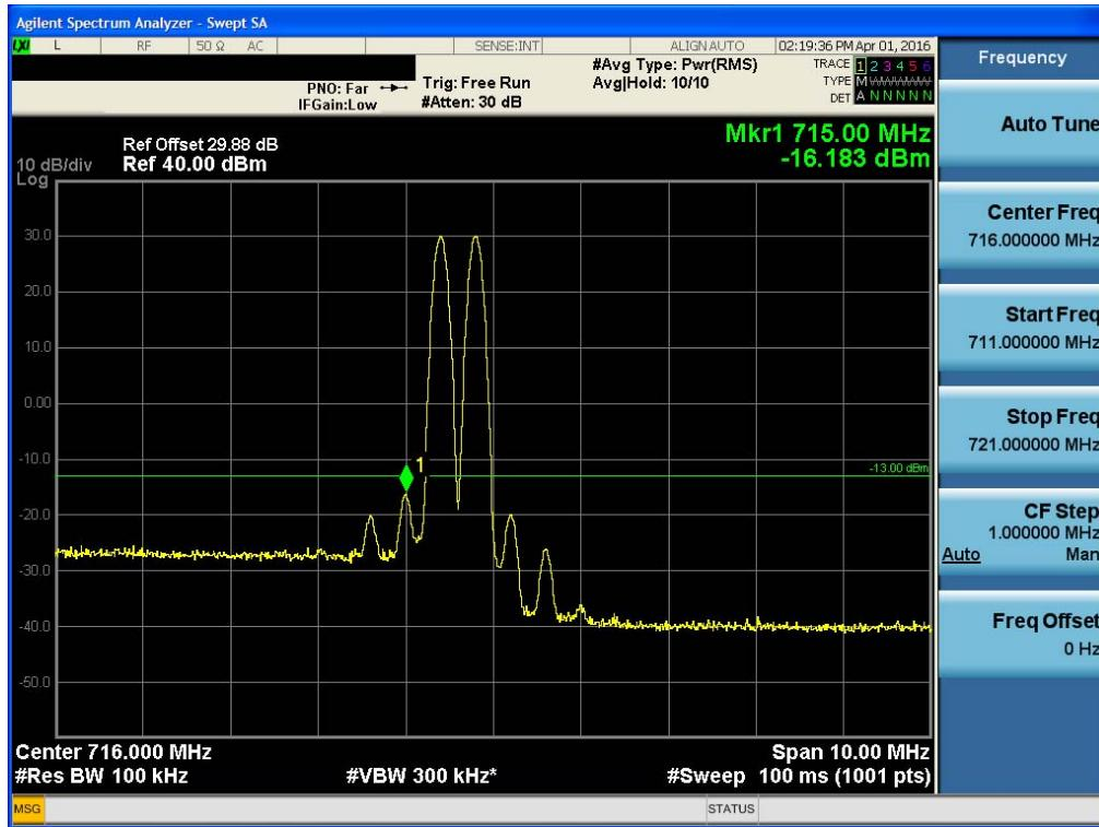
**Multi channel Enhancer Band Edge for IC\_Uplink LTE 10 MHz**
