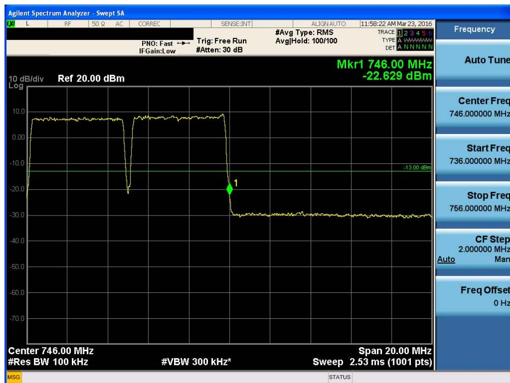
**Intermodulation Spurious Emissions for FCC\_LTE 10 MHz Downlink**
