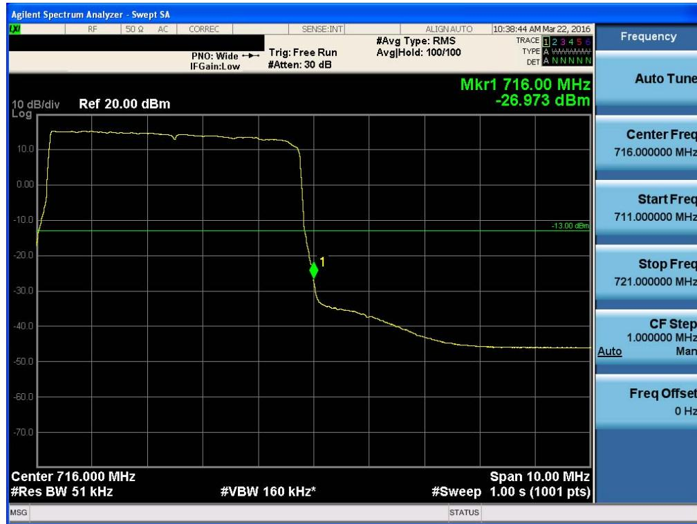
**Single channel Enhancer Band Edge\_Uplink LTE 10 MHz**
