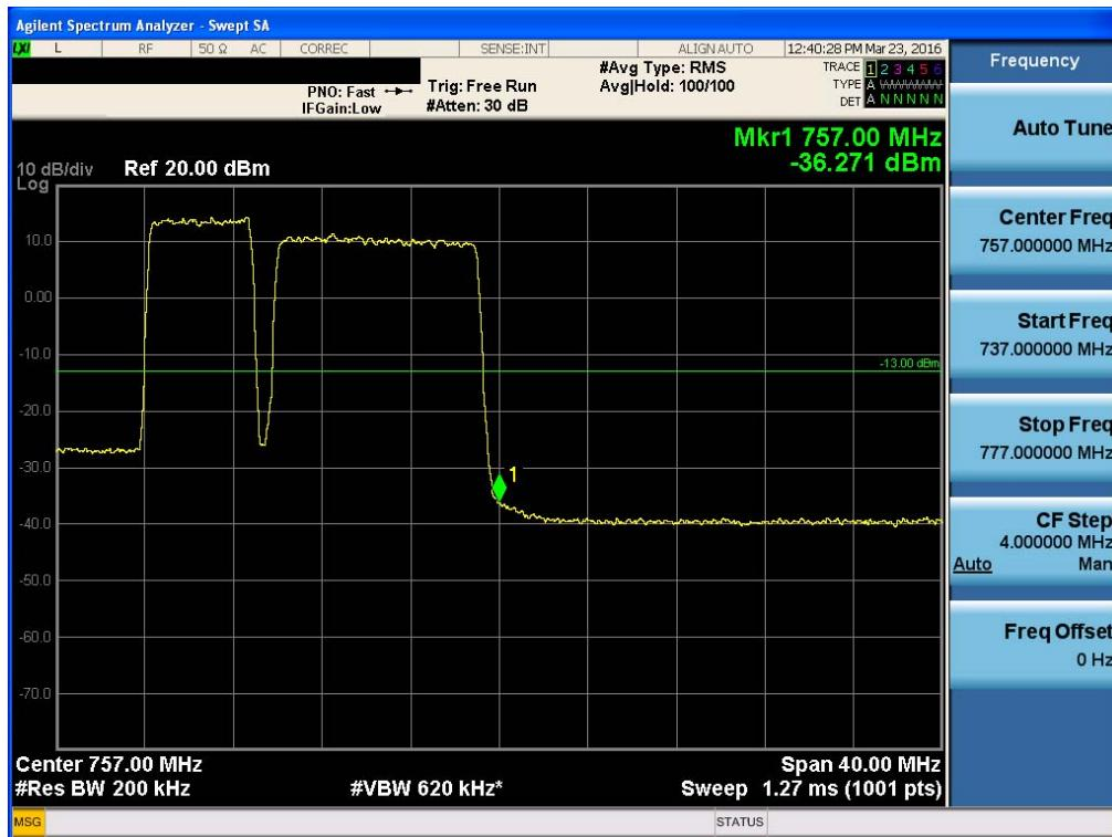
**Intermodulation Spurious Emissions for FCC\_LTE 5 MHz Uplink**
