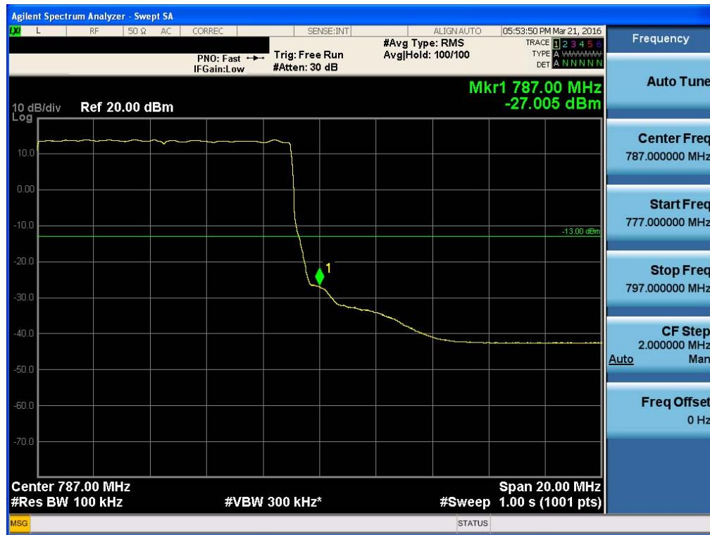
**Multi channel Enhancer Band Edge for IC\_Downlink LTE 5 MHz**
