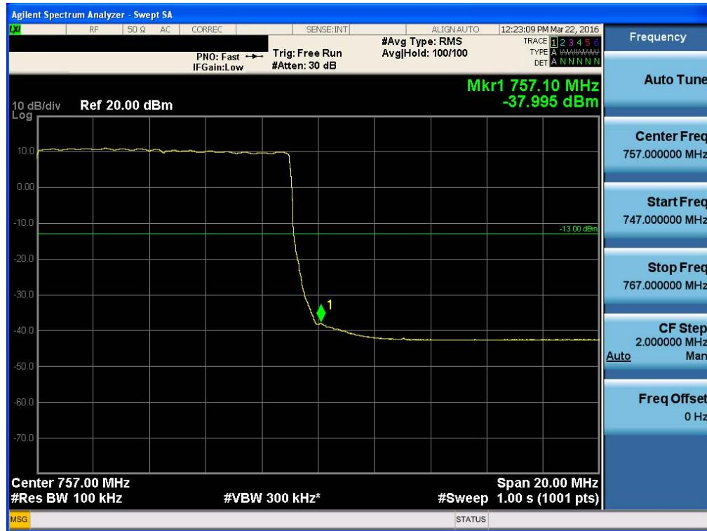
**Single channel Enhancer Band Edge\_Uplink LTE 5 MHz**
