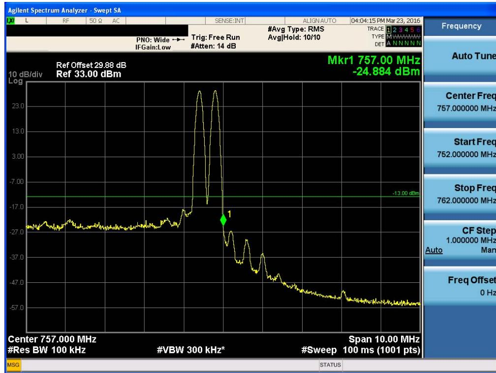
**Multi channel Enhancer Band Edge for IC\_Uplink LTE 5 MHz**
