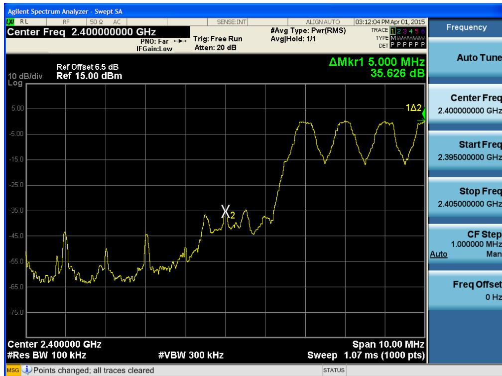
Test Plots with hopping (GFSK)
