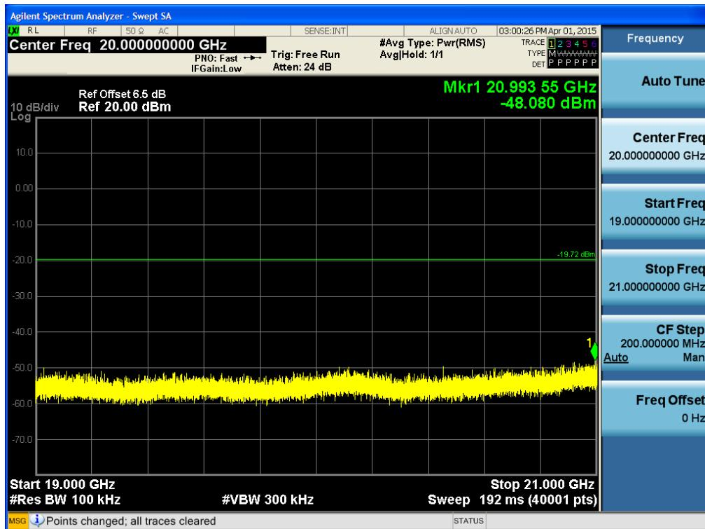
Test Plots (8DPSK)- 21 GHz - 23 GHz
