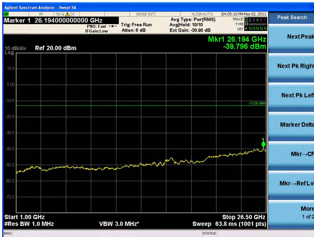
Conducted Spurious Emissions Downlink High CH (1 GHz – 26.5 GHz)
