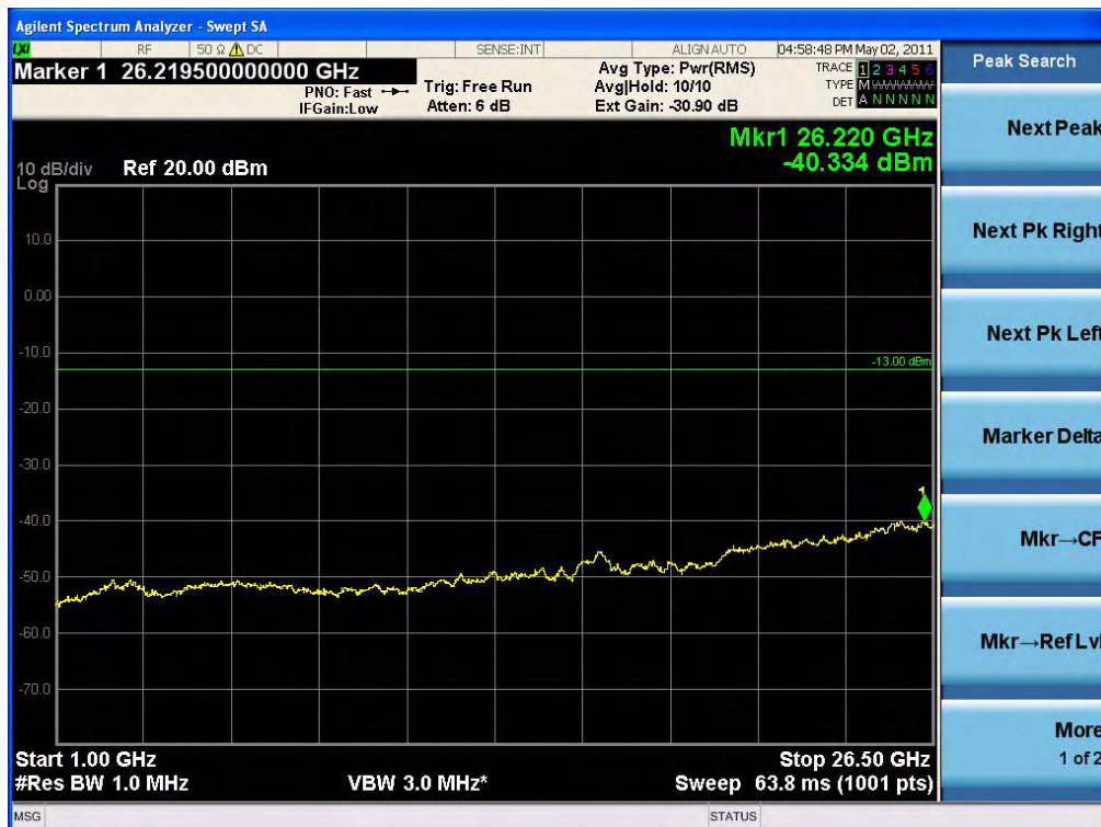
Conducted Spurious Emissions Uplink Mid CH (1 GHz – 26.5 GHz)
