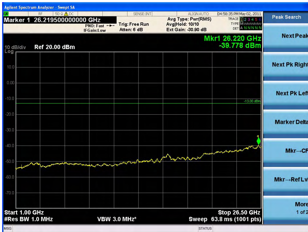
Conducted Spurious Emissions Uplink Low CH (1 GHz – 26.5 GHz)
