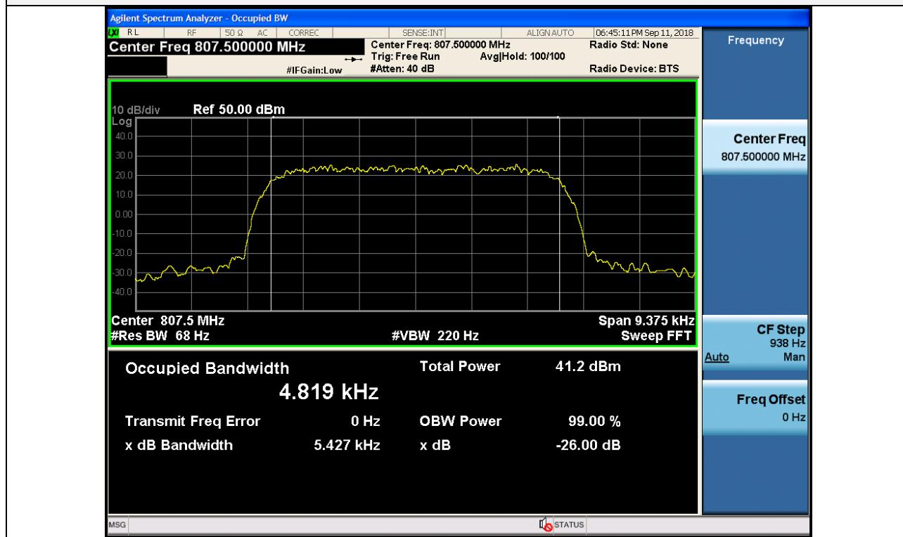
3 dB above the AGC threshold Output / NPSPAC / Downlink / P25 Phase 1
