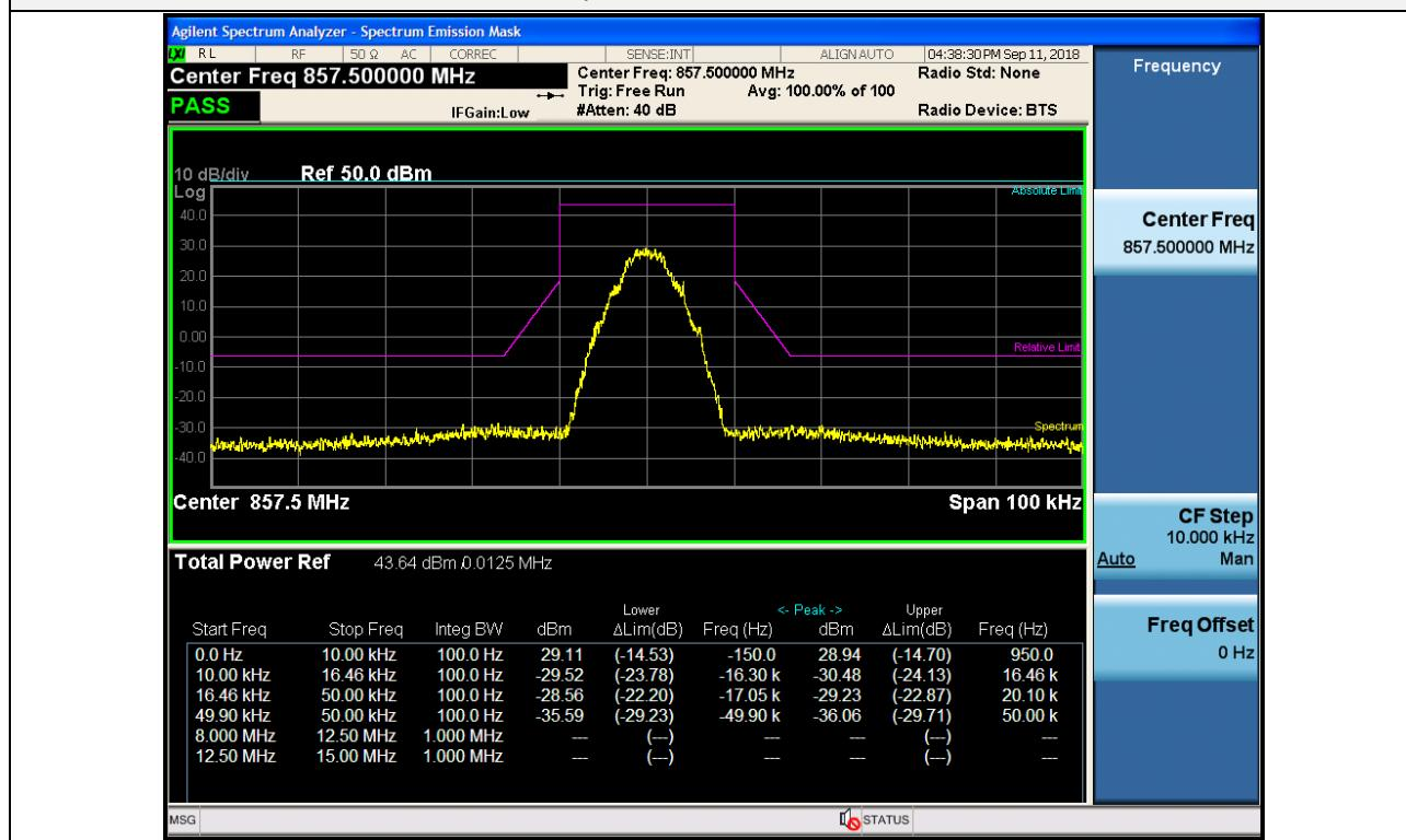
3 dB above the AGC threshold Output / PS B/ILT SMR / Downlink / P25 Phase 2 / Mask G
