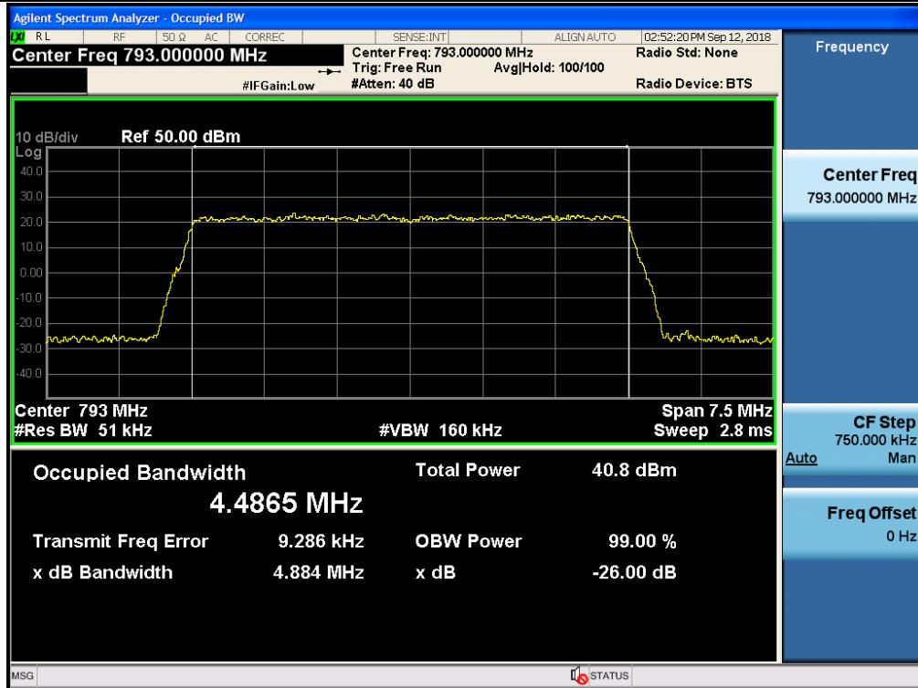
3 dB above the AGC threshold Output / PS Broadband / Uplink / LTE 10 MHz
