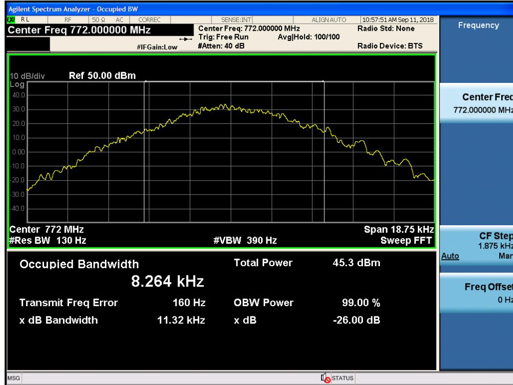
3 dB above the AGC threshold Output / PS Narrowband / Downlink / P25 Phase 2
