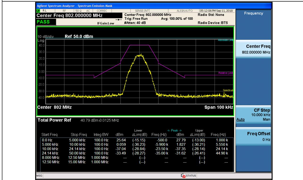
3 dB above the AGC threshold Output / PS Narrowband / Uplink / P25 Phase 2 / Mask C
