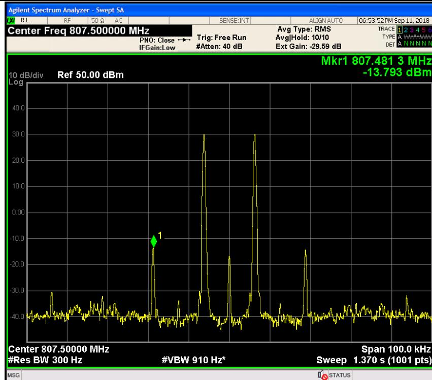
3 dB above the AGC threshold Output Intermodulation / NPSPAC / Downlink / 12.5 kHz
