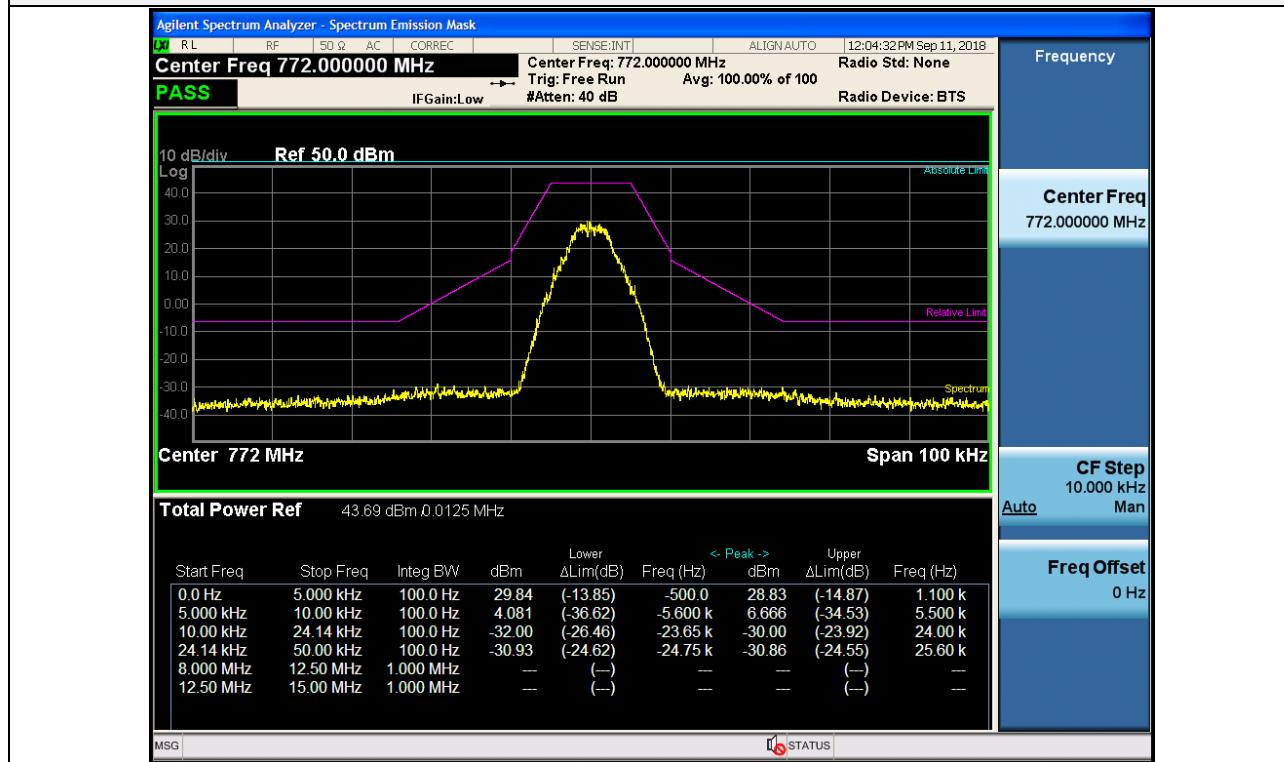
3 dB above the AGC threshold Output / PS Narrowband / Downlink / P25 Phase 2 / Mask C
