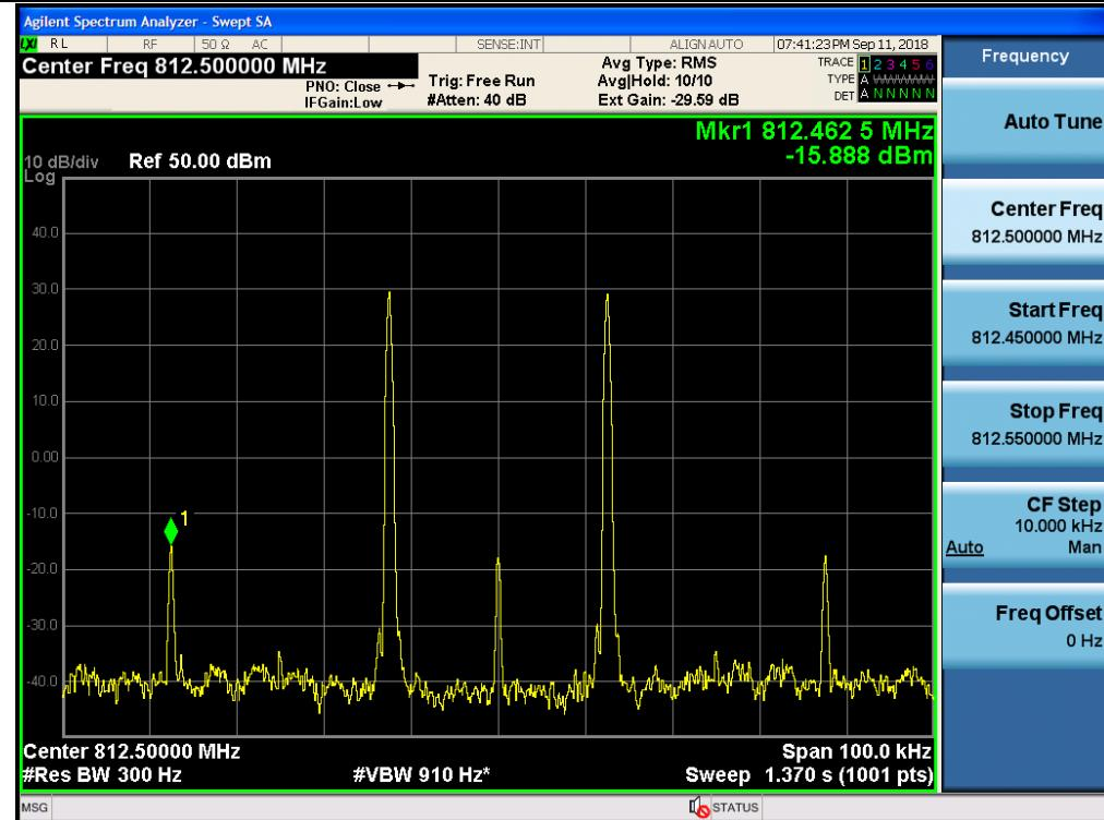
3 dB above the AGC threshold Output Intermodulation / PS B/ILT SMR / Downlink / 25 kHz
