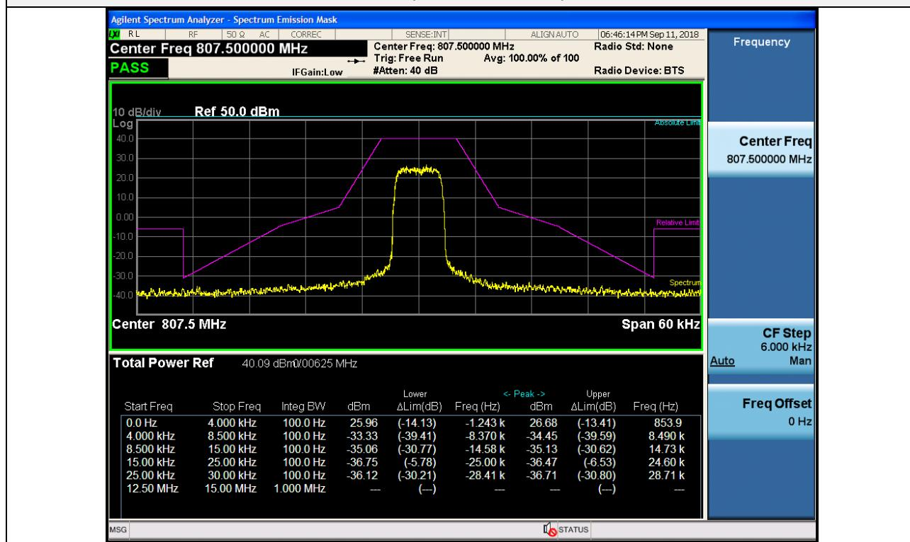
3 dB above the AGC threshold Output / NPSPAC / Downlink / P25 Phase 1 / Mask H
