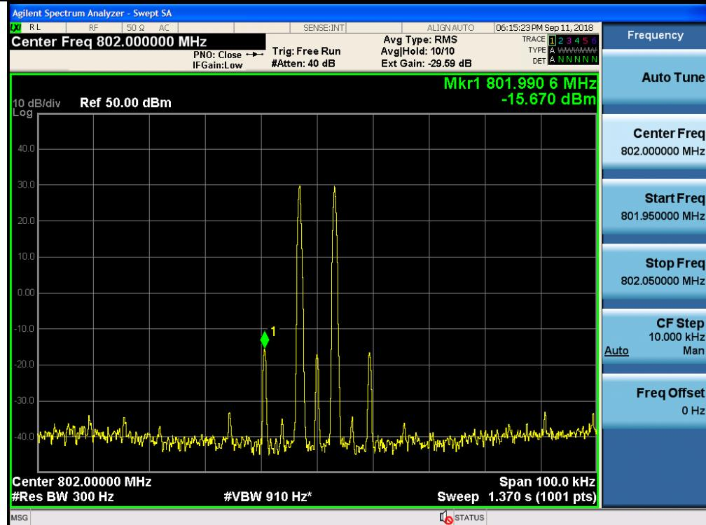
3 dB above the AGC threshold Output Intermodulation / PS Narrowband / Downlink / 12.5 kHz
