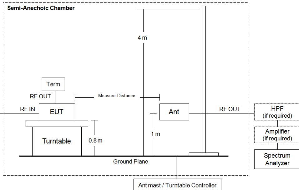
\* EUT position is adopted by placement of wall-mounted refer to section 6.3.5 of ANSI C63.4-2014
