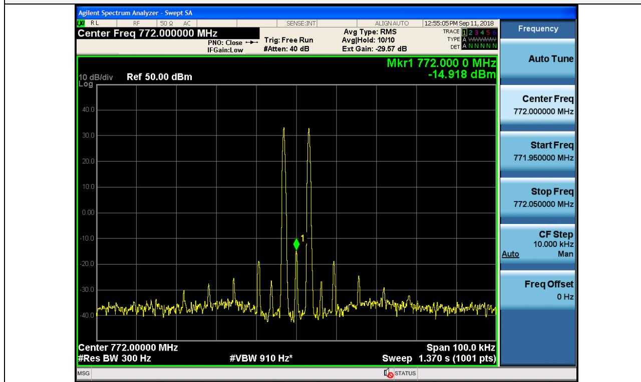
3 dB above the AGC threshold Output Intermodulation / NPSPAC / Uplink / 12.5 kHz
