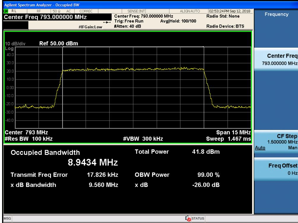
3 dB above the AGC threshold Output / PS Broadband / Downlink / LTE 5 MHz
