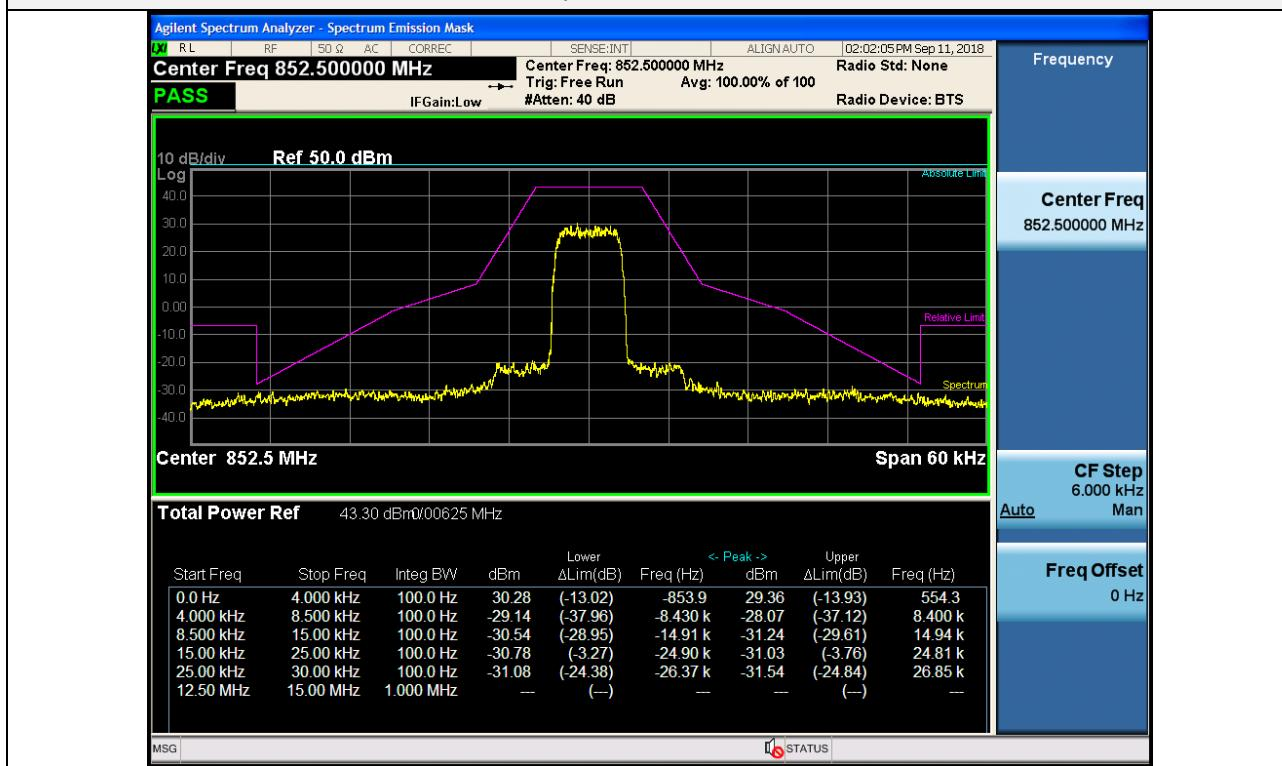
3 dB above the AGC threshold Output / PS B/ILT SMR / Uplink / P25 Phase 1 / Mask G
