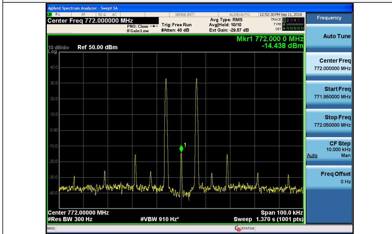
3 dB above the AGC threshold Output Intermodulation / PS Narrowband / Downlink / 6.25 kHz
