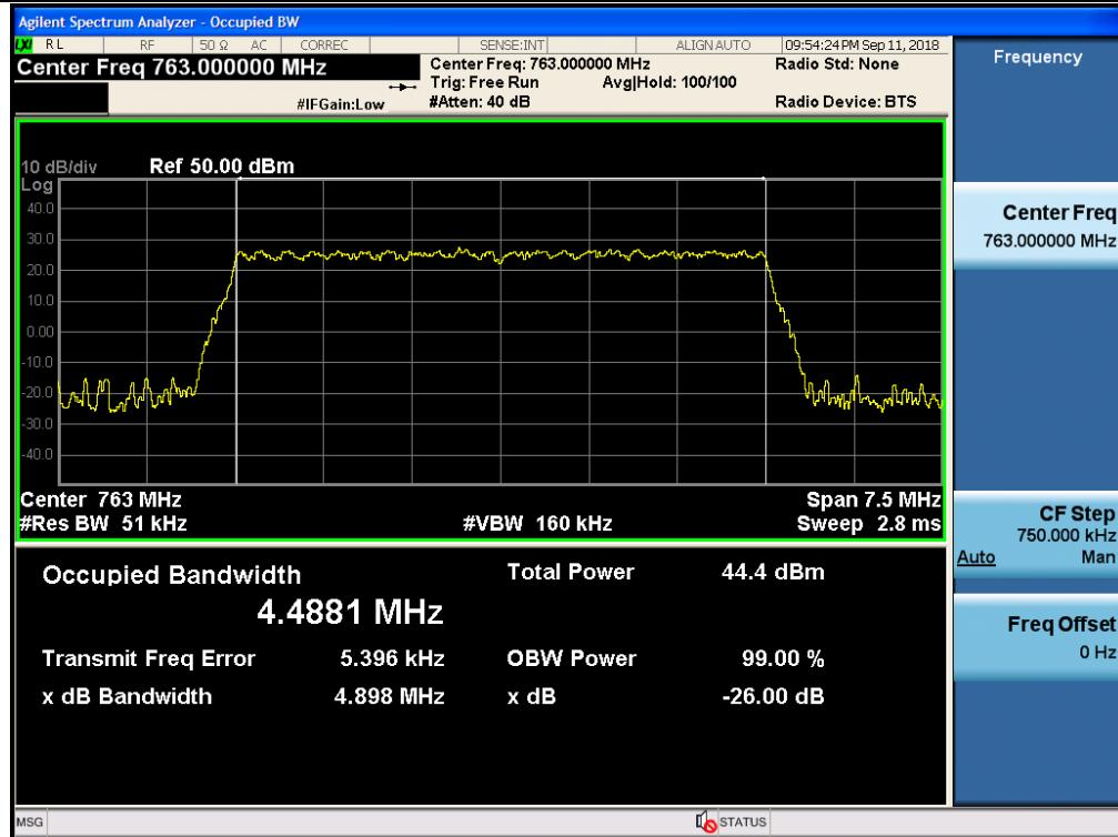
3 dB above the AGC threshold Output / PS Broadband / Downlink / LTE 10 MHz
