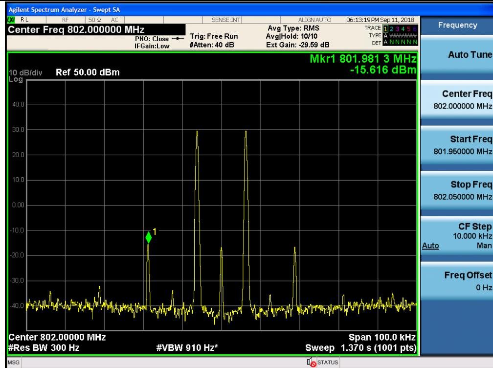
3 dB above the AGC threshold Output Intermodulation / PS Narrowband / Uplink / 6.25 kHz
