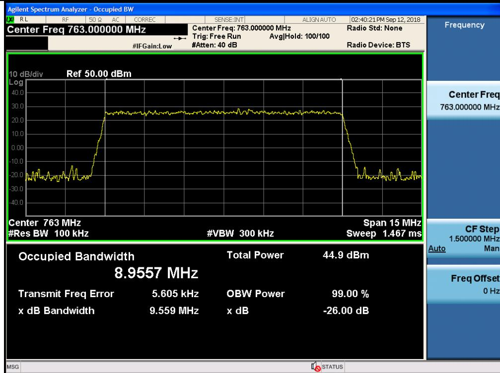
3 dB above the AGC threshold Output / PS Narrowband / Uplink / P25 Phase 1
