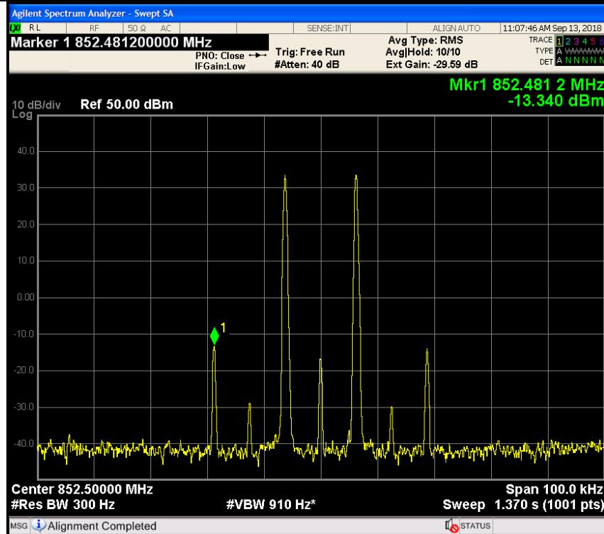
3 dB above the AGC threshold Output Intermodulation / PS B/ILT SMR / Uplink / 25 kHz
