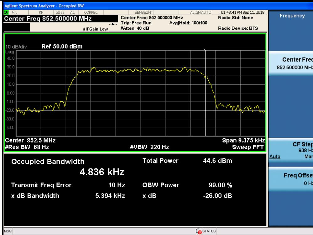
3 dB above the AGC threshold Output / PS B/ILT SMR / Uplink / P25 Phase 1
