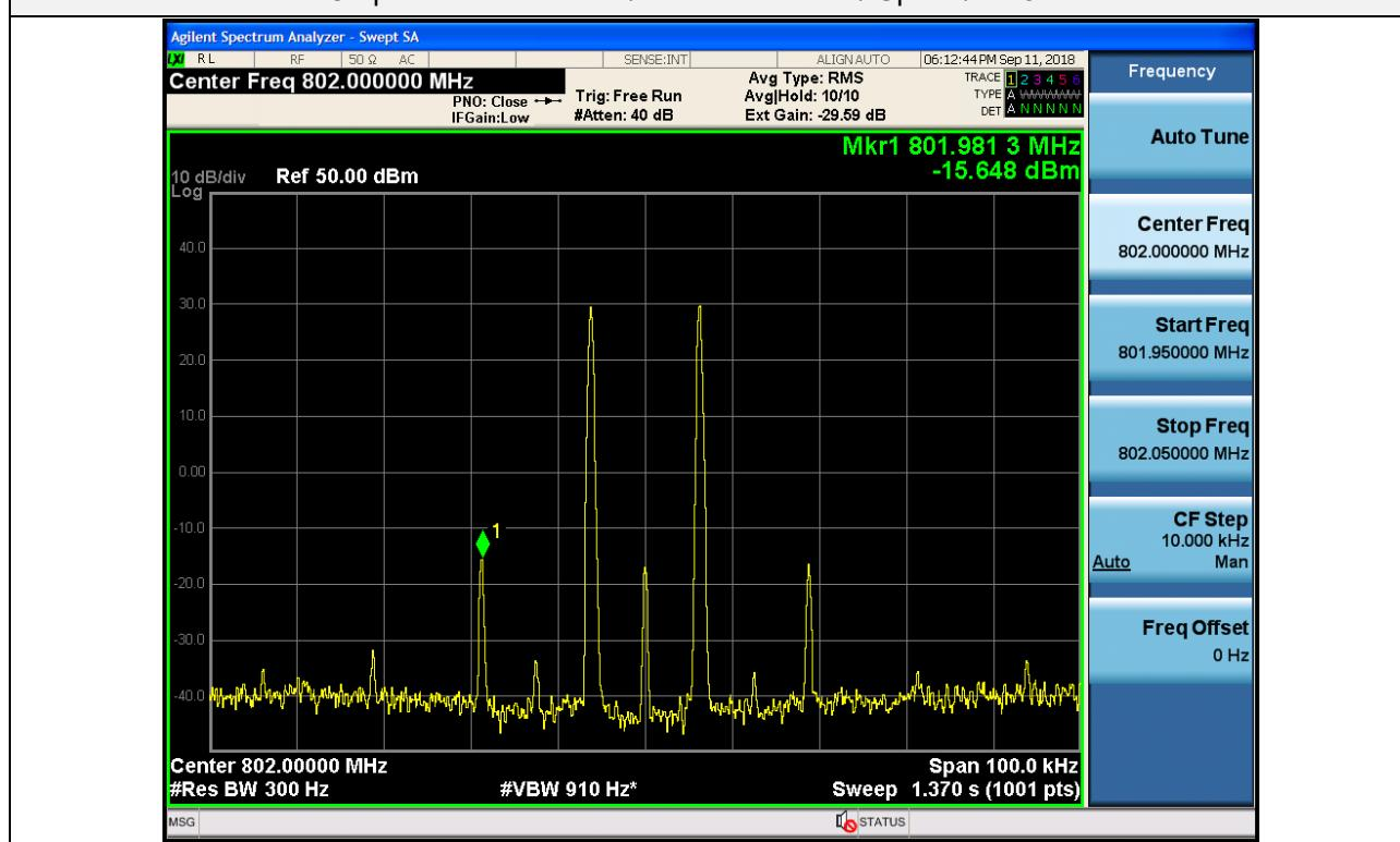
Output Intermodulation / PS Narrowband / Uplink / 6.25 kHz
