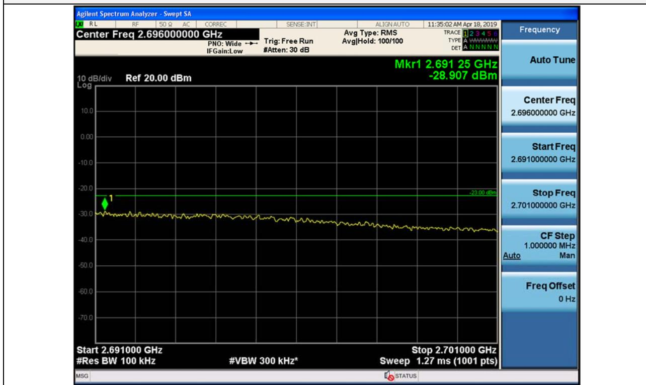
Spurious / 5G NR 60 MHz, 1 Carrier / Downlink / NR 60 MHz / High / High Edge + 11 MHz ~ 10 GHz
