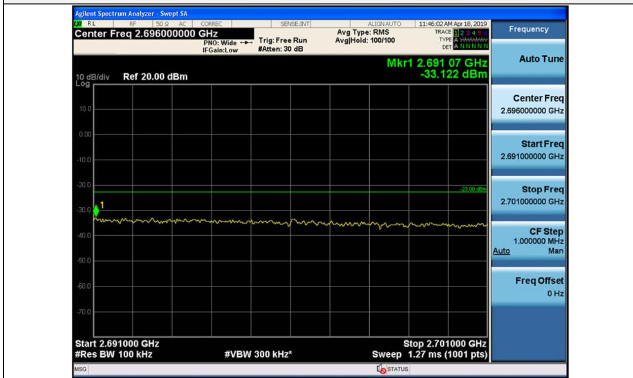
Spurious / 5G NR 60 MHz, 1 Carrier / Downlink / NR 60 MHz / Middle / High Edge + 11 MHz ~ 10 GHz
