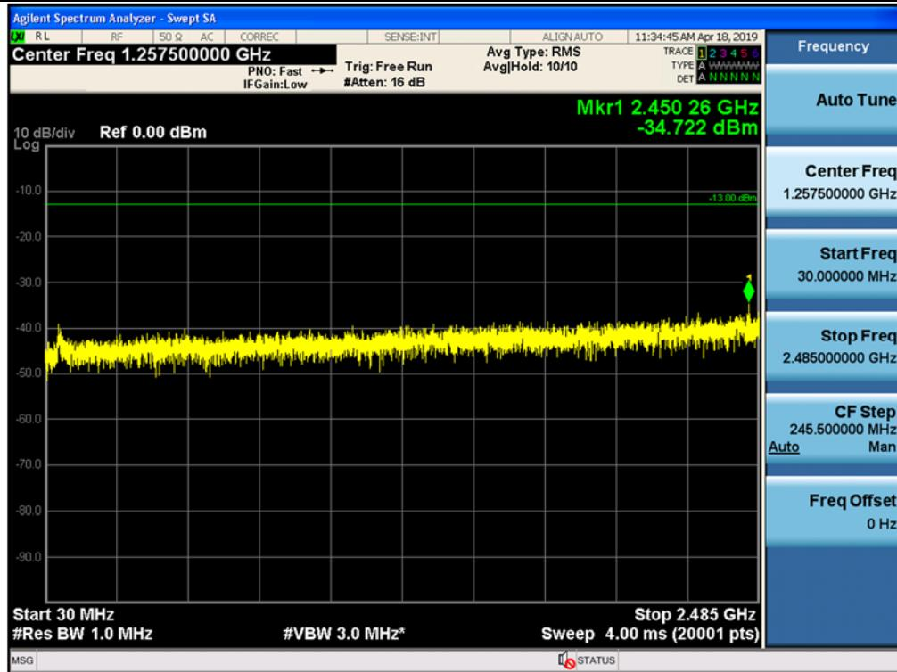
Spurious / 5G NR 60 MHz, 1 Carrier / Downlink / NR 60 MHz / High / Low Edge - 11 MHz ~ Low Edge - 1 MHz
