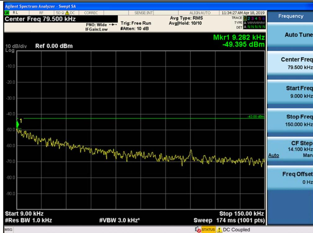
Spurious / 5G NR 60 MHz, 1 Carrier / Downlink / NR 60 MHz / High / 150 kHz ~ 30 MHz
