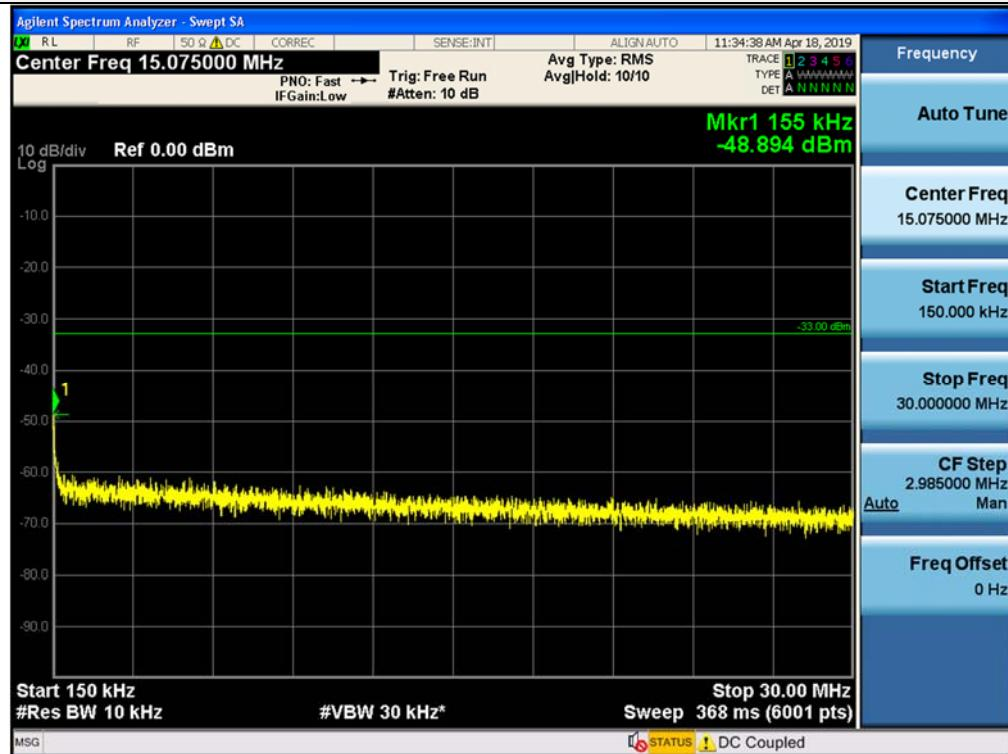
Spurious / 5G NR 60 MHz, 1 Carrier / Downlink / NR 60 MHz / High / 30 MHz ~ Low Edge - 11 MHz
