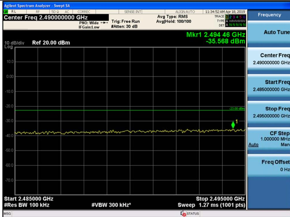
Spurious / 5G NR 60 MHz, 1 Carrier / Downlink / NR 60 MHz / High / High Edge + 1 MHz ~ High Edge + 11 MHz
