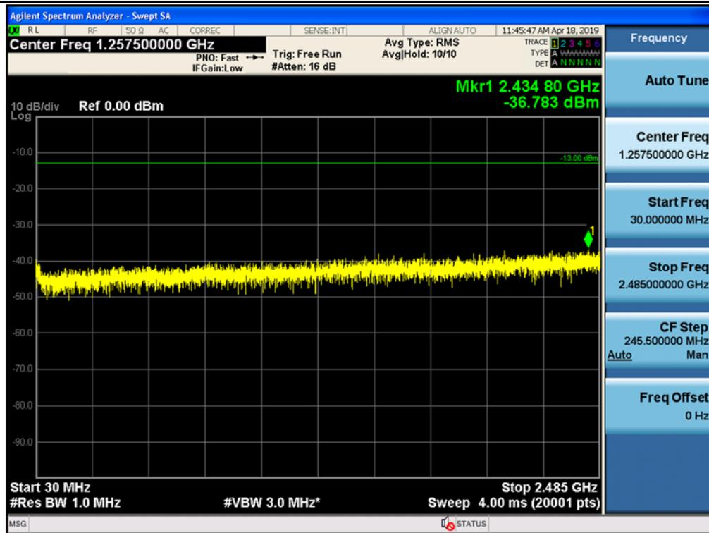
Spurious / 5G NR 60 MHz, 1 Carrier / Downlink / NR 60 MHz / Middle / Low Edge - 11 MHz ~ Low Edge - 1 MHz
