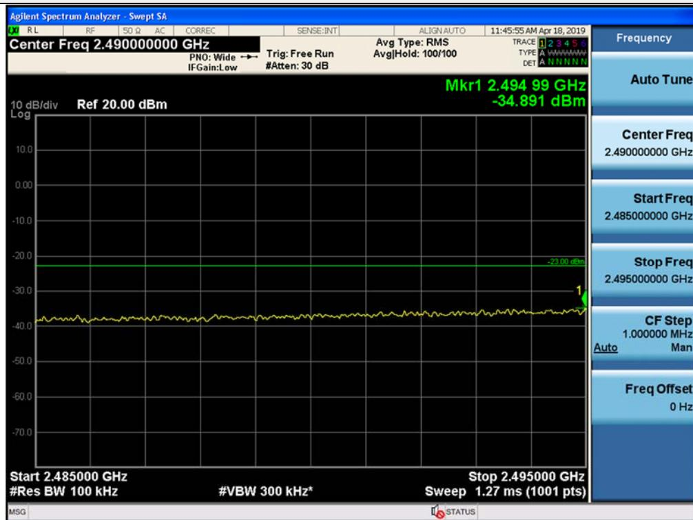
Spurious / 5G NR 60 MHz, 1 Carrier / Downlink / NR 60 MHz / Middle / High Edge + 1 MHz ~ High Edge + 11 MHz
