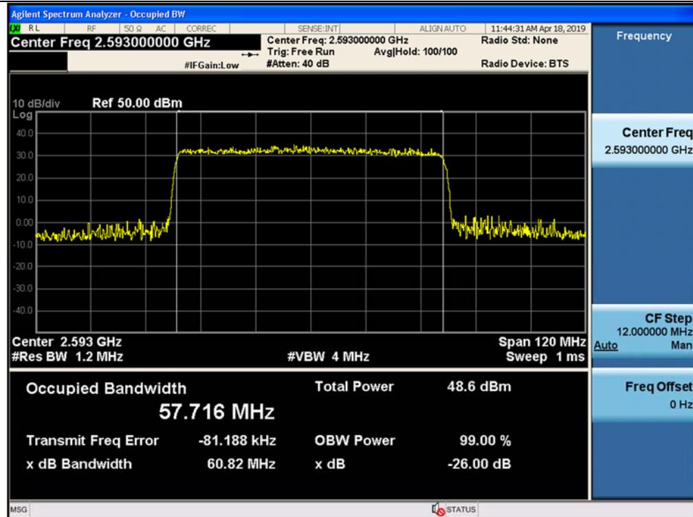
Input / BRS/EBS 4G LTE 20 MHz, 3 Carrier / Uplink / LTE 20 MHz (3C)
