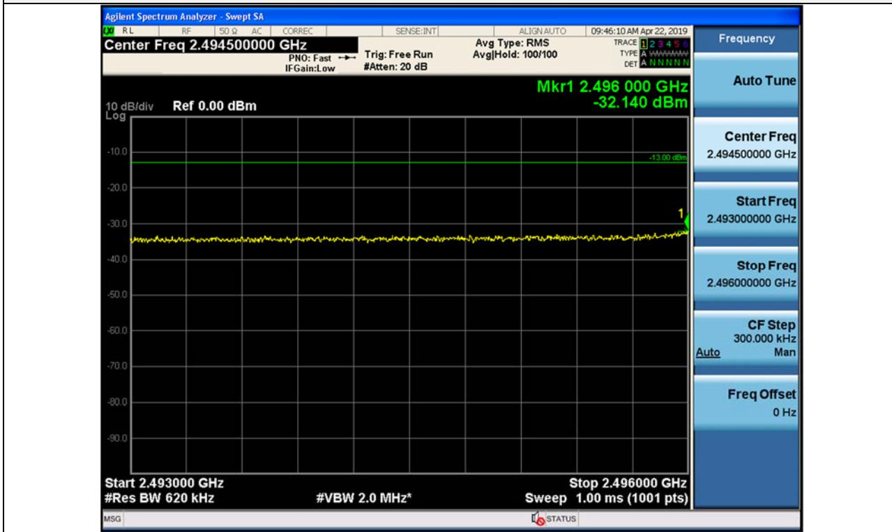
+3 dB above Out-of-band (two adjacent test signals) / 5G NR 60 MHz, 1 Carrier / Downlink / NR 60 MHz / Upper
