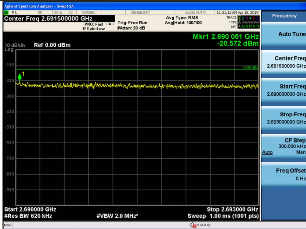
Out-of-band (single test signal) / 5G NR 60 MHz, 1 Carrier / Downlink / NR 60 MHz / Lower
