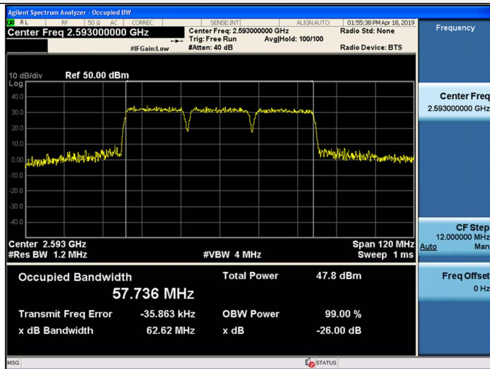
3 dB above the AGC threshold output / BRS/EBS 5G NR 60 MHz, 1 Carrier / Uplink / NR 60 MHz
