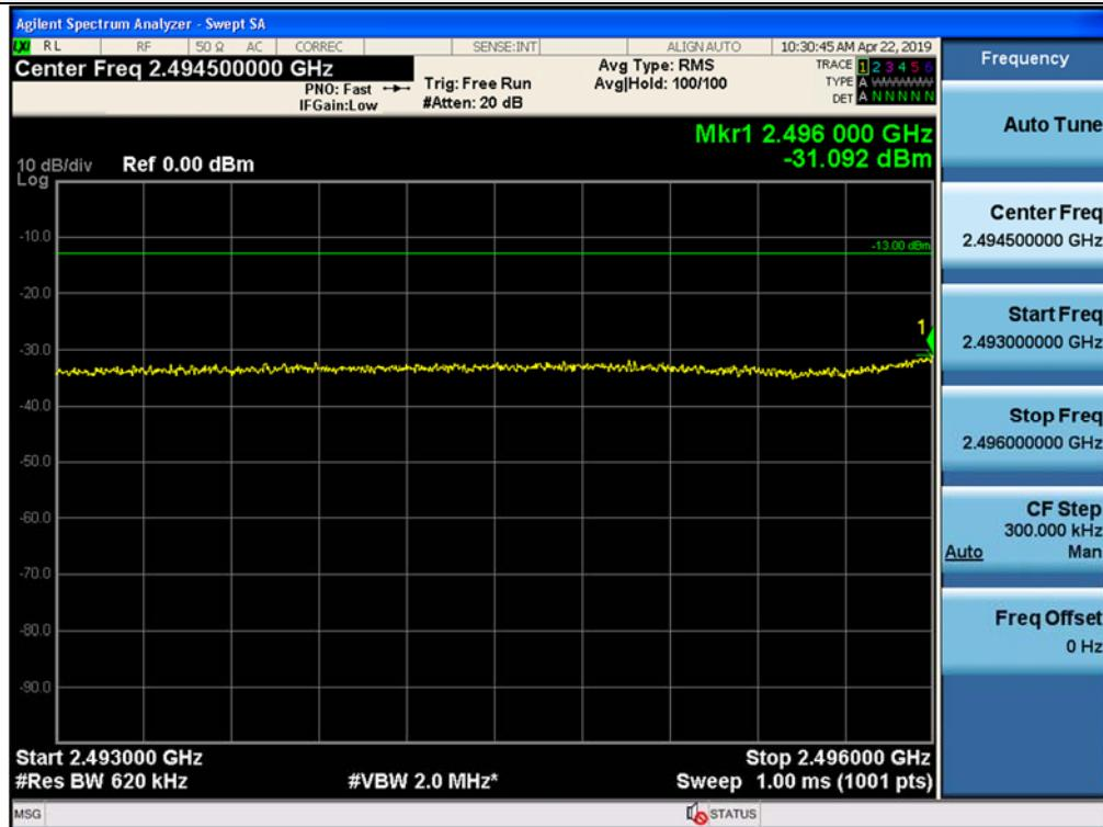
Out-of-band (single test signal) / 4G LTE 20 MHz, 3 Carrier / Downlink / LTE 20 MHz (3C) / Upper
