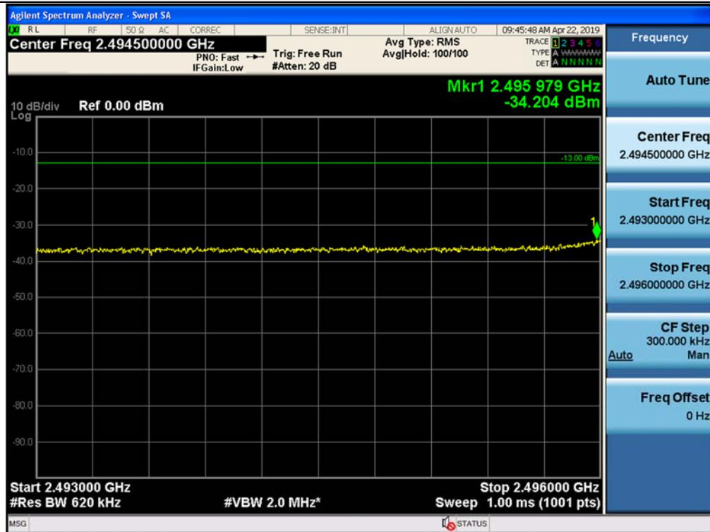
Out-of-band (two adjacent test signals) / 5G NR 60 MHz, 1 Carrier / Downlink / NR 60 MHz / Upper
