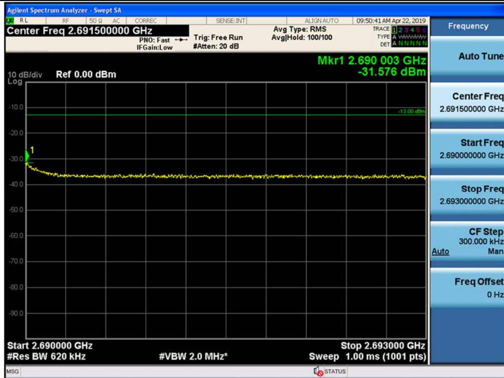
Out-of-band (two adjacent test signals) / BRS/EBS 5G NR 60 MHz, 1 Carrier / Uplink / NR 60 MHz / Lower
