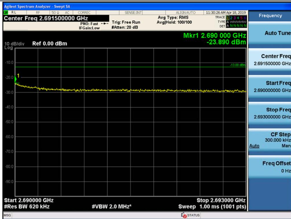
Out-of-band (two adjacent test signals) / 5G NR 60 MHz, 1 Carrier / Downlink / NR 60 MHz / Lower
