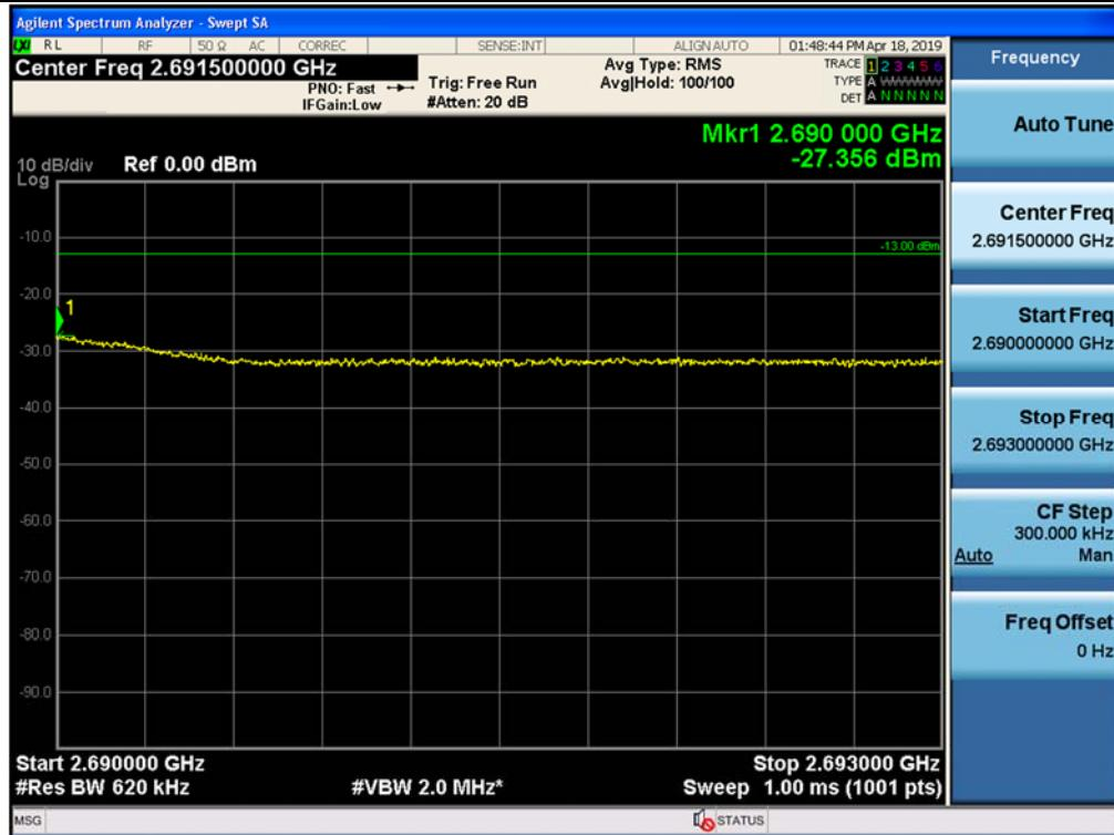
Out-of-band (single test signal) / 4G LTE 20 MHz, 3 Carrier / Downlink / LTE 20 MHz (3C) / Lower
