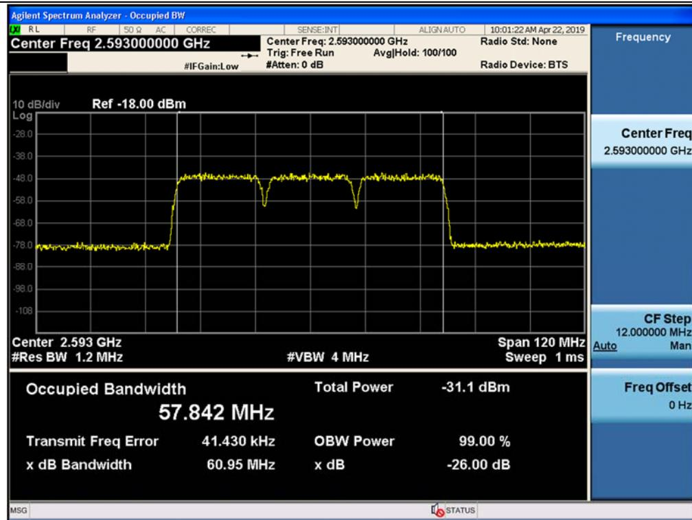
Input / BRS/EBS 4G LTE 20 MHz, 3 Carrier / Downlink / LTE 20 MHz (3C)
