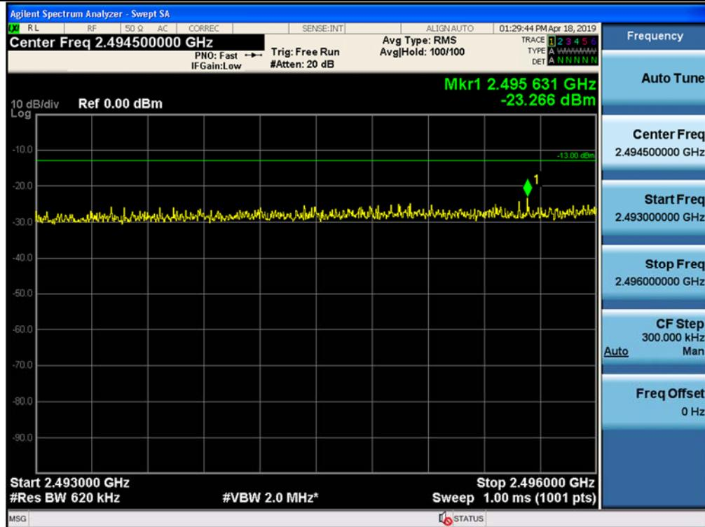
Out-of-band (single test signal) / 5G NR 60 MHz, 1 Carrier / Uplink / NR 60 MHz / Upper
