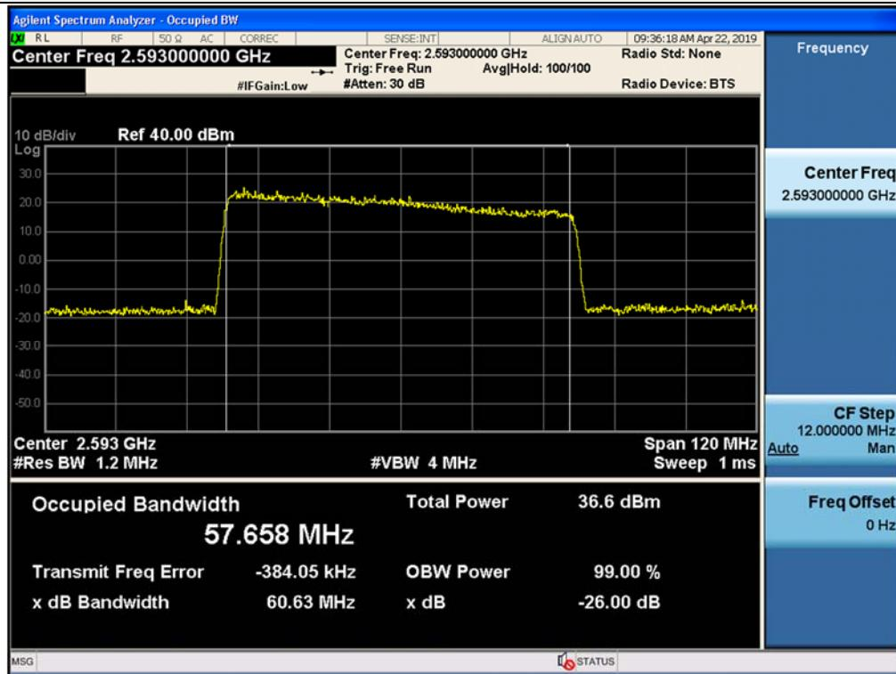
3 dB above the AGC threshold output / BRS/EBS 5G NR 60 MHz, 1 Carrier / Downlink / NR 60 MHz
