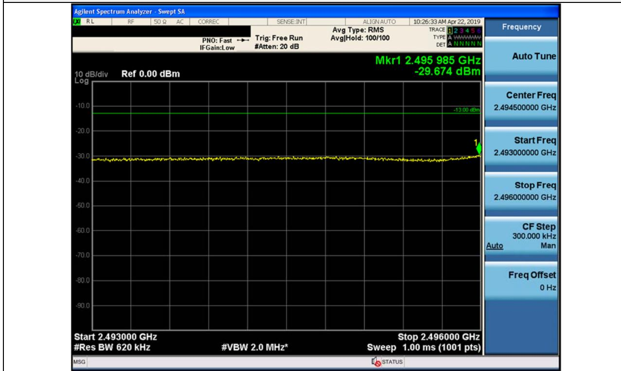
+3 dB above Out-of-band (two adjacent test signals) / 4G LTE 20 MHz, 3 Carrier / Downlink / LTE 20 MHz (3C) / Upper
