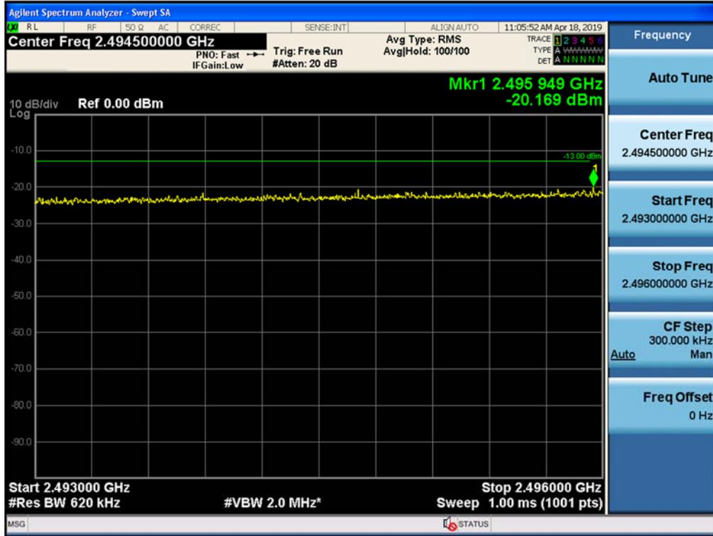
Out-of-band (single test signal) / 4G LTE 20 MHz, 3 Carrier / Uplink / LTE 20 MHz (3C) / Upper
