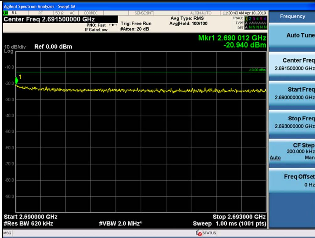
+3 dB above Out-of-band (two adjacent test signals) / 5G NR 60 MHz, 1 Carrier / Downlink / NR 60 MHz / Lower
