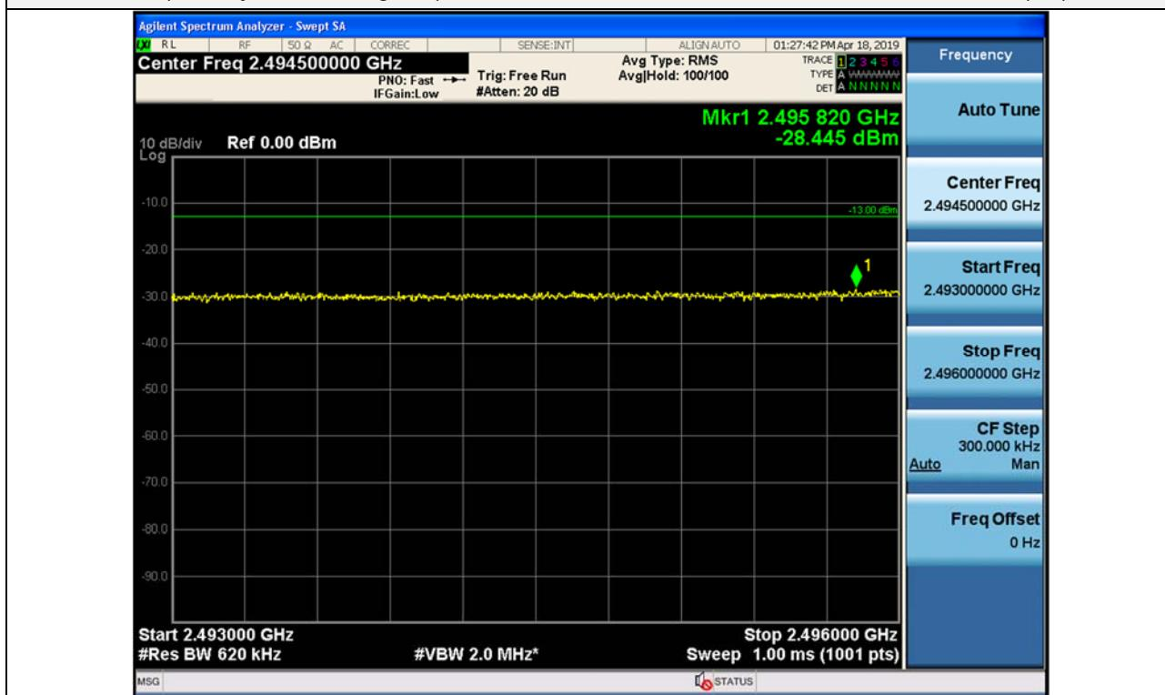
Out-of-band (two adjacent test signals) / 5G NR 60 MHz, 1 Carrier / Uplink / NR 60 MHz / Upper
