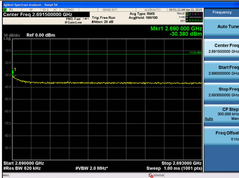
Out-of-band (single test signal) / 5G NR 60 MHz, 1 Carrier / Uplink / NR 60 MHz / Lower
