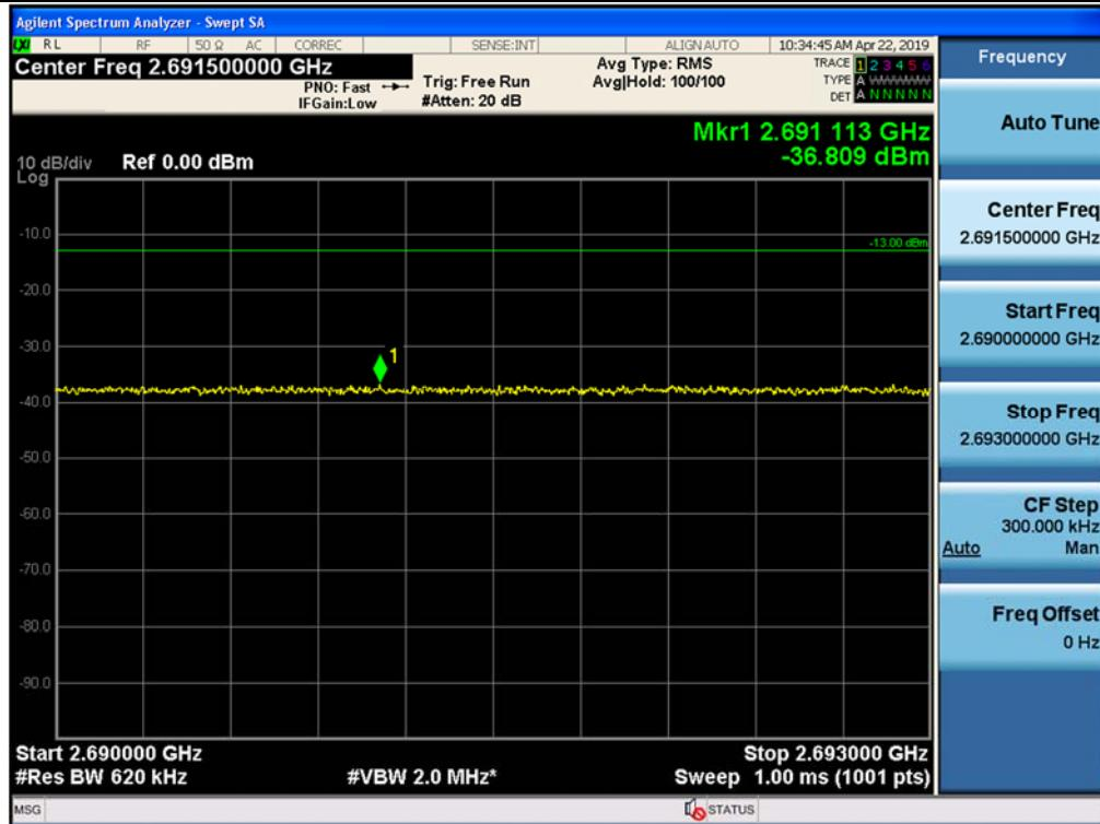
Out-of-band (single test signal) / 4G LTE 20 MHz, 3 Carrier / Uplink / LTE 20 MHz (3C) / Lower
