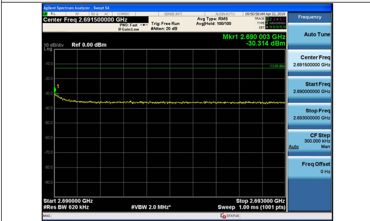
+3 dB above Out-of-band (two adjacent test signals) / BRS/EBS 5G NR 60 MHz, 1 Carrier / Uplink / NR 60 MHz / Lower
