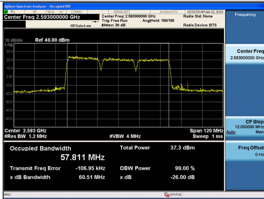
3 dB above the AGC threshold output / BRS/EBS 4G LTE 20 MHz, 3 Carrier / Downlink / LTE 20 MHz (3C)
