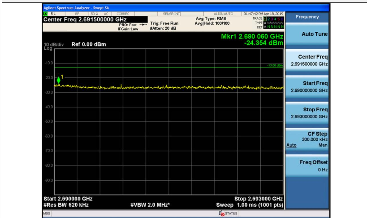
Out-of-band (two adjacent test signals) / 4G LTE 20 MHz, 3 Carrier / Downlink / LTE 20 MHz (3C) / Lower
