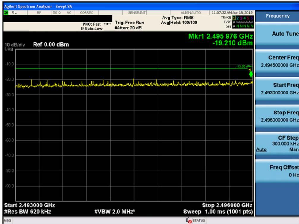
+3 dB above Out-of-band (single test signal) / 4G LTE 20 MHz, 3 Carrier / Uplink / LTE 20 MHz (3C) / Upper
