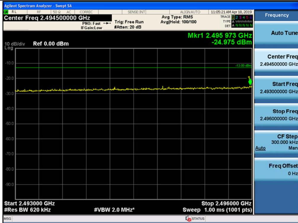
+3 dB above Out-of-band (two adjacent test signals) / 4G LTE 20 MHz, 3 Carrier / Uplink / LTE 20 MHz (3C) / Upper
