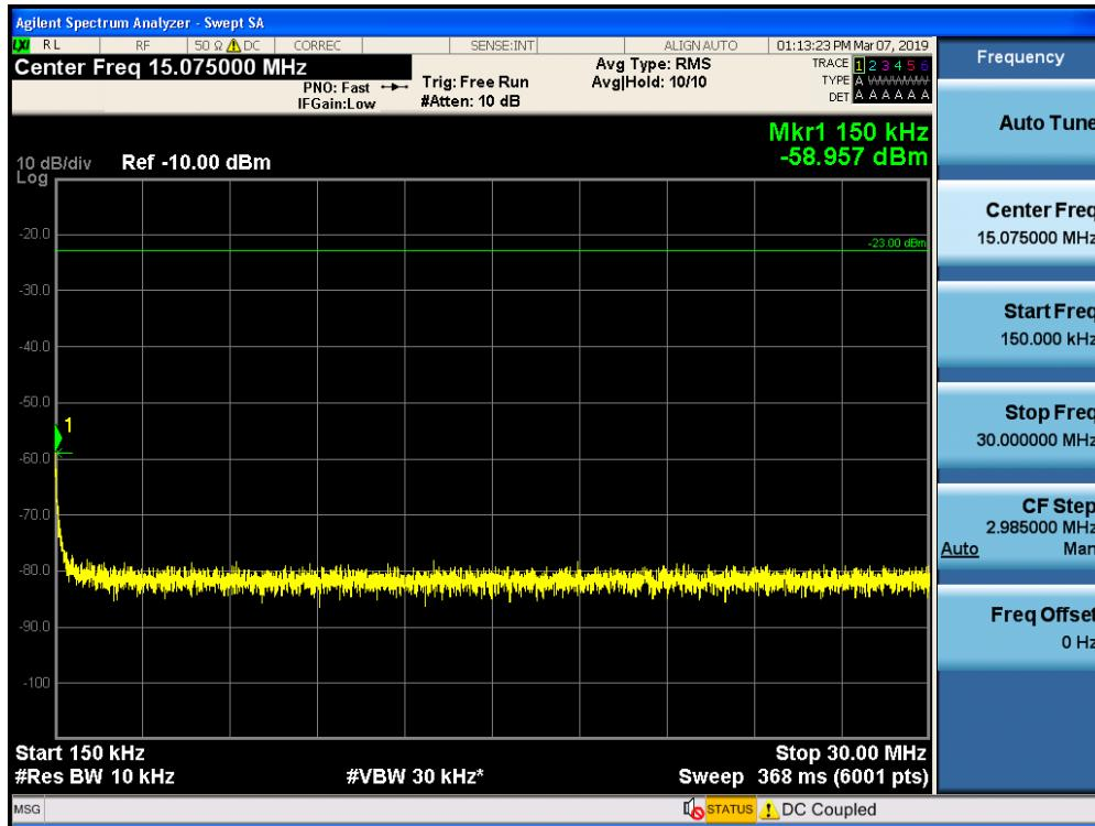
Conducted Spurious Emissions / Upper 700 MHz / Uplink / 30 MHz ~ 775.9 MHz
