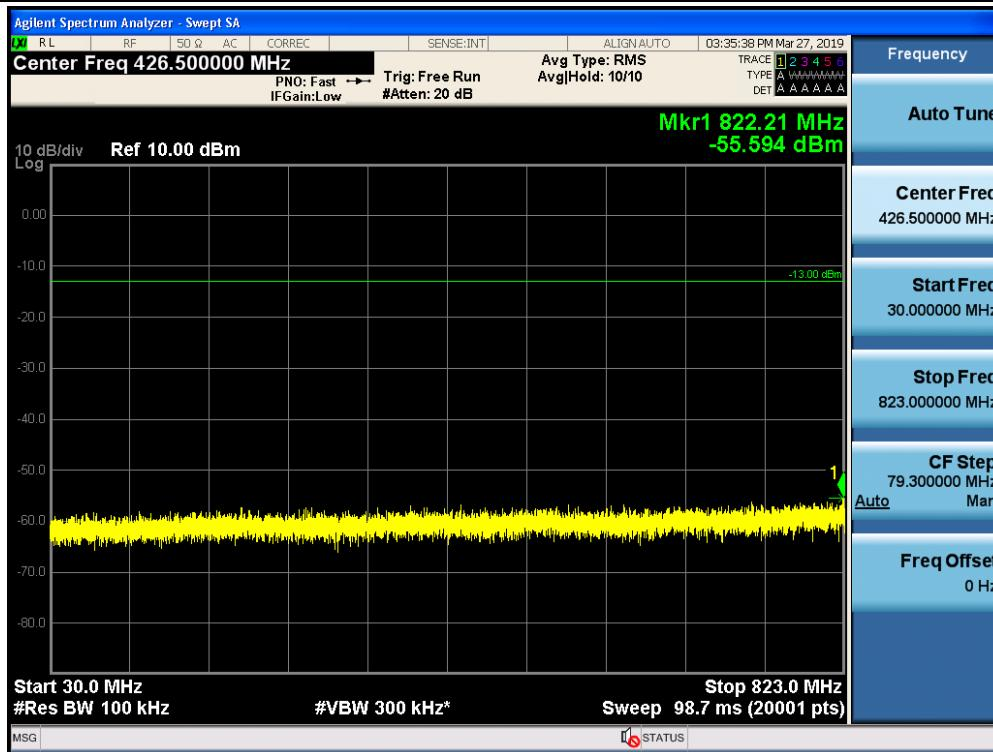
Conducted Spurious Emissions / Cellular / Uplink / 850 MHz ~ 1 GHz
