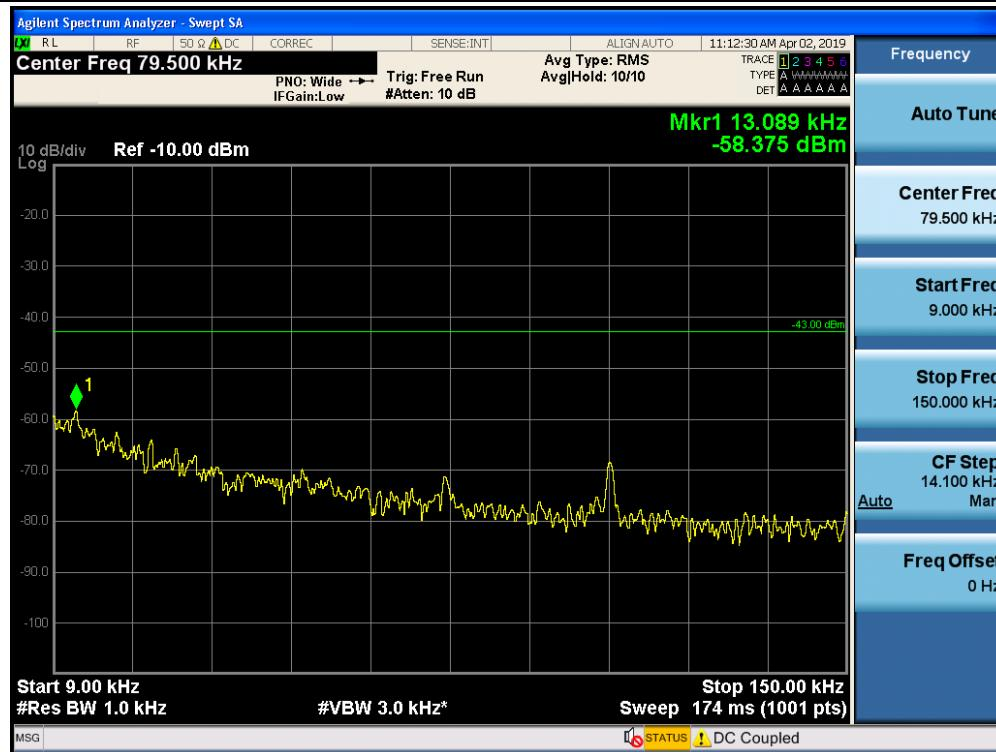
Conducted Spurious Emissions / AWS-1 / Downlink / 150 kHz ~ 30 MHz
