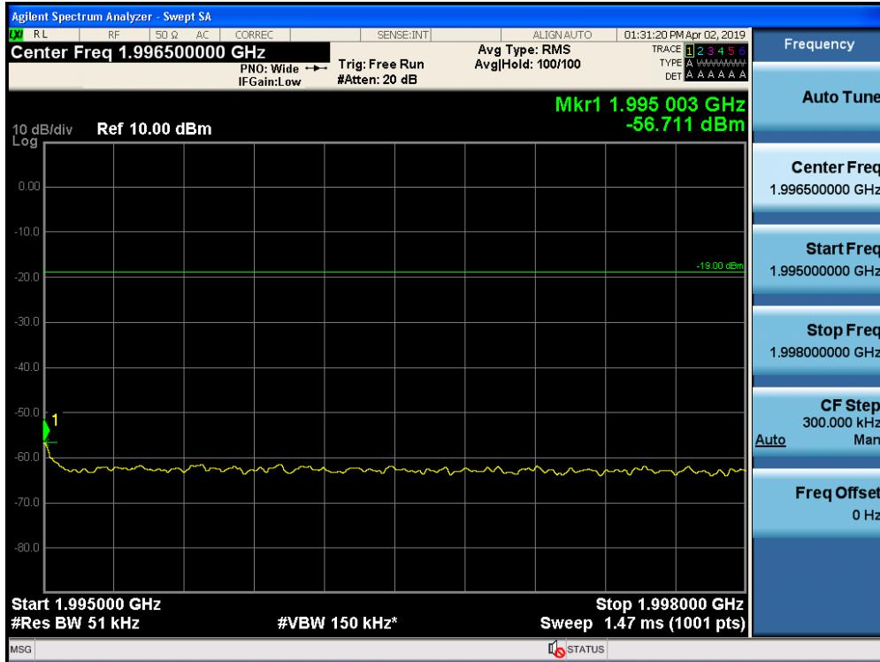
Out-of-Band Emissions / Broadband PCS / Downlink / LTE 5 MHz / Upper Edge / AGC threshold +10 dB
