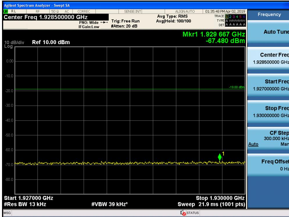
Out-of-Band Emissions / Broadband PCS / Downlink / CDMA / Lower Edge / AGC threshold +10 dB
