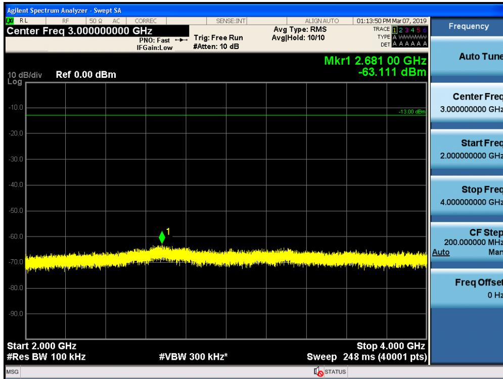
Conducted Spurious Emissions / Upper 700 MHz / Uplink / 4 GHz ~ 6 GHz
