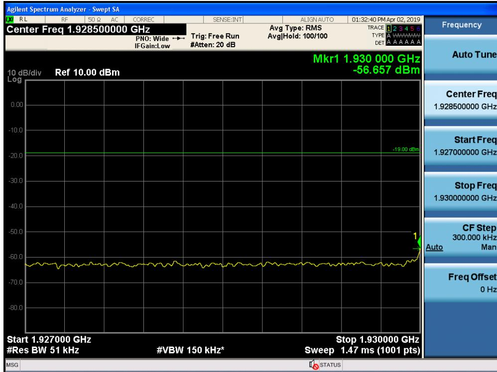
Out-of-Band Emissions / Broadband PCS / Downlink / LTE 5 MHz / Lower Edge / AGC threshold +10 dB
