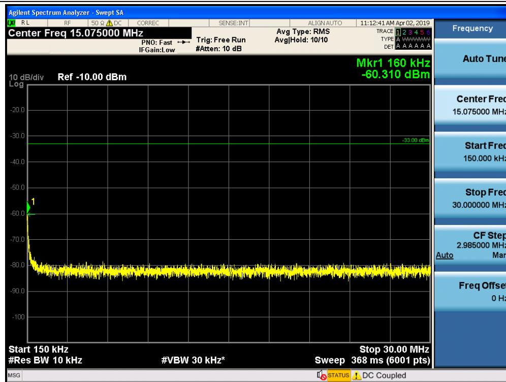
Conducted Spurious Emissions / AWS-1 / Downlink / 30 MHz ~ 2.109 GHz
