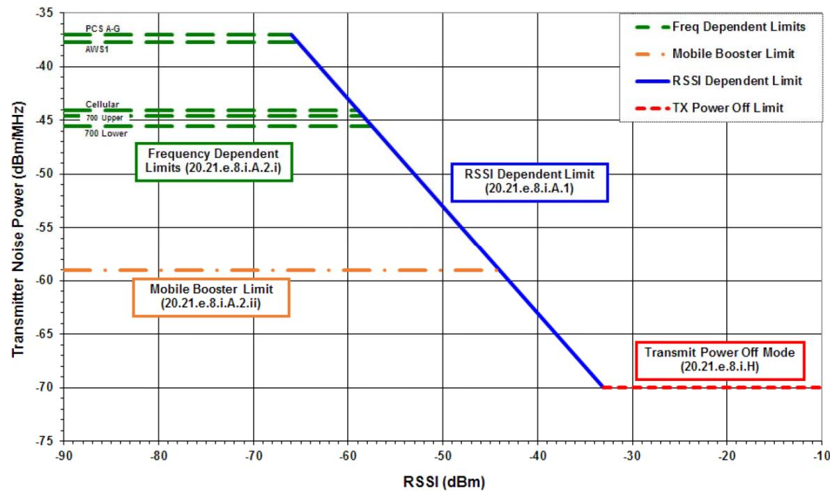
**Test Result:****Tabulated Result of Uplink Maximum Transmitter Noise Power Level**
