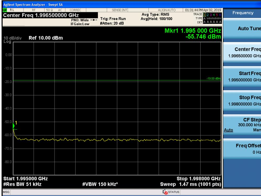
Out-of-Band Emissions / Broadband PCS / Downlink / LTE 5 MHz / Lower Edge / AGC threshold
