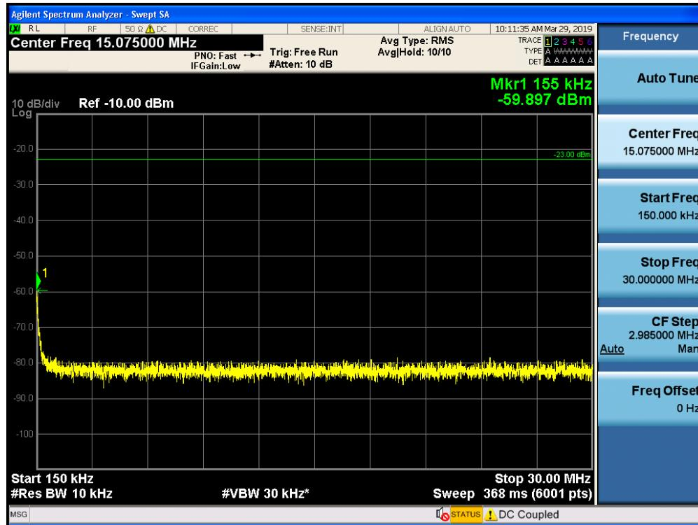
Conducted Spurious Emissions / Lower 700 MHz / Downlink / 30 MHz ~ 733.9 MHz
