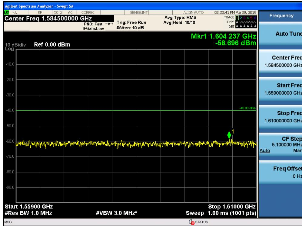
Conducted Spurious Emissions / Upper 700 MHz / Downlink / 1.559 GHz ~ 1.573 GHz (700 Hz)
