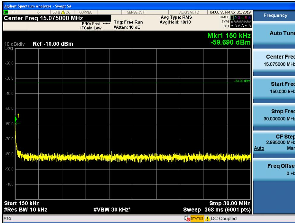
Conducted Spurious Emissions / AWS-1 / Uplink / 30 MHz ~ 1.709 GHz
