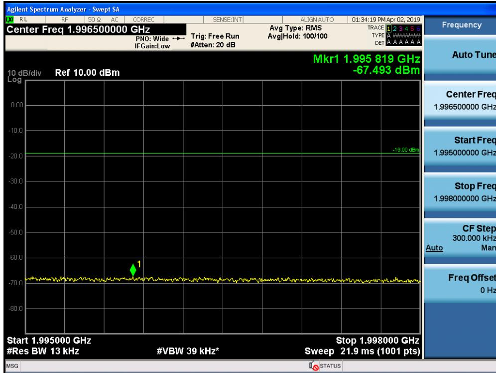
Out-of-Band Emissions / Broadband PCS / Downlink / CDMA / Upper Edge / AGC threshold +10 dB
