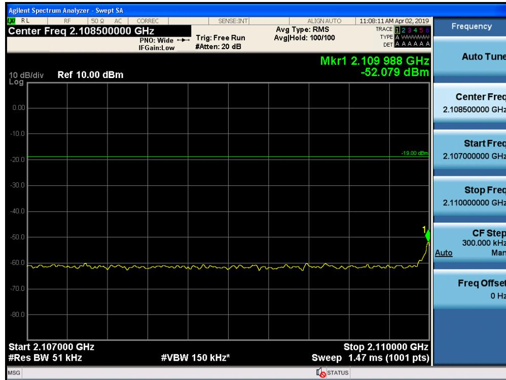
Out-of-Band Emissions / AWS-1 / Downlink / LTE 5 MHz / Lower Edge / AGC threshold +10 dB
