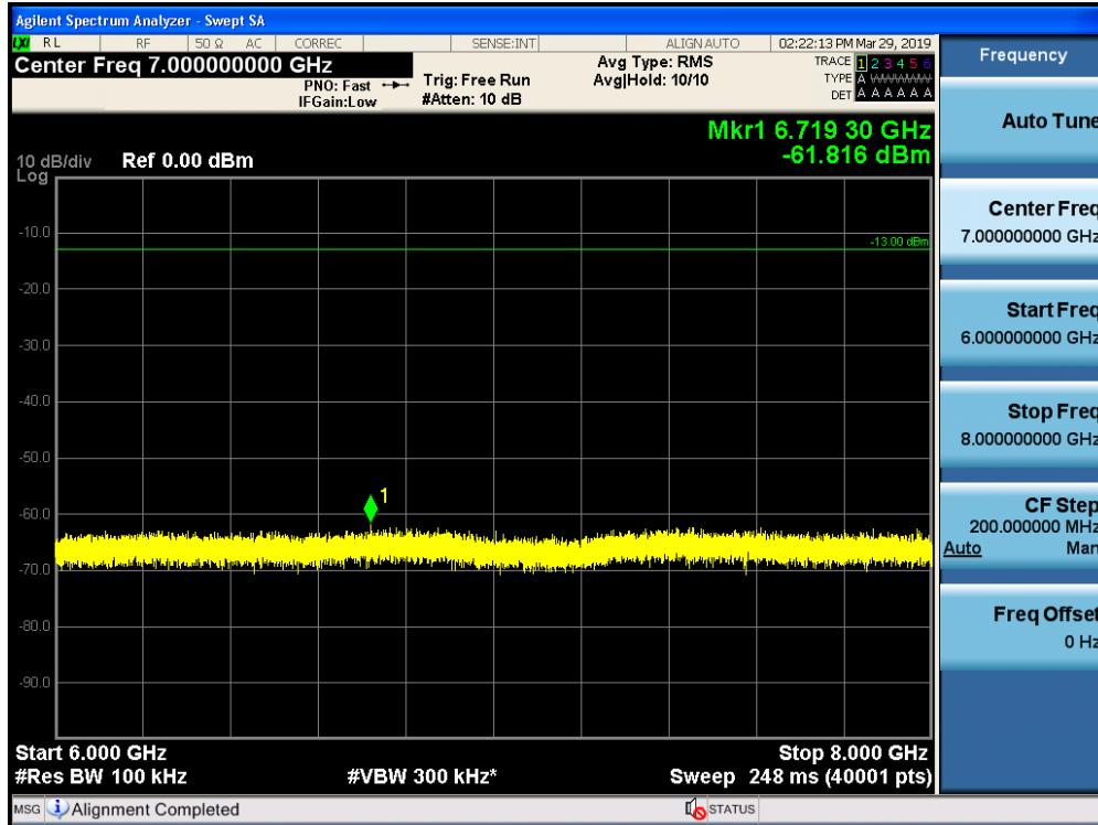
Conducted Spurious Emissions / Upper 700 MHz / Downlink / 763 MHz ~ 775 MHz
