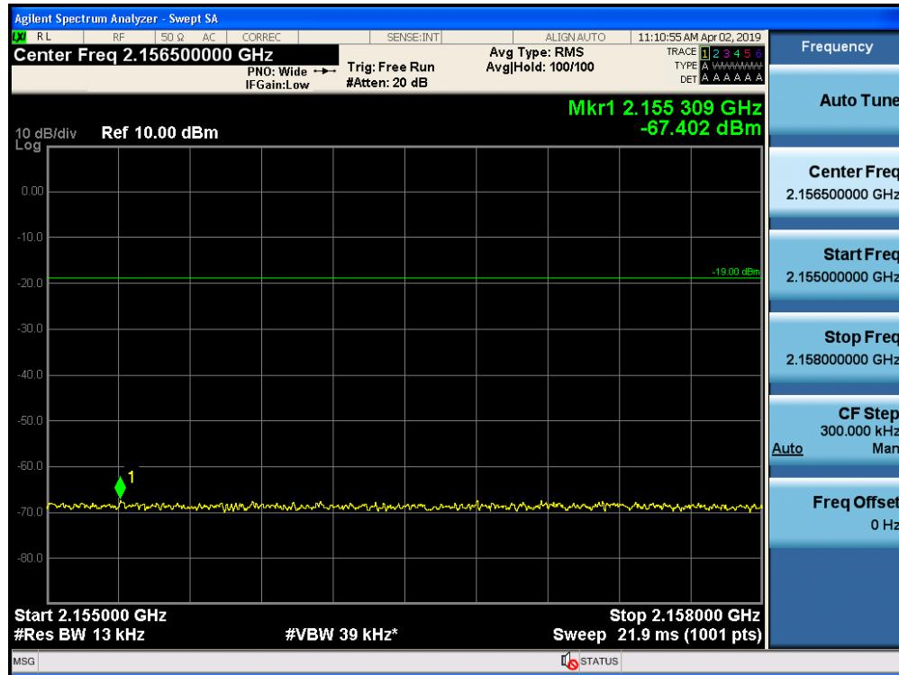
Out-of-Band Emissions / AWS-1 / Downlink / CDMA / Lower Edge / AGC threshold
