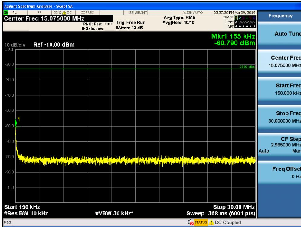
Conducted Spurious Emissions / Cellular / Downlink / 30 MHz ~ 868 MHz
