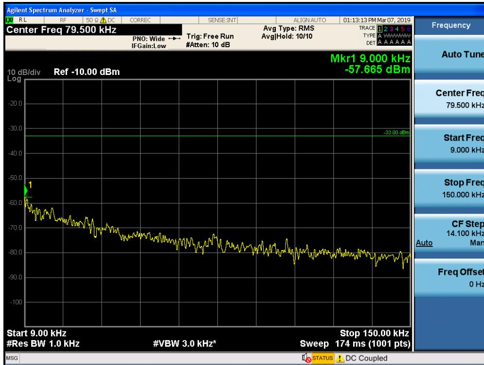
Conducted Spurious Emissions / Upper 700 MHz / Uplink / 150 kHz ~ 30 MHz
