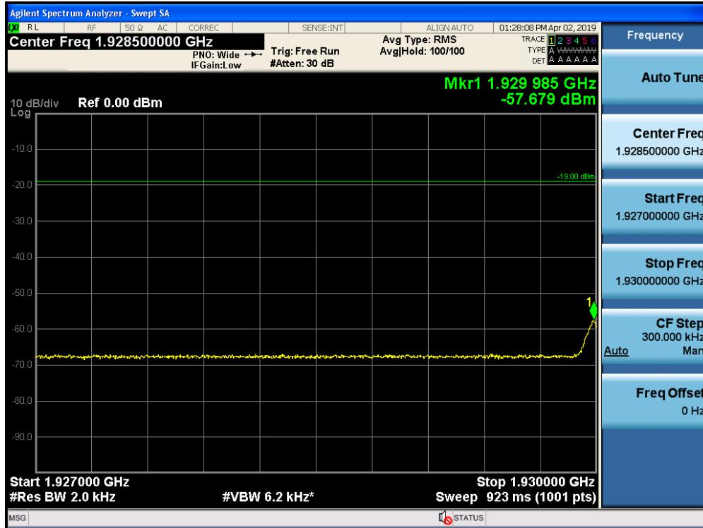
Out-of-Band Emissions / Broadband PCS / Downlink / GSM / Lower Edge / AGC threshold +10 dB
