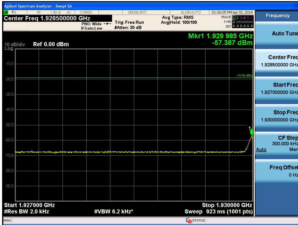
Out-of-Band Emissions / Broadband PCS / Downlink / LTE 5 MHz / Upper Edge / AGC threshold
