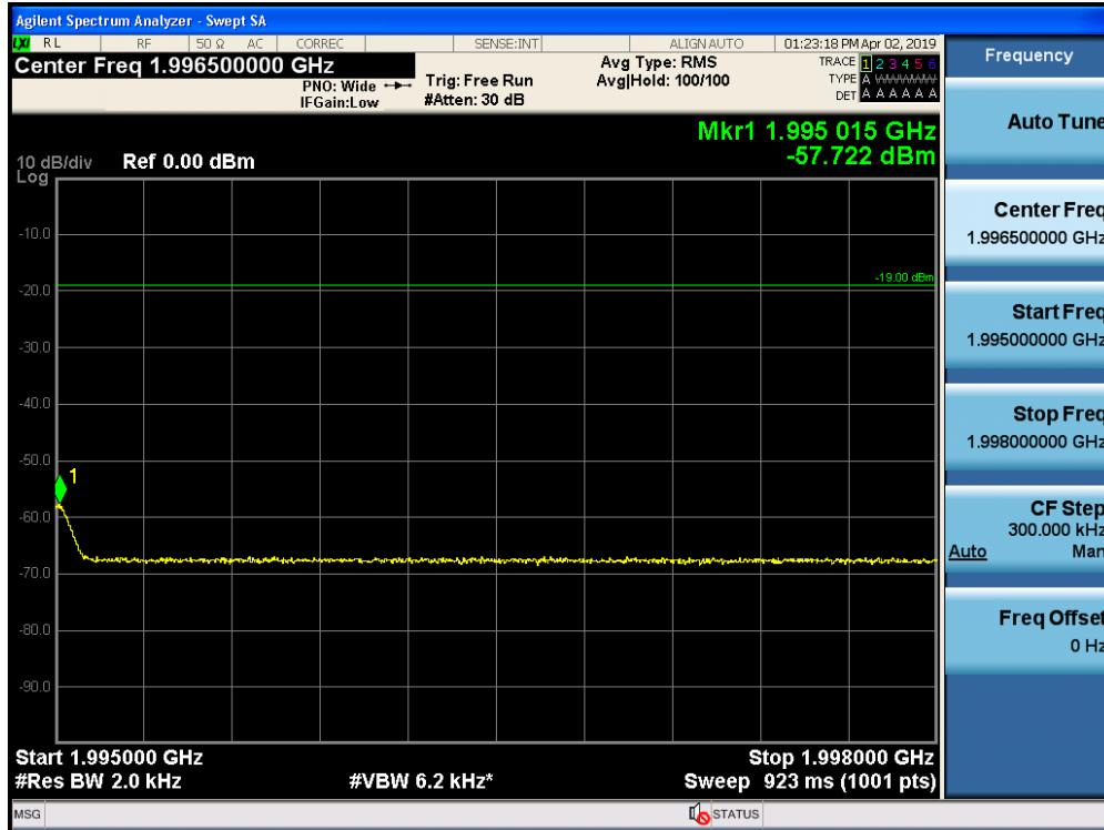
Out-of-Band Emissions / Broadband PCS / Downlink / GSM / Upper Edge / AGC threshold +10 dB
