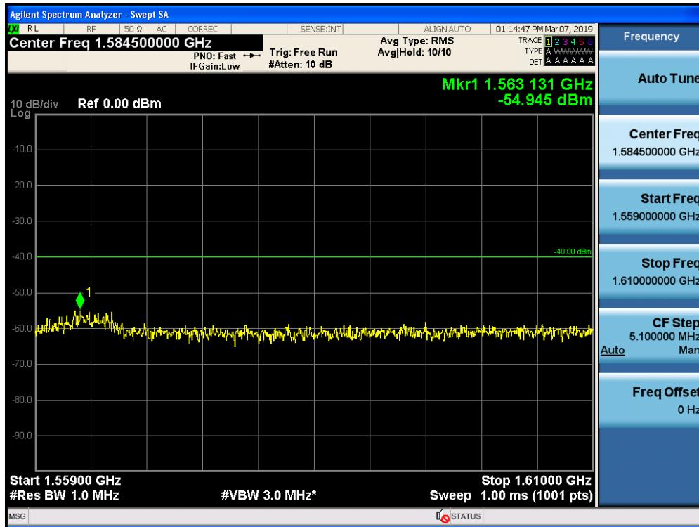
Conducted Spurious Emissions / Upper 700 MHz / Uplink / 1.559 GHz ~ 1.573 GHz (700 Hz)
