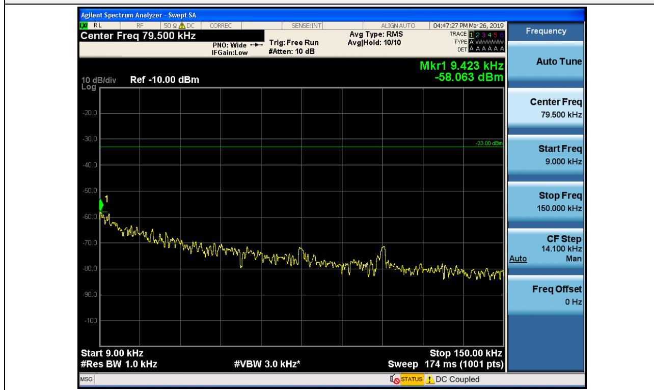
Conducted Spurious Emissions / Lower 700 MHz / Uplink / 150 kHz ~ 30 MHz
