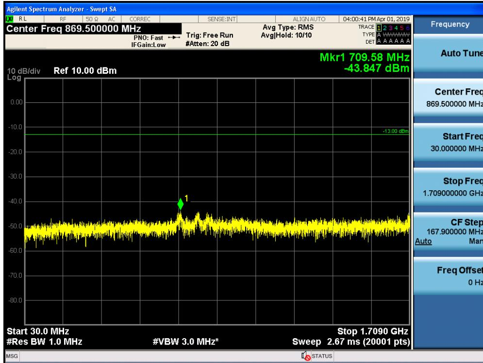
Conducted Spurious Emissions / AWS-1 / Uplink / 1.756 GHz ~ 10 GHz
