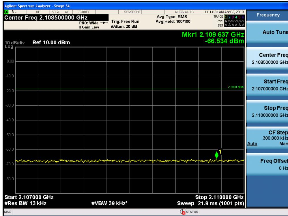
Out-of-Band Emissions / AWS-1 / Downlink / CDMA / Lower Edge / AGC threshold +10 dB
