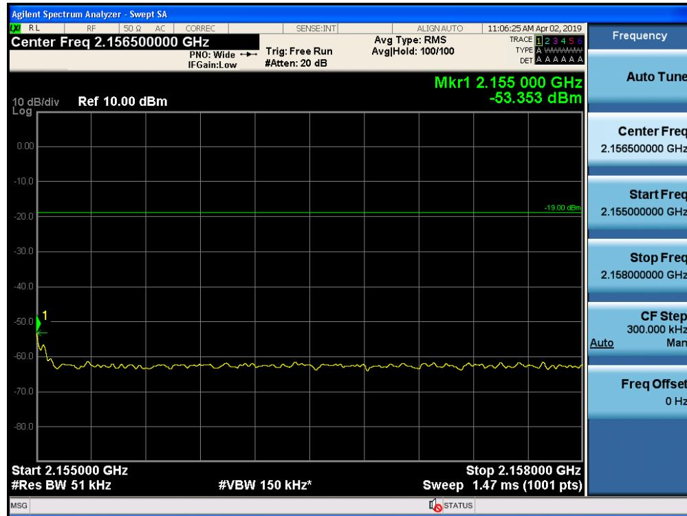
Out-of-Band Emissions / AWS-1 / Downlink / LTE 5 MHz / Lower Edge / AGC threshold
