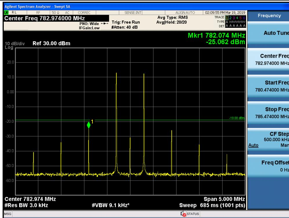
Intermodulation / Upper 700 MHz / Uplink / AGC threshold +10 dB
