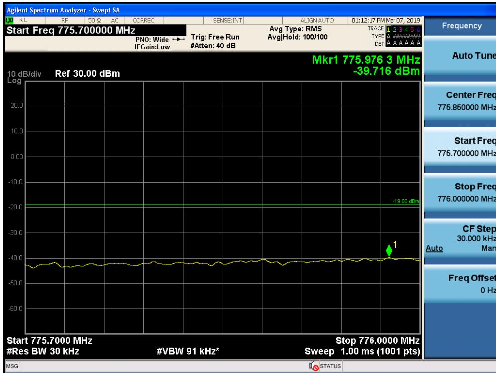
Out-of-Band Emissions / Upper 700 MHz / Uplink / CDMA / Lower Edge / AGC threshold +10 dB
