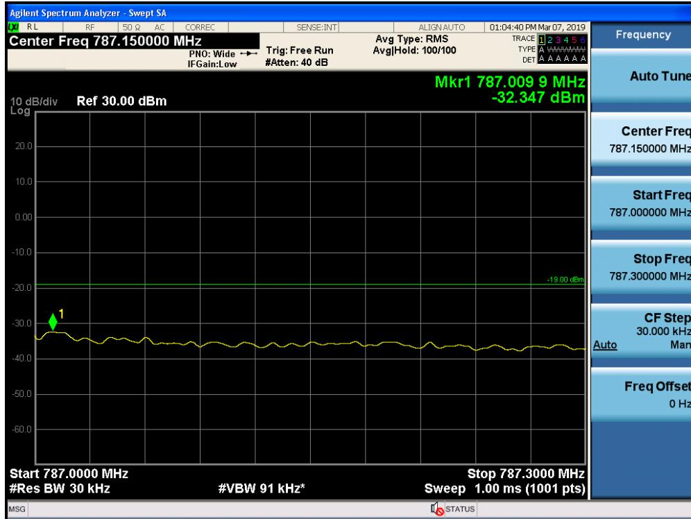
Out-of-Band Emissions / Upper 700 MHz / Uplink / LTE 5 MHz / Upper Edge / AGC threshold +10 dB
