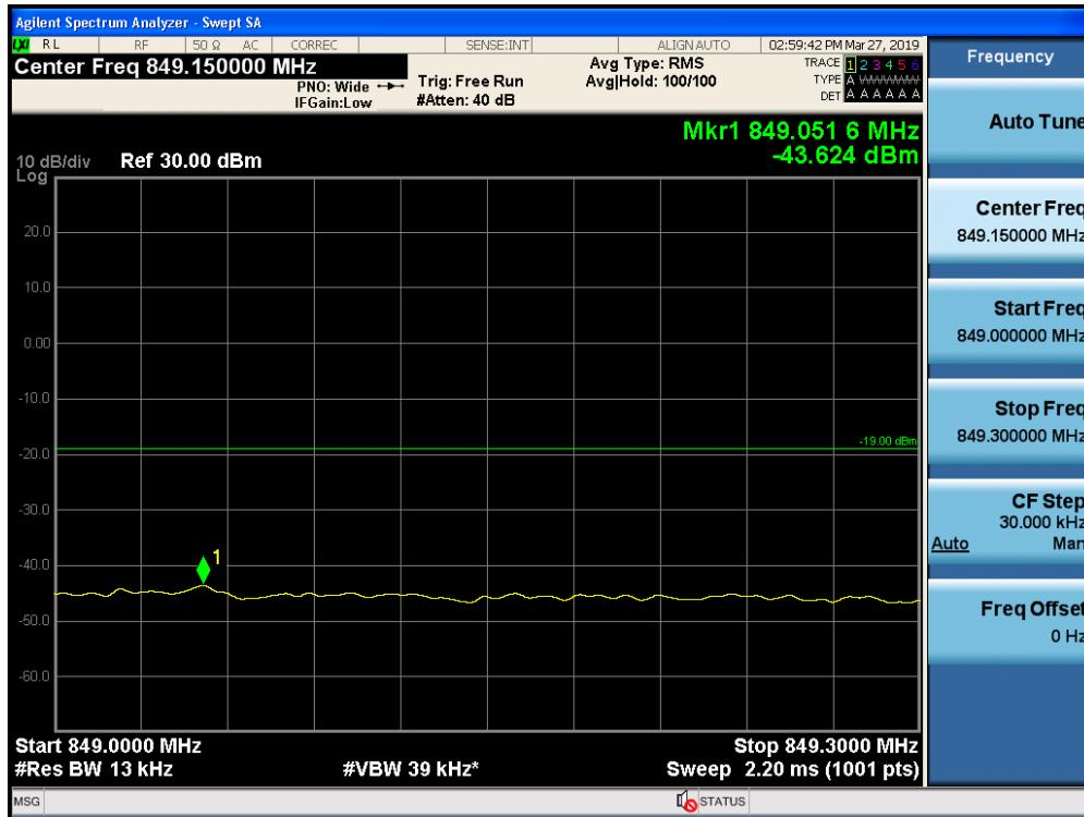
Out-of-Band Emissions / Cellular / Uplink / CDMA / Upper Edge / AGC threshold +10 dB
