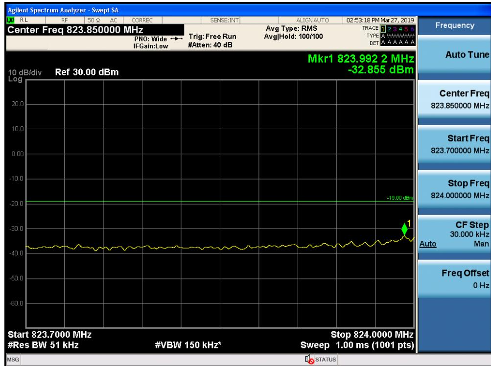
Out-of-Band Emissions / Cellular / Uplink / CDMA / Upper Edge / AGC threshold
