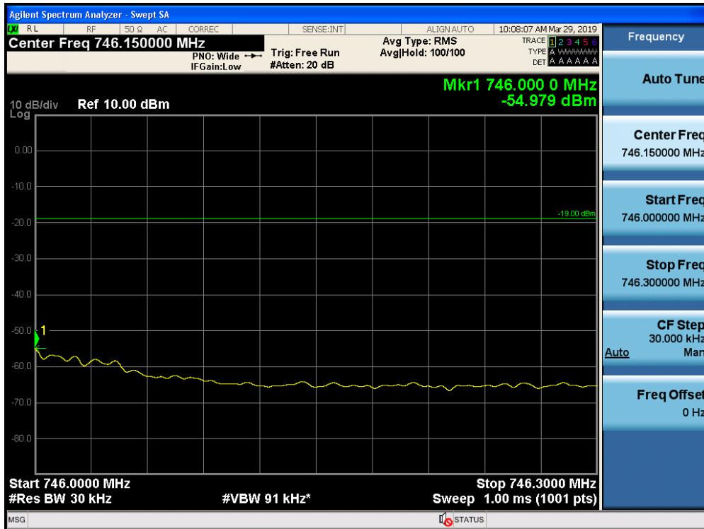
Out-of-Band Emissions / Lower 700 MHz / Downlink / LTE 5 MHz / Lower Edge / AGC threshold
