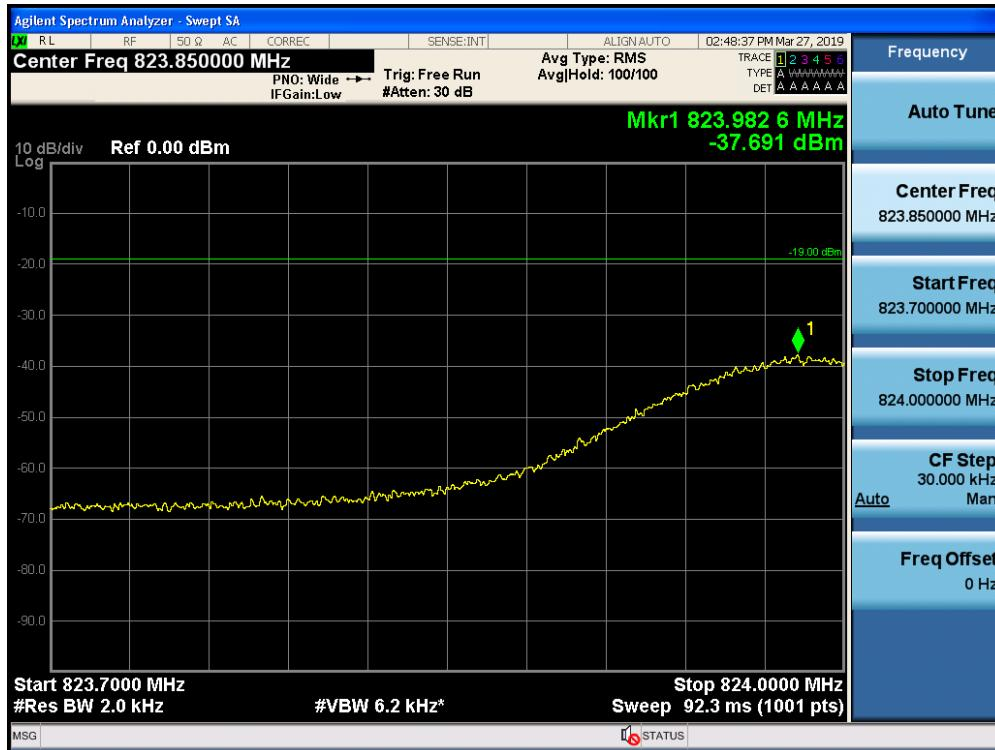
Out-of-Band Emissions / Cellular / Uplink / GSM / Lower Edge / AGC threshold +10 dB
