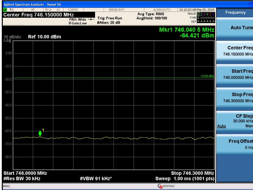
Out-of-Band Emissions / Lower 700 MHz / Downlink / CDMA / Lower Edge / AGC threshold
