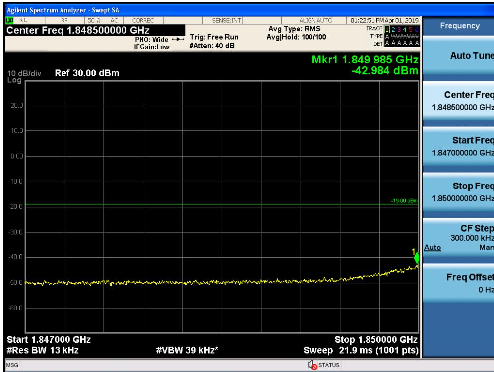
Out-of-Band Emissions / Broadband PCS / Uplink / CDMA / Lower Edge / AGC threshold +10 dB
