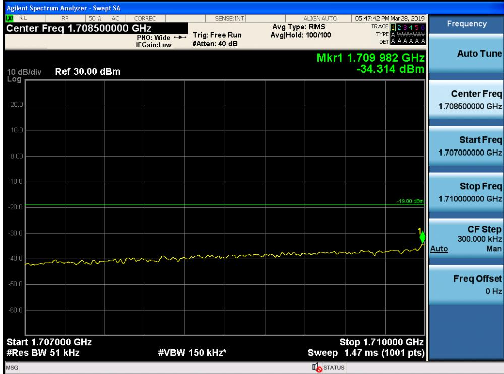
Out-of-Band Emissions / AWS-1 / Uplink / LTE 5 MHz / Lower Edge / AGC threshold +10 dB
