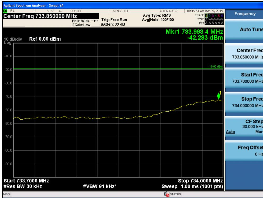
Out-of-Band Emissions / Lower 700 MHz / Downlink / GSM / Lower Edge / AGC threshold +10 dB
