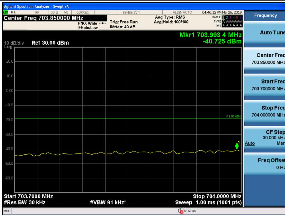
Out-of-Band Emissions / Lower 700 MHz / Uplink / CDMA / Lower Edge / AGC threshold +10 dB
