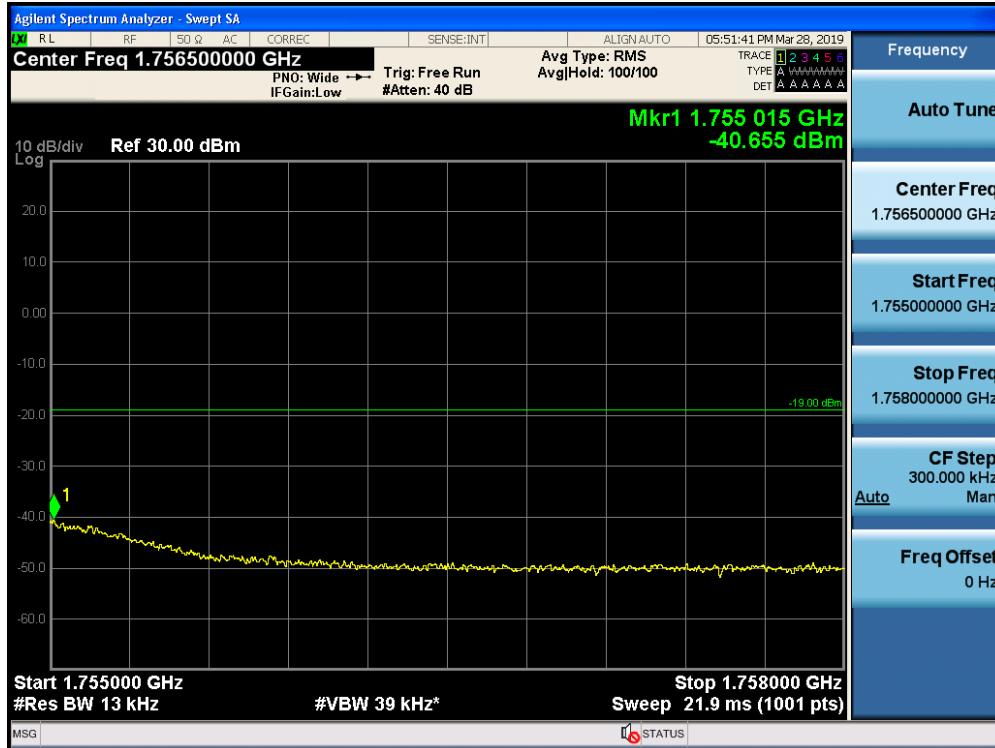
Out-of-Band Emissions / AWS-1 / Uplink / CDMA / Upper Edge / AGC threshold +10 dB
