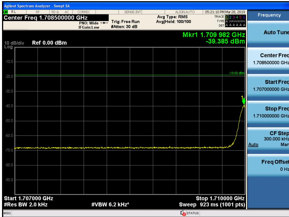
Out-of-Band Emissions / AWS-1 / Uplink / LTE 5 MHz / Upper Edge / AGC threshold
