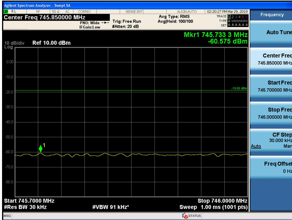
Out-of-Band Emissions / Upper 700 MHz / Downlink / CDMA / Lower Edge / AGC threshold +10 dB
