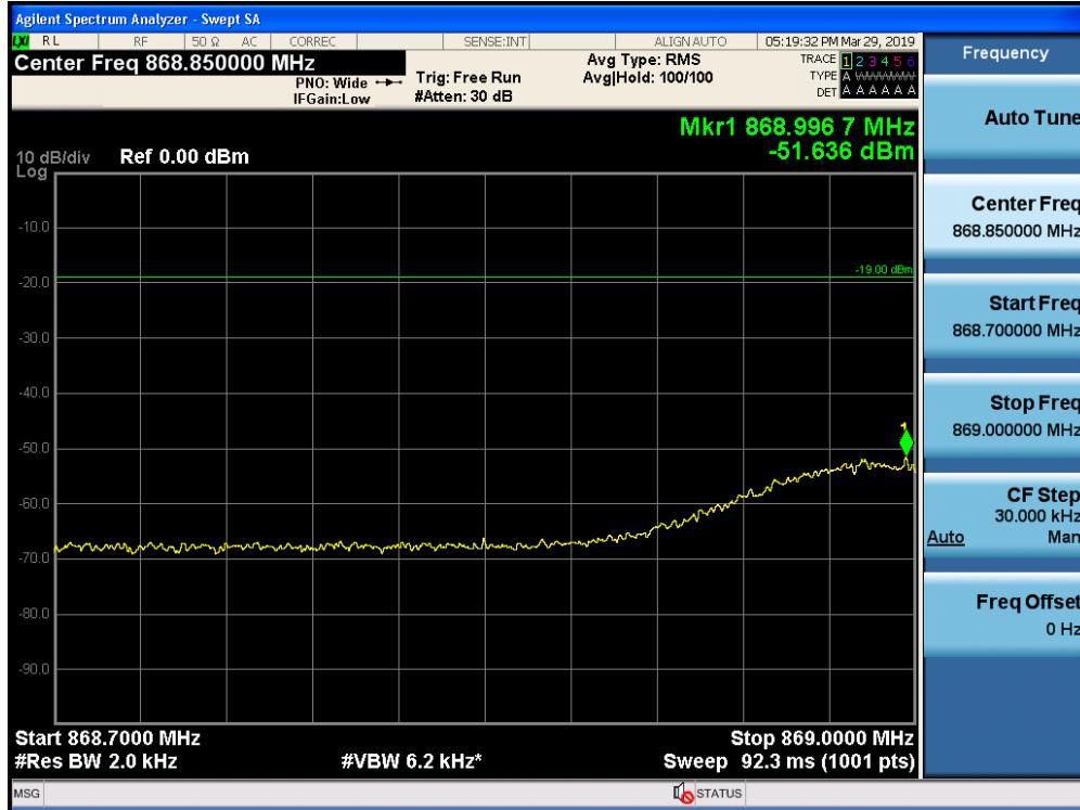
Out-of-Band Emissions / Cellular / Downlink / LTE 5 MHz / Upper Edge / AGC threshold
