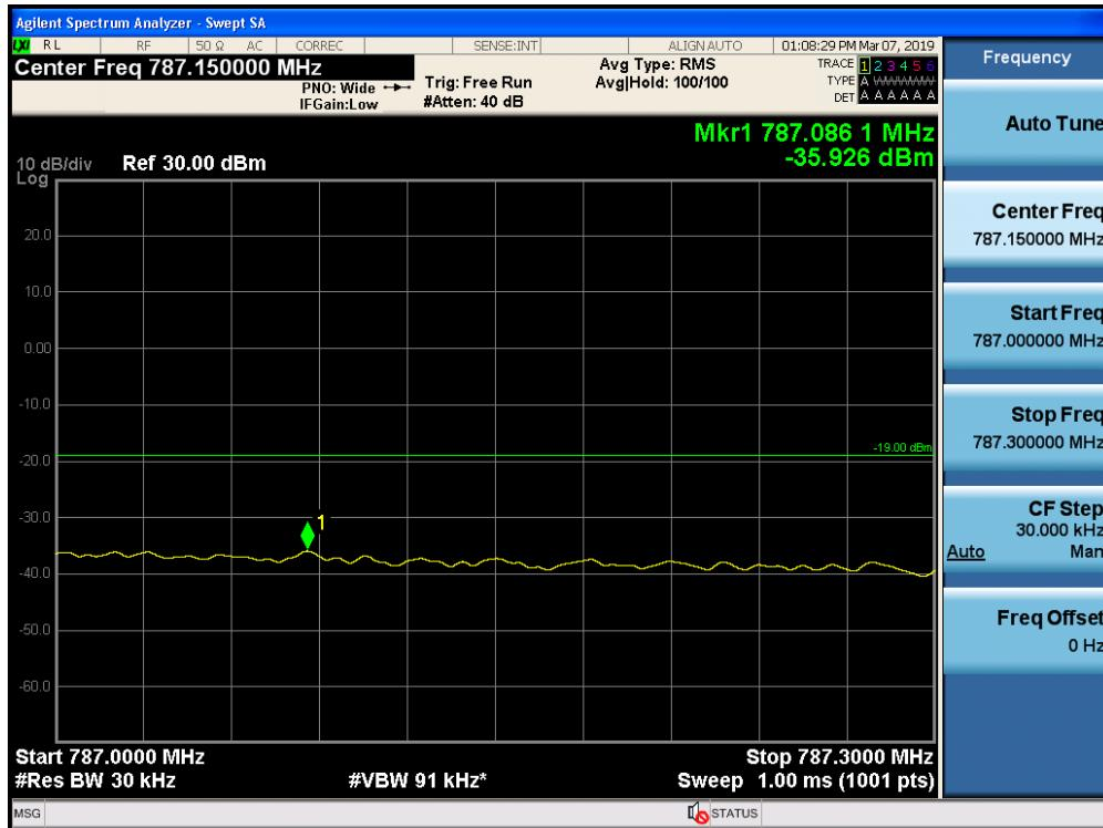
Out-of-Band Emissions / Upper 700 MHz / Uplink / CDMA / Lower Edge / AGC threshold
