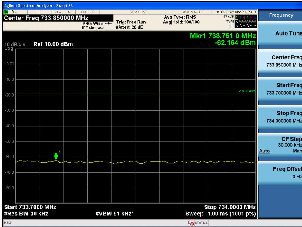
Out-of-Band Emissions / Lower 700 MHz / Downlink / CDMA / Lower Edge / AGC threshold +10 dB
