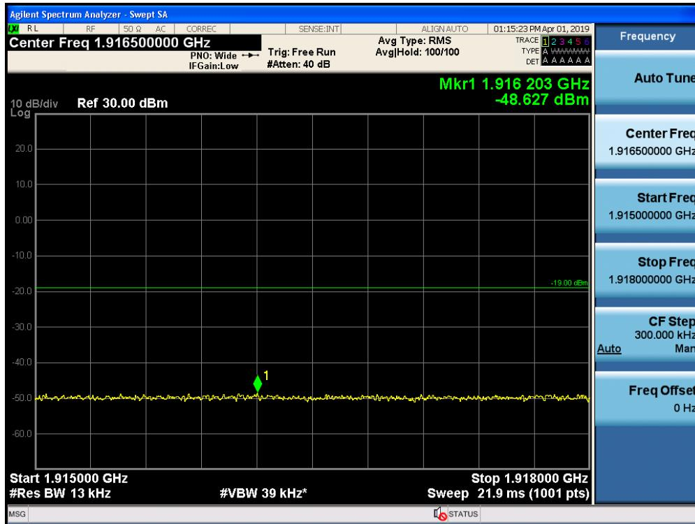
Out-of-Band Emissions / Broadband PCS / Uplink / CDMA / Upper Edge / AGC threshold +10 dB
