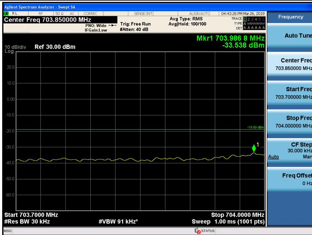
Out-of-Band Emissions / Lower 700 MHz / Uplink / CDMA / Upper Edge / AGC threshold
