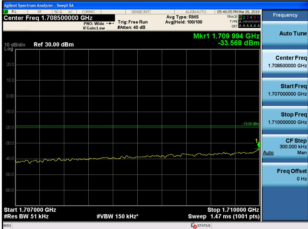
Out-of-Band Emissions / AWS-1 / Uplink / CDMA / Upper Edge / AGC threshold
