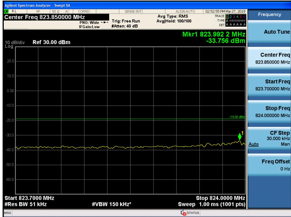
Out-of-Band Emissions / Cellular / Uplink / LTE 5 MHz / Lower Edge / AGC threshold +10 dB
