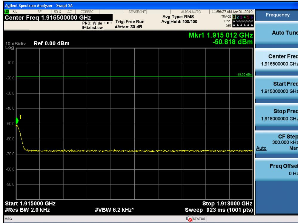
Out-of-Band Emissions / Broadband PCS / Uplink / GSM / Upper Edge / AGC threshold +10 dB
