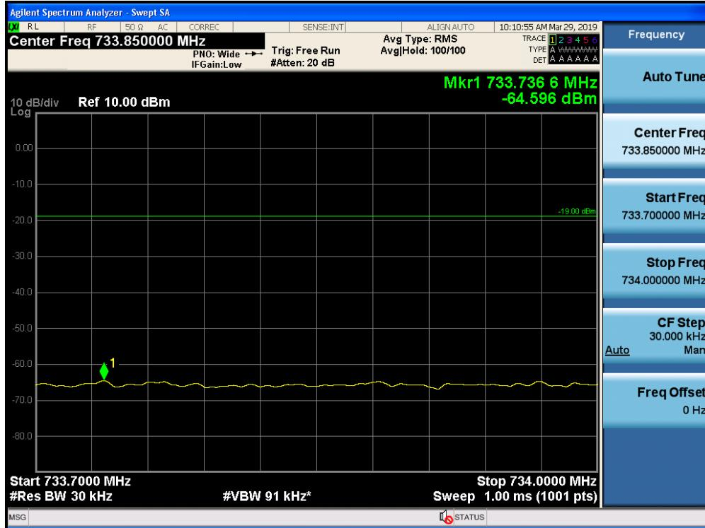
Out-of-Band Emissions / Upper 700 MHz / Downlink / GSM / Upper Edge / AGC threshold
