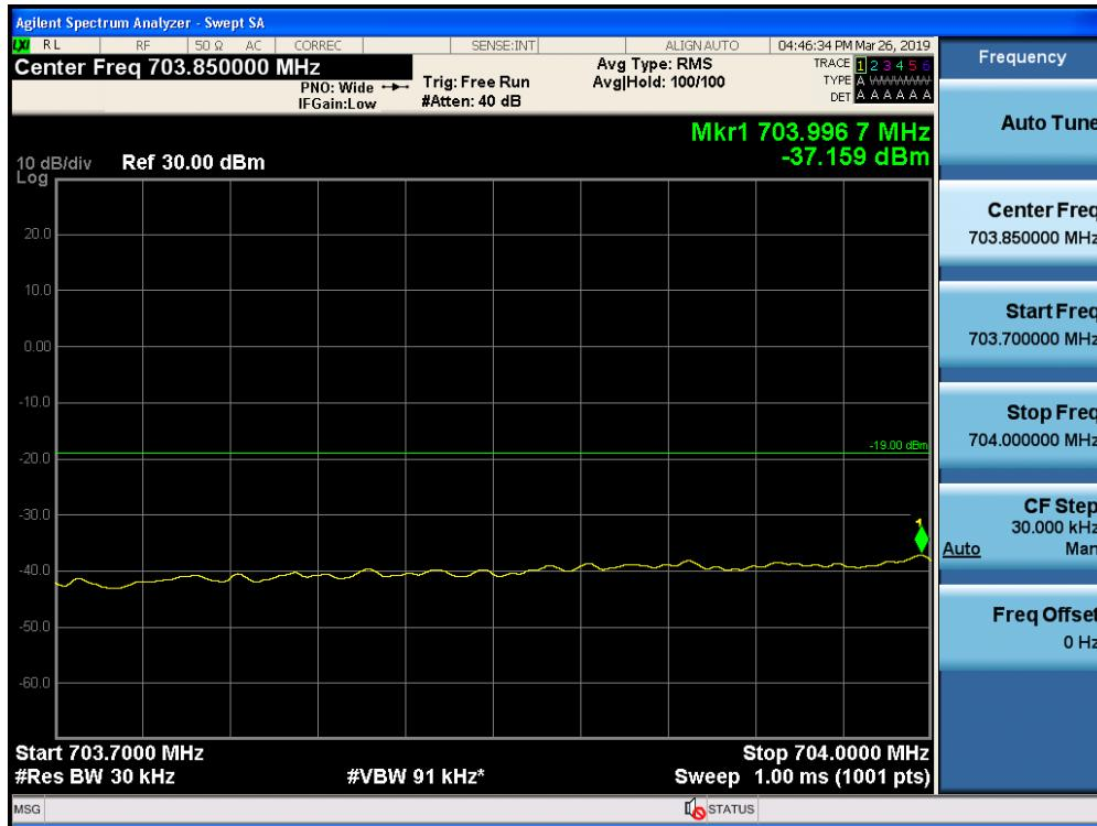
Out-of-Band Emissions / Upper 700 MHz / Uplink / GSM / Upper Edge / AGC threshold
