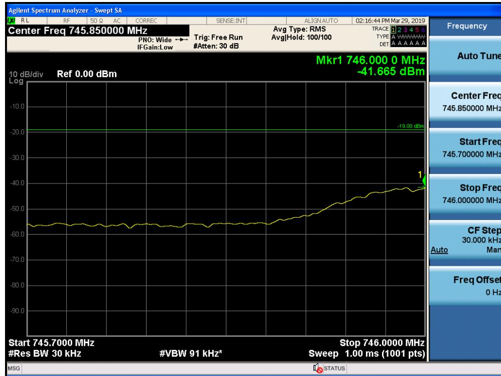
Out-of-Band Emissions / Upper 700 MHz / Downlink / LTE 5 MHz / Upper Edge / AGC threshold
