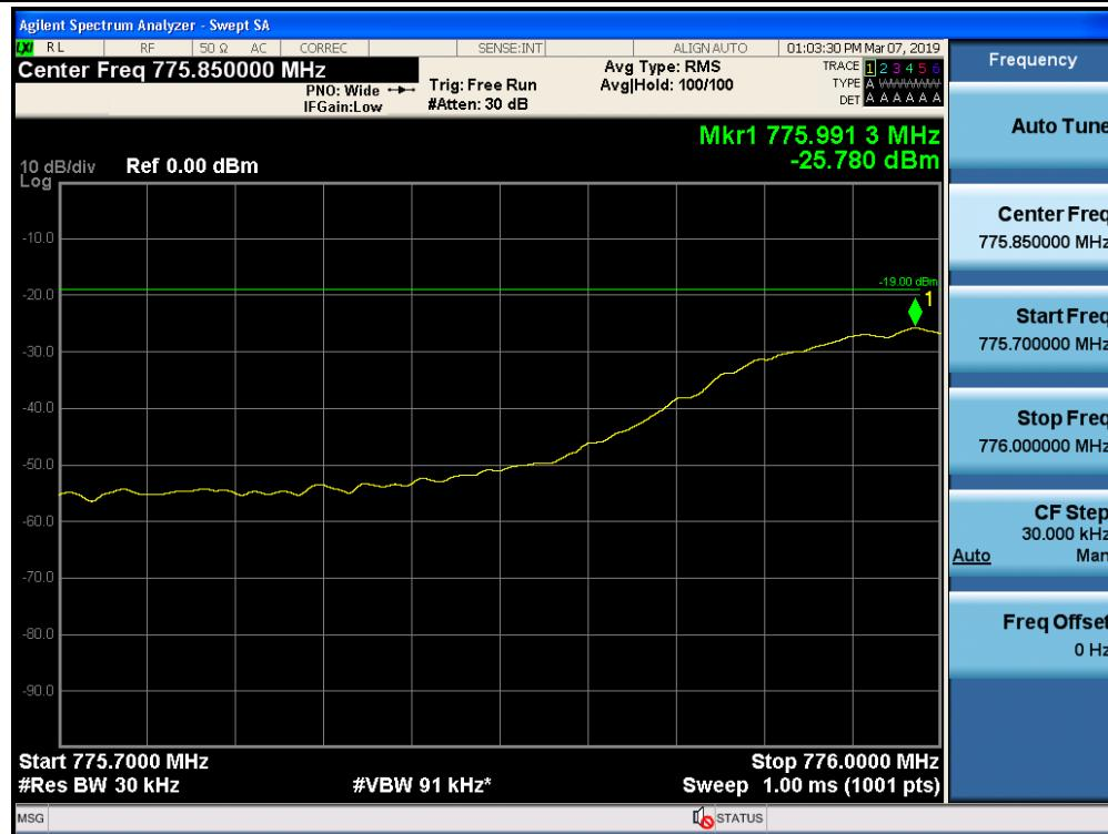
Out-of-Band Emissions / Upper 700 MHz / Uplink / GSM / Lower Edge / AGC threshold +10 dB
