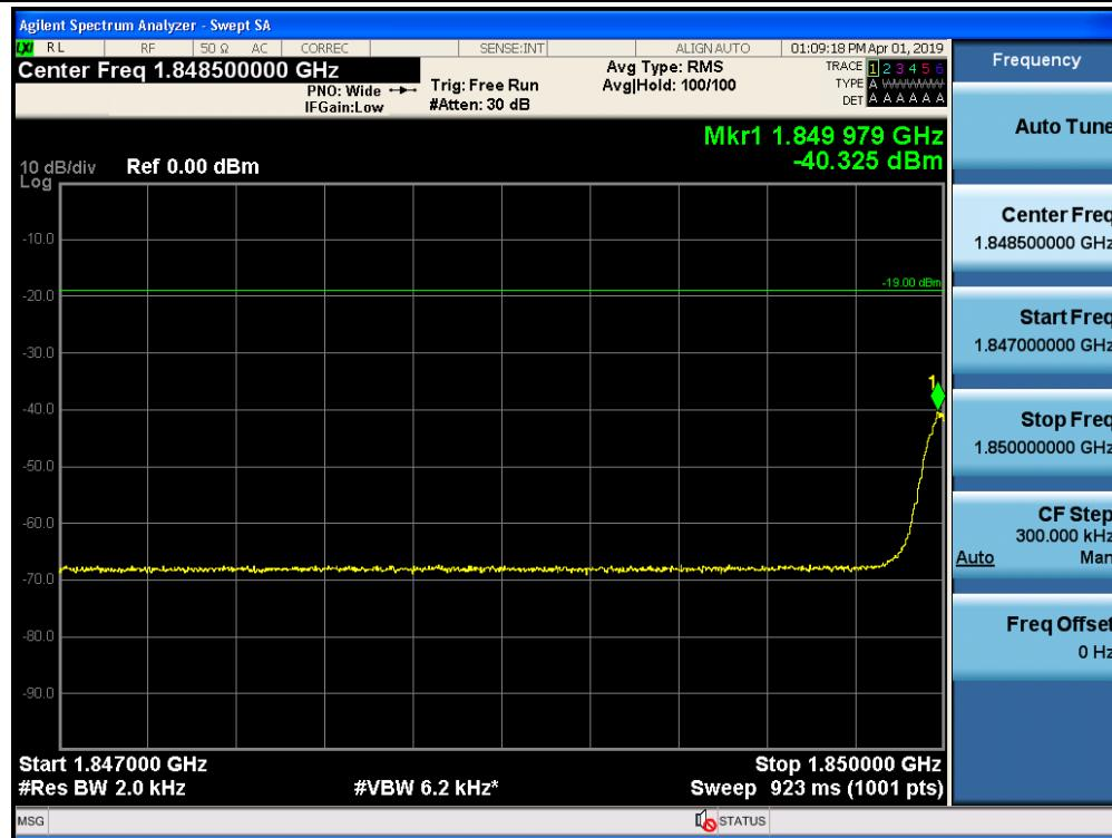
Out-of-Band Emissions / Broadband PCS / Uplink / LTE 5 MHz / Upper Edge / AGC threshold
