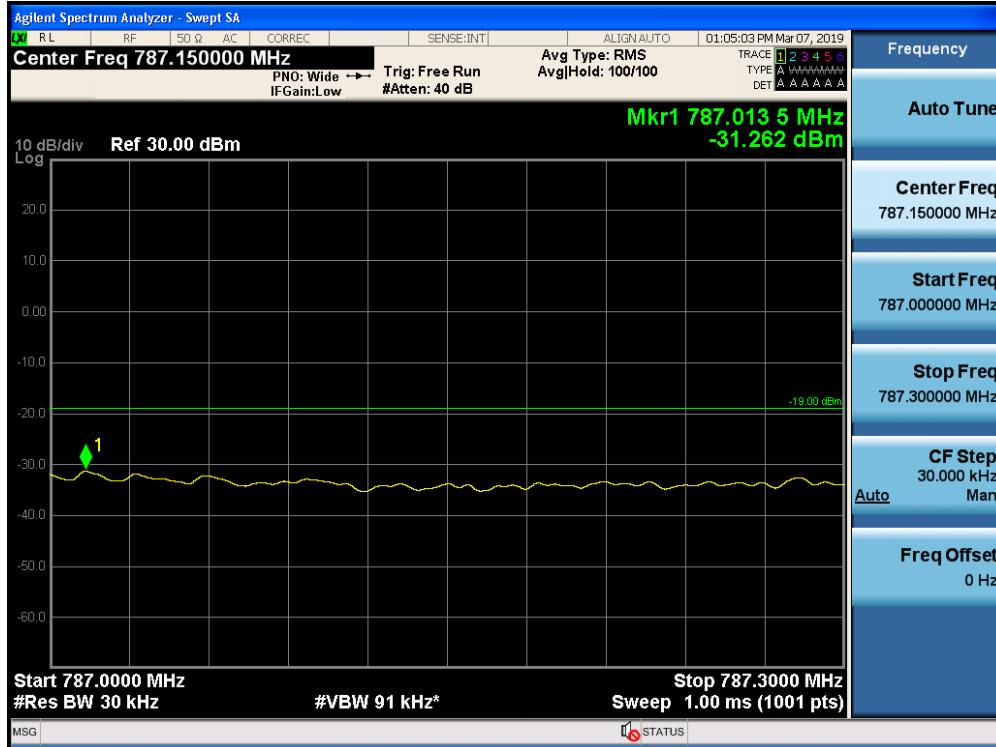
Out-of-Band Emissions / Upper 700 MHz / Uplink / LTE 5 MHz / Lower Edge / AGC threshold
