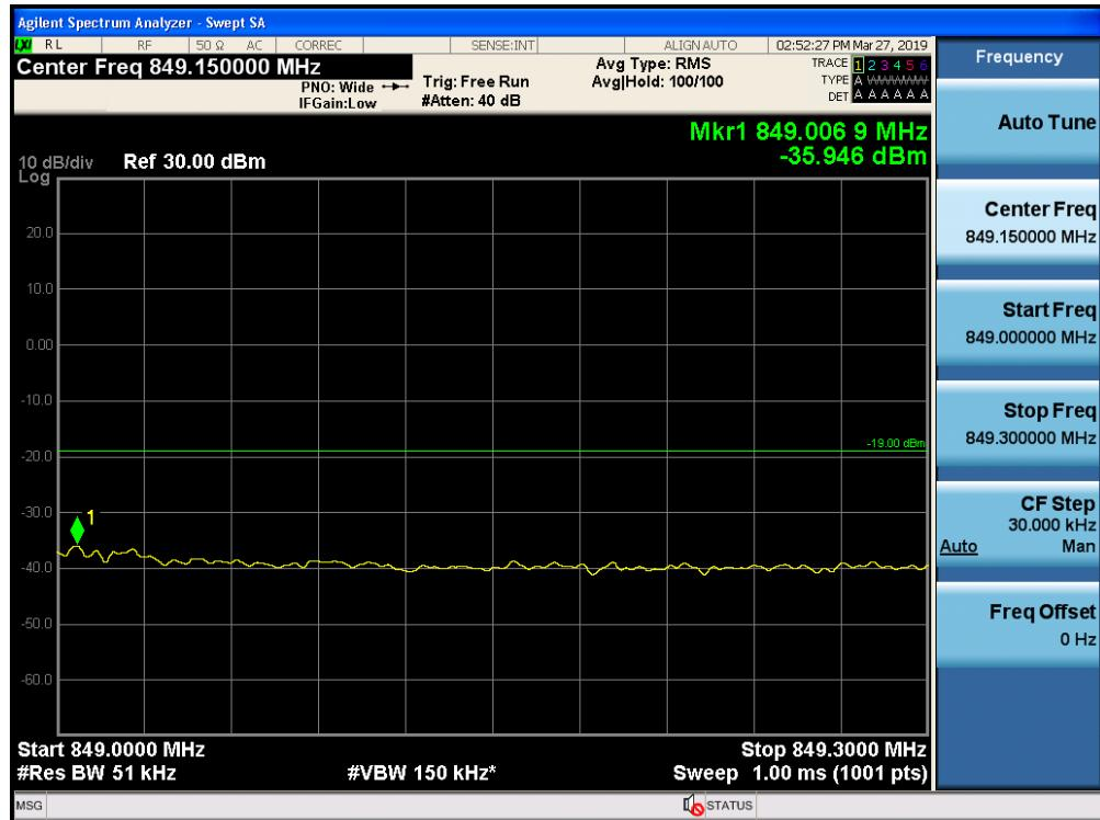
Out-of-Band Emissions / Cellular / Uplink / LTE 5 MHz / Lower Edge / AGC threshold
