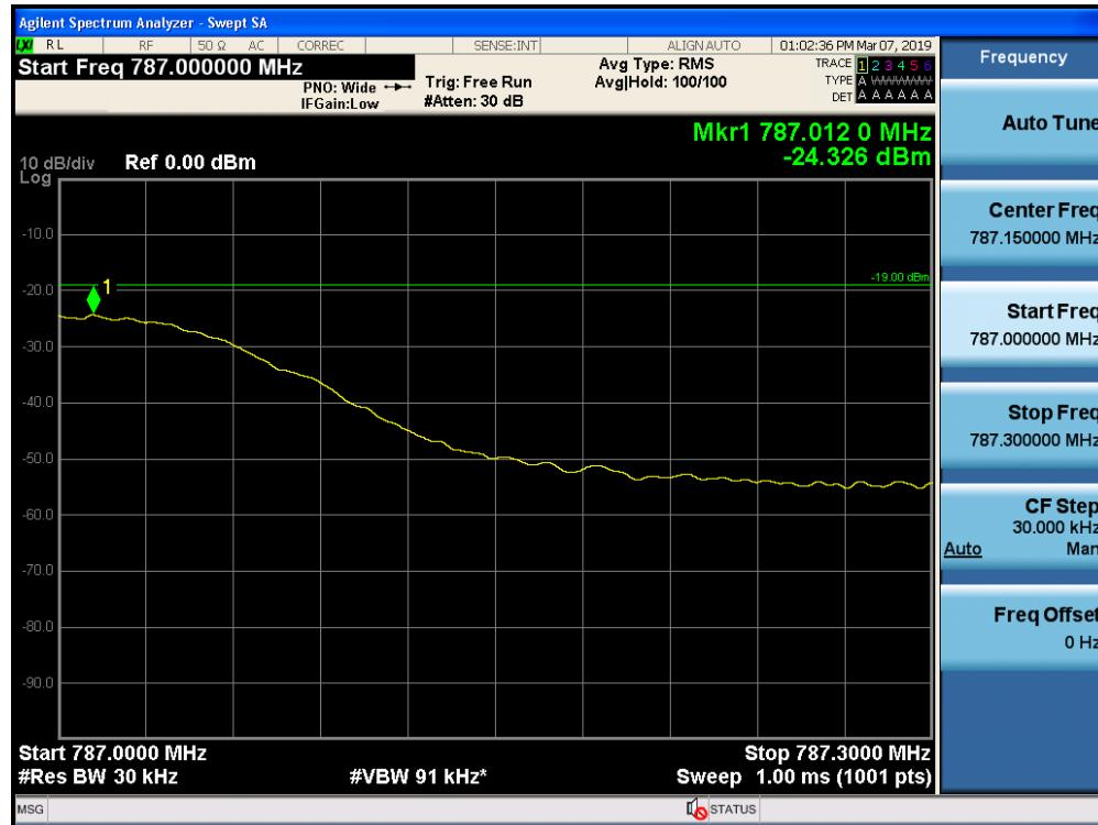
Out-of-Band Emissions / Upper 700 MHz / Uplink / GSM / Upper Edge / AGC threshold +10 dB
