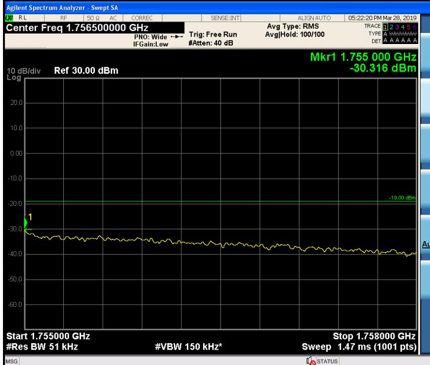
Out-of-Band Emissions / AWS-1 / Uplink / LTE 5 MHz / Upper Edge / AGC threshold +10 dB
