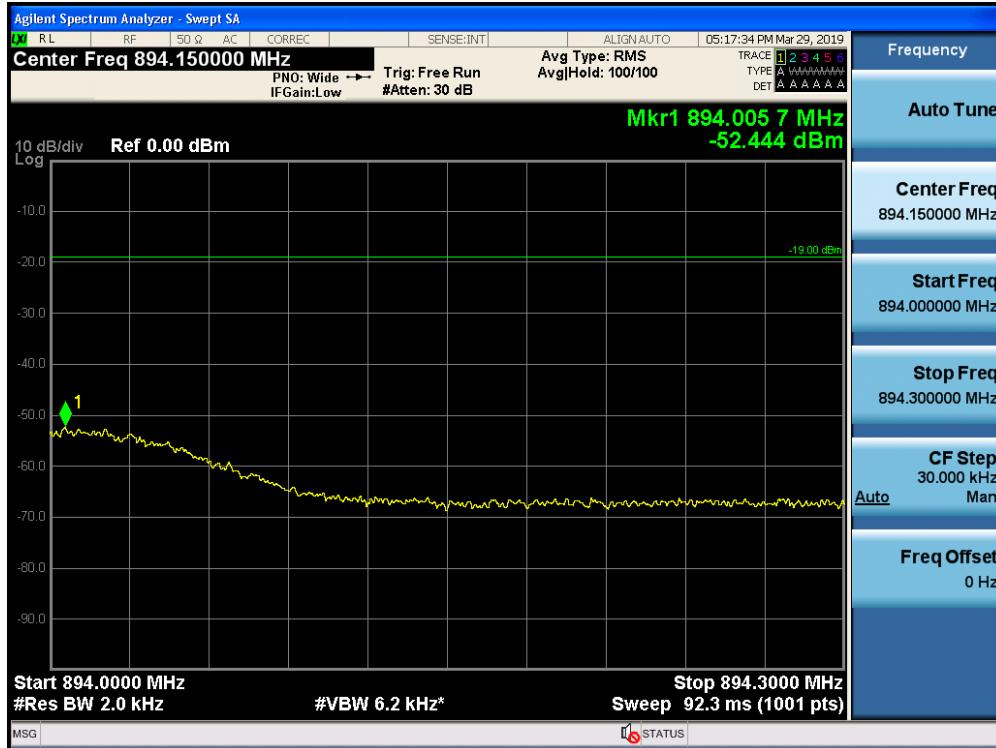
Out-of-Band Emissions / Cellular / Downlink / GSM / Upper Edge / AGC threshold +10 dB
