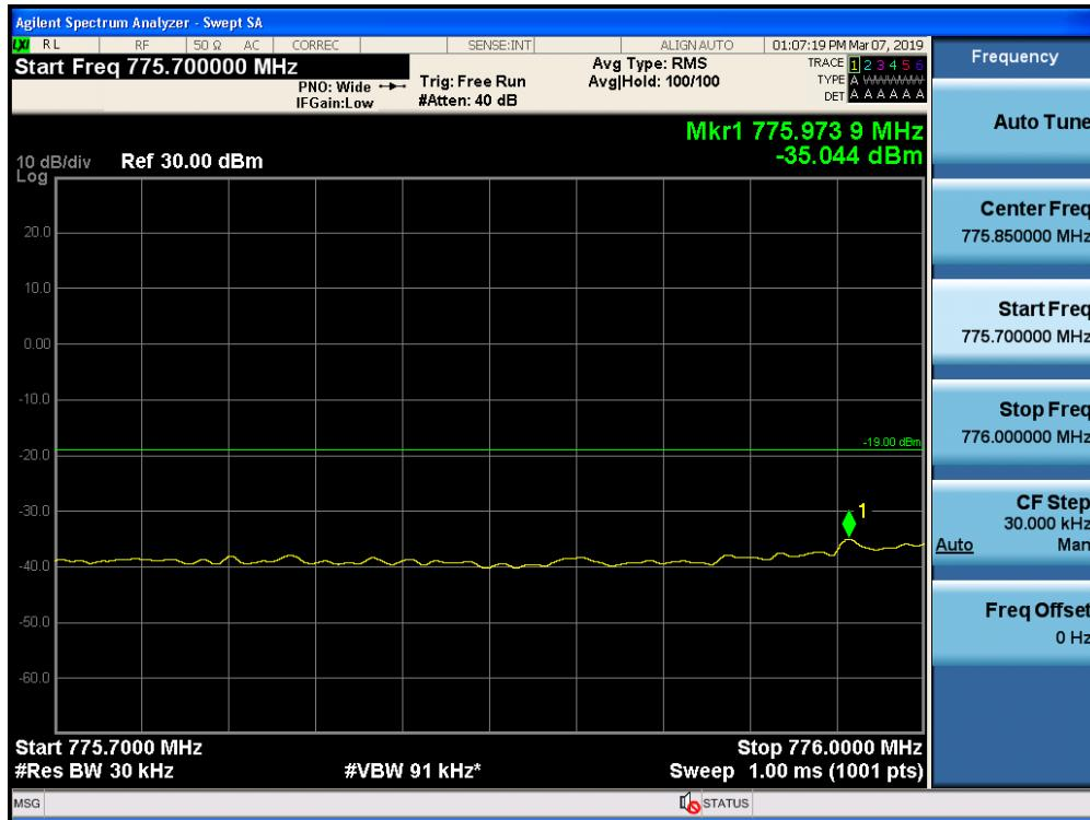
Out-of-Band Emissions / Upper 700 MHz / Uplink / CDMA / Upper Edge / AGC threshold
