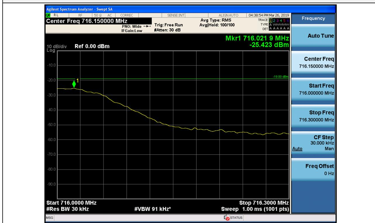
Out-of-Band Emissions / Lower 700 MHz / Uplink / GSM / Lower Edge / AGC threshold
