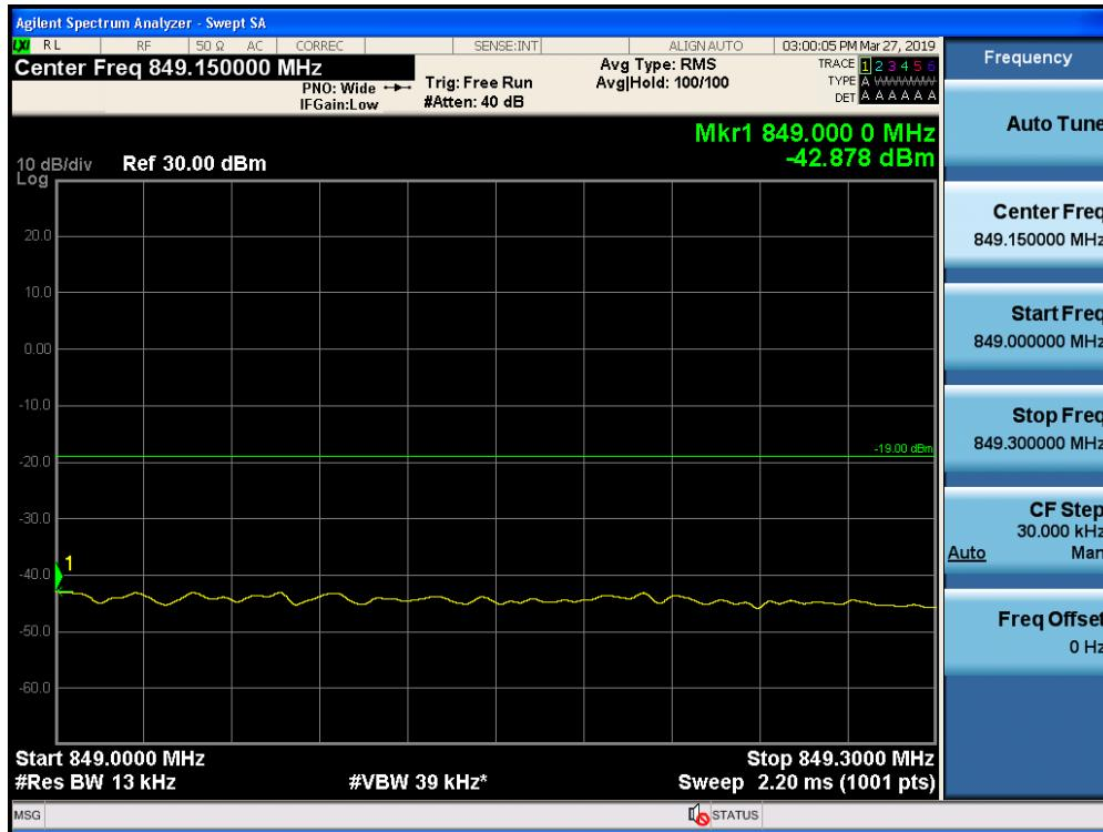
Out-of-Band Emissions / Cellular / Uplink / CDMA / Lower Edge / AGC threshold
