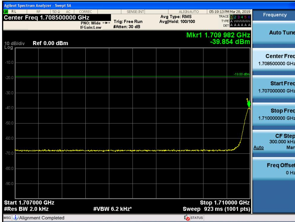
Out-of-Band Emissions / AWS-1 / Uplink / GSM / Lower Edge / AGC threshold +10 dB
