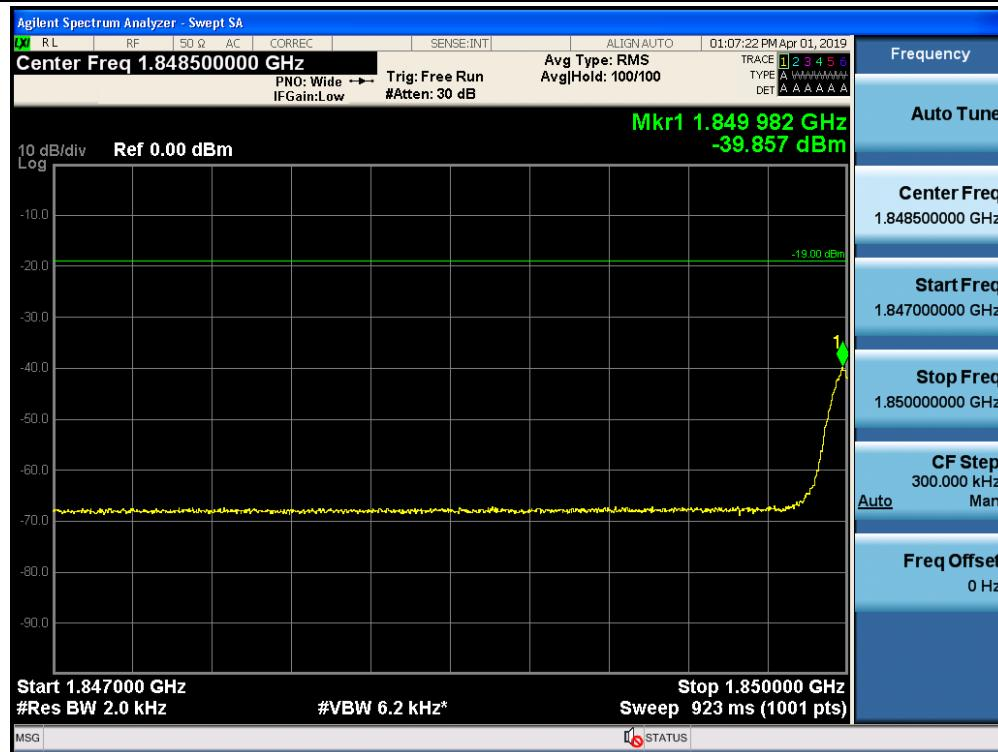
Out-of-Band Emissions / Broadband PCS / Uplink / GSM / Lower Edge / AGC threshold +10 dB
