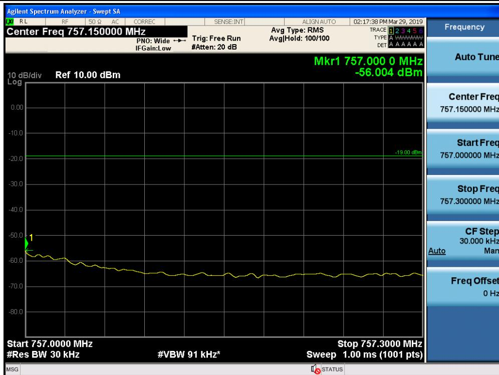
Out-of-Band Emissions / Upper 700 MHz / Downlink / LTE 5 MHz / Lower Edge / AGC threshold
