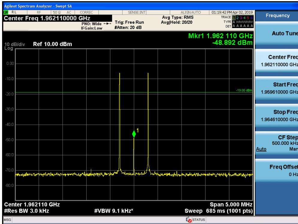
Intermodulation / Broadband PCS / Downlink / AGC threshold +10 dB
