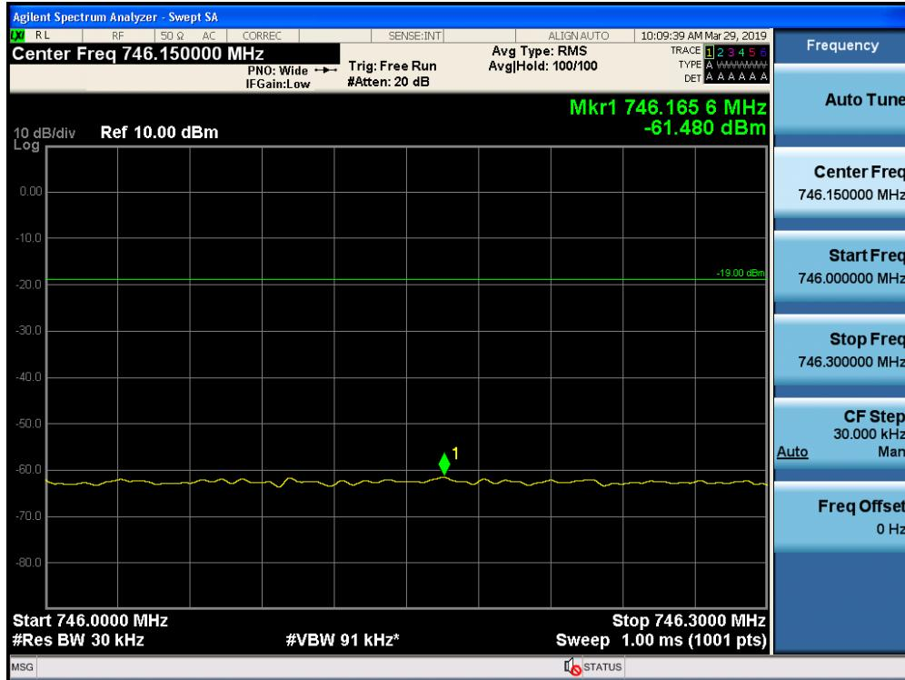
Out-of-Band Emissions / Lower 700 MHz / Downlink / CDMA / Upper Edge / AGC threshold +10 dB
