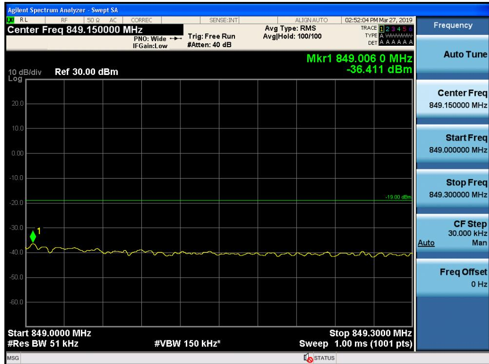
Out-of-Band Emissions / Cellular / Uplink / LTE 5 MHz / Upper Edge / AGC threshold +10 dB
