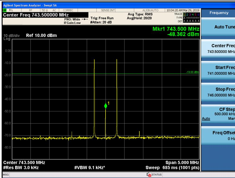
Intermodulation / Lower 700 MHz / Downlink / AGC threshold +10 dB
