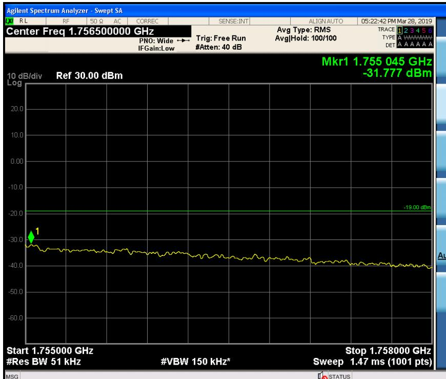
Out-of-Band Emissions / AWS-1 / Uplink / LTE 5 MHz / Lower Edge / AGC threshold
