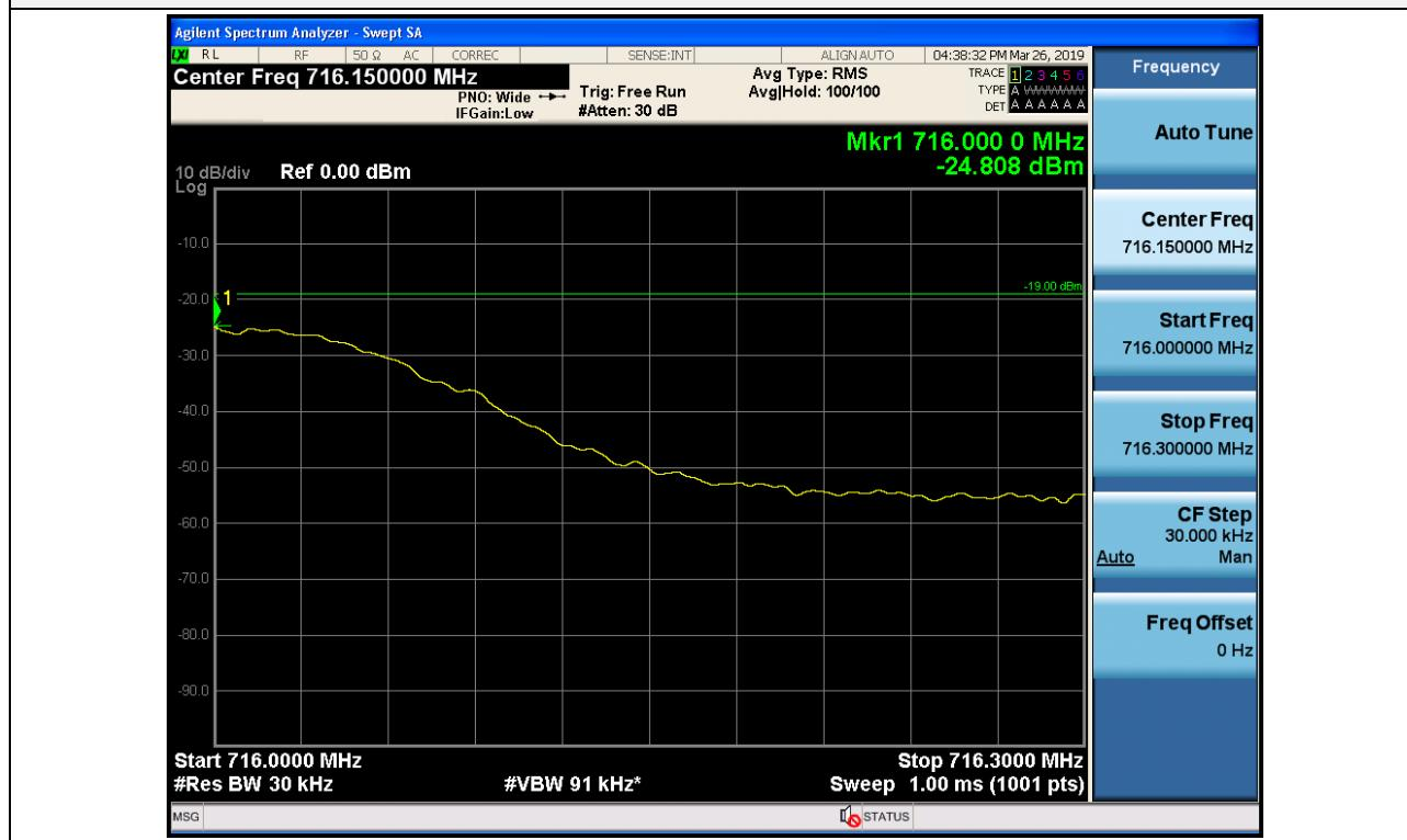
Out-of-Band Emissions / Lower 700 MHz / Uplink / GSM / Upper Edge / AGC threshold +10 dB
