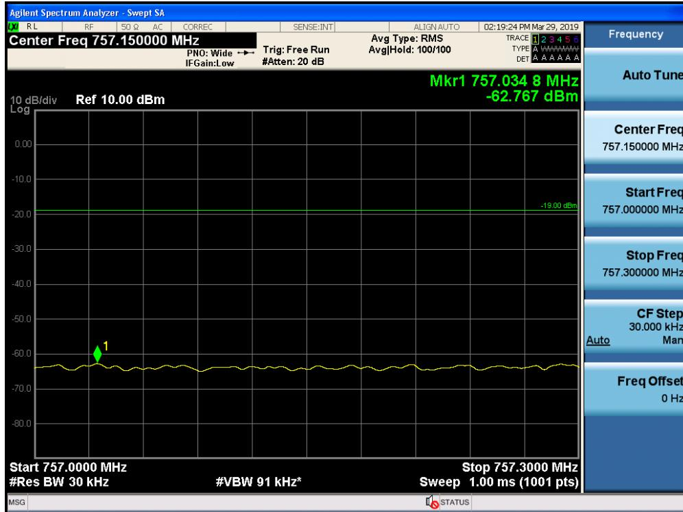
Out-of-Band Emissions / Upper 700 MHz / Downlink / CDMA / Upper Edge / AGC threshold +10 dB
