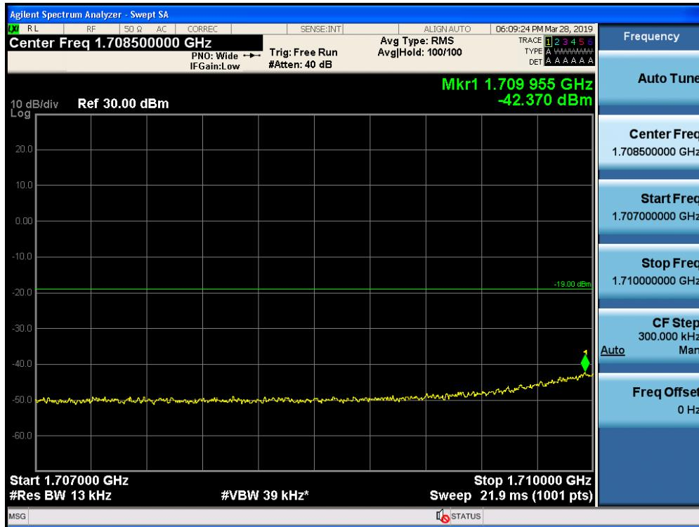
Out-of-Band Emissions / Broadband PCS / Uplink / GSM / Upper Edge / AGC threshold
