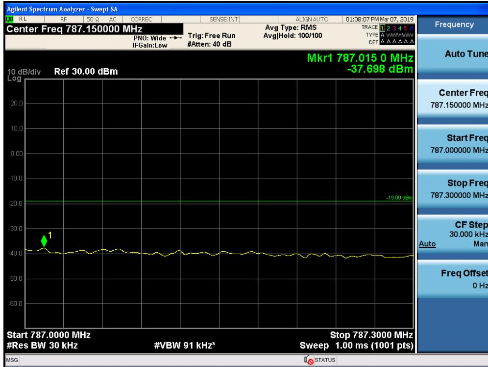
Out-of-Band Emissions / Upper 700 MHz / Uplink / CDMA / Upper Edge / AGC threshold +10 dB
