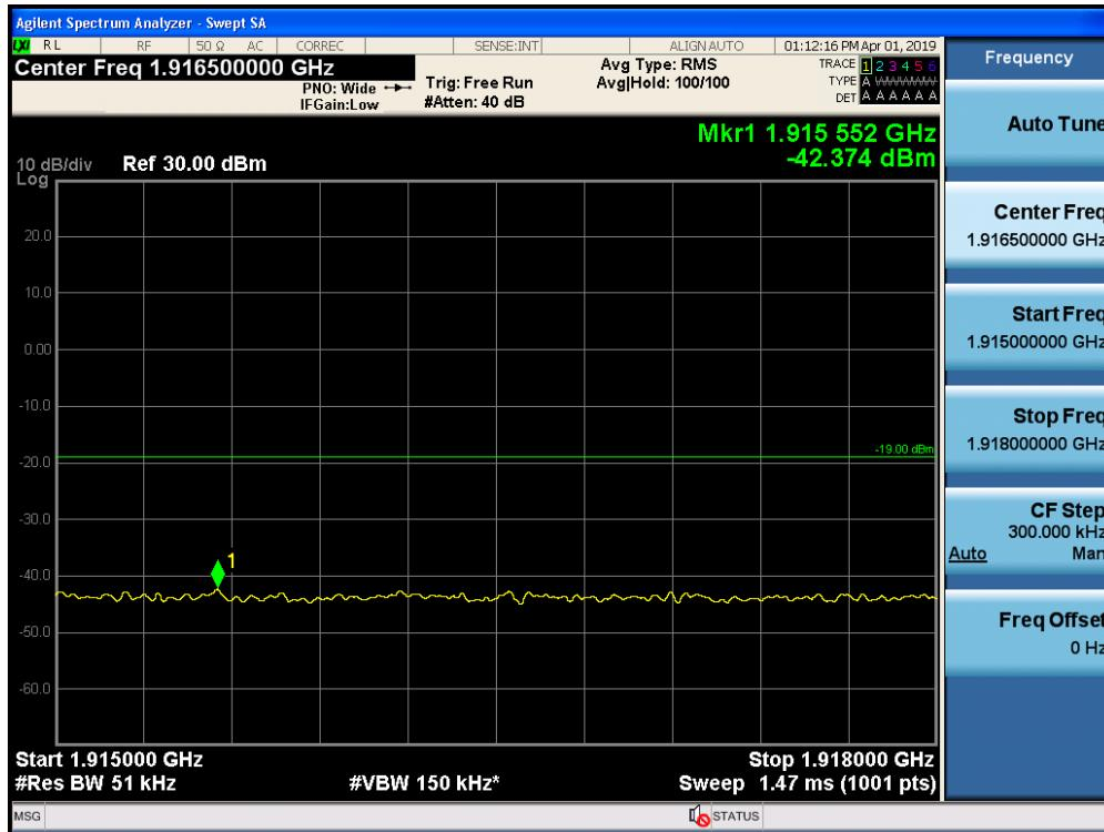
Out-of-Band Emissions / Broadband PCS / Uplink / LTE 5 MHz / Upper Edge / AGC threshold +10 dB
