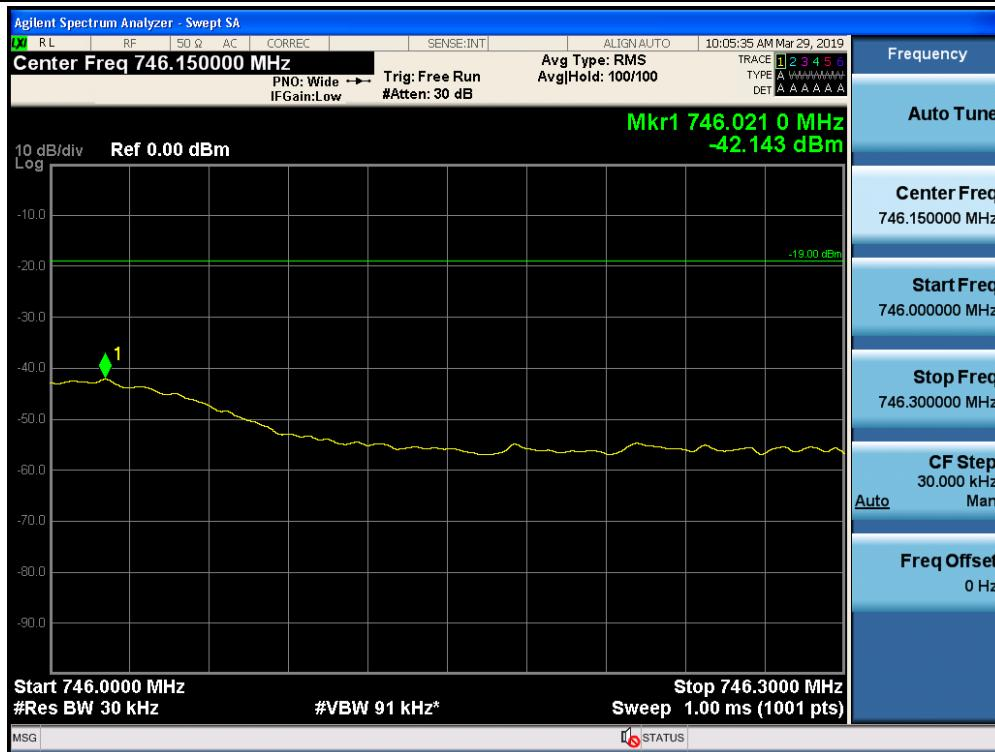
Out-of-Band Emissions / Lower 700 MHz / Downlink / GSM / Upper Edge / AGC threshold +10 dB
