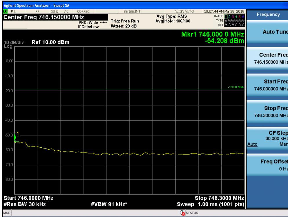
Out-of-Band Emissions / Lower 700 MHz / Downlink / LTE 5 MHz / Upper Edge / AGC threshold +10 dB
