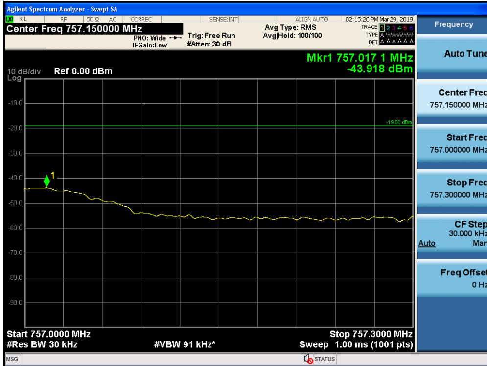
Out-of-Band Emissions / Upper 700 MHz / Downlink / GSM / Upper Edge / AGC threshold +10 dB
