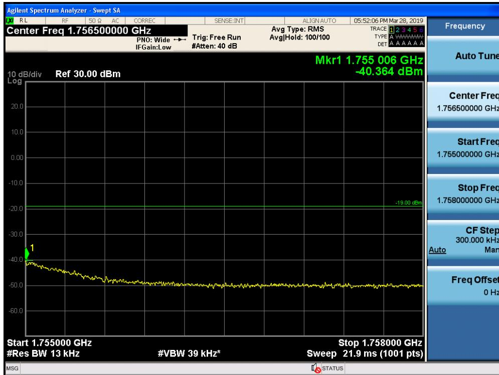
Out-of-Band Emissions / AWS-1 / Uplink / CDMA / Lower Edge / AGC threshold
