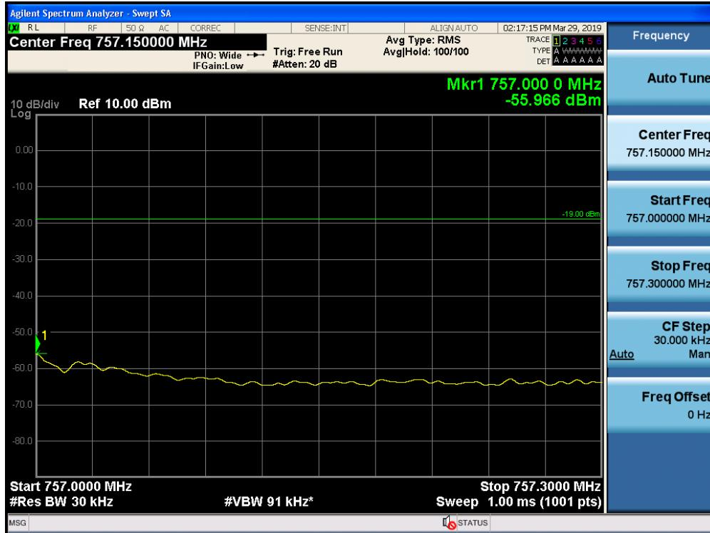
Out-of-Band Emissions / Upper 700 MHz / Downlink / LTE 5 MHz / Upper Edge / AGC threshold +10 dB
