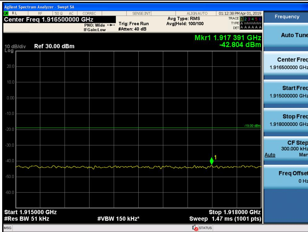
Out-of-Band Emissions / Broadband PCS / Uplink / LTE 5 MHz / Lower Edge / AGC threshold
