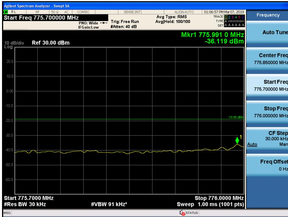
Out-of-Band Emissions / Upper 700 MHz / Uplink / LTE 5 MHz / Lower Edge / AGC threshold +10 dB
