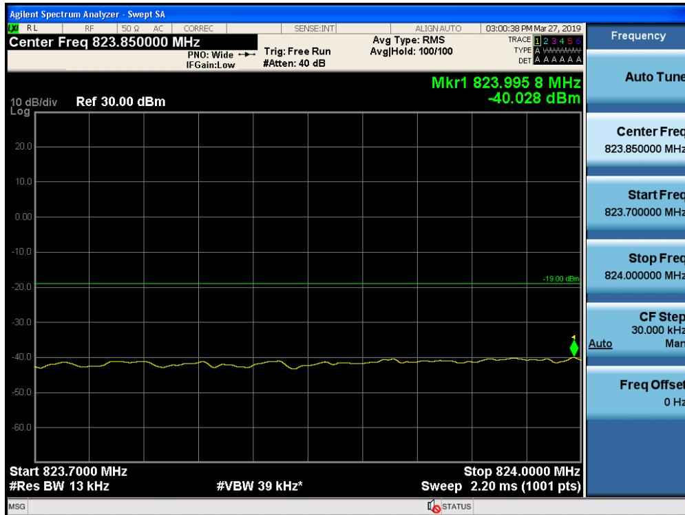
Out-of-Band Emissions / Cellular / Uplink / CDMA / Lower Edge / AGC threshold +10 dB
