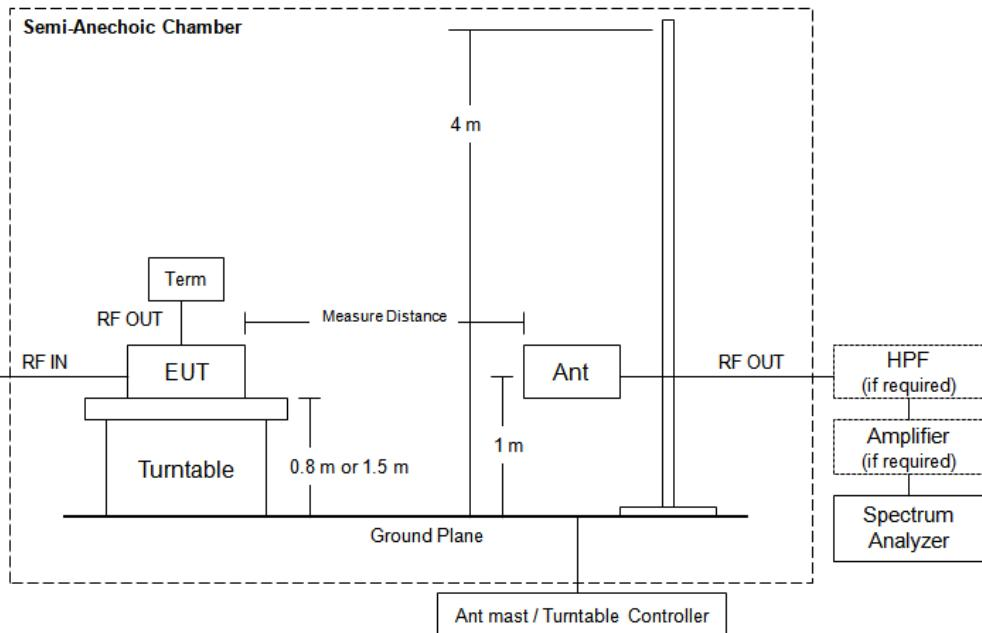
\* EUT position is refer to placement of tabletop refer to section 5.5.2.3.1 of ANSI C63.26-2015
