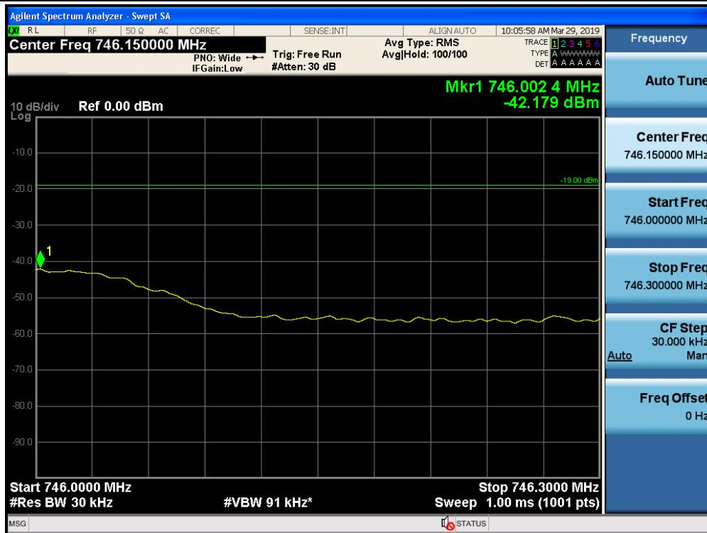
Out-of-Band Emissions / Lower 700 MHz / Downlink / GSM / Lower Edge / AGC threshold
