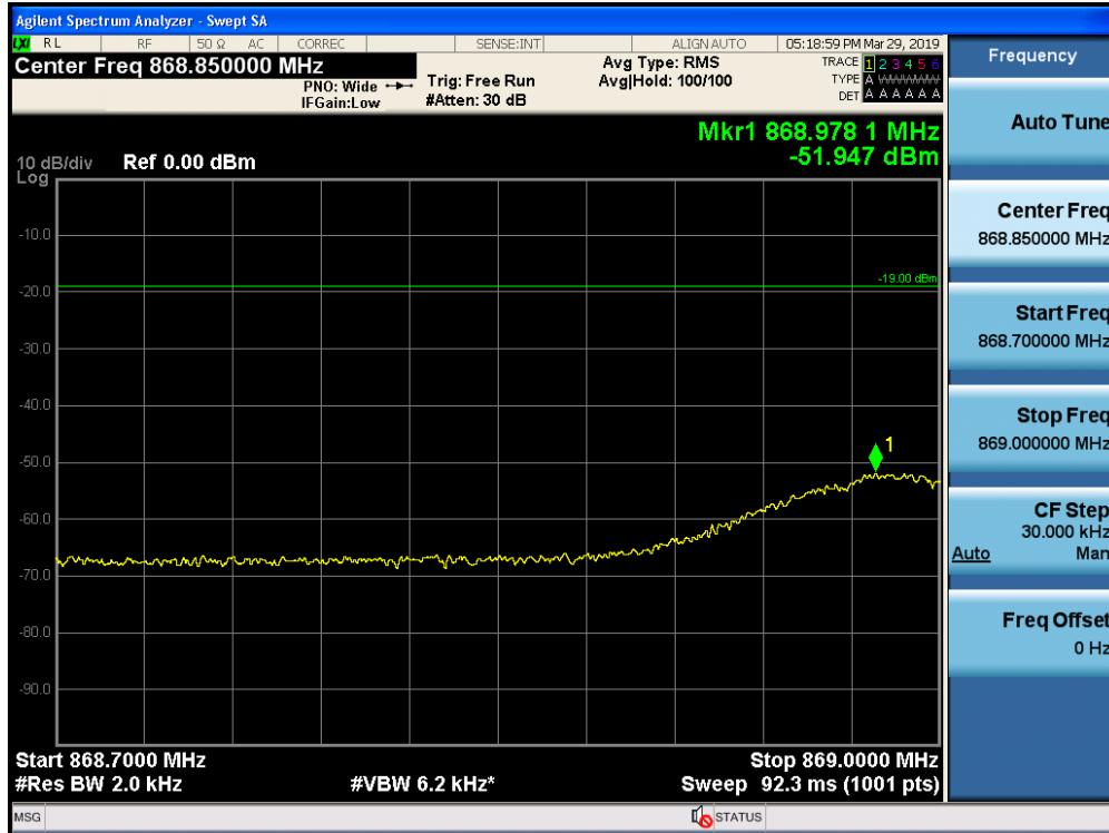
Out-of-Band Emissions / Cellular / Downlink / GSM / Lower Edge / AGC threshold +10 dB
