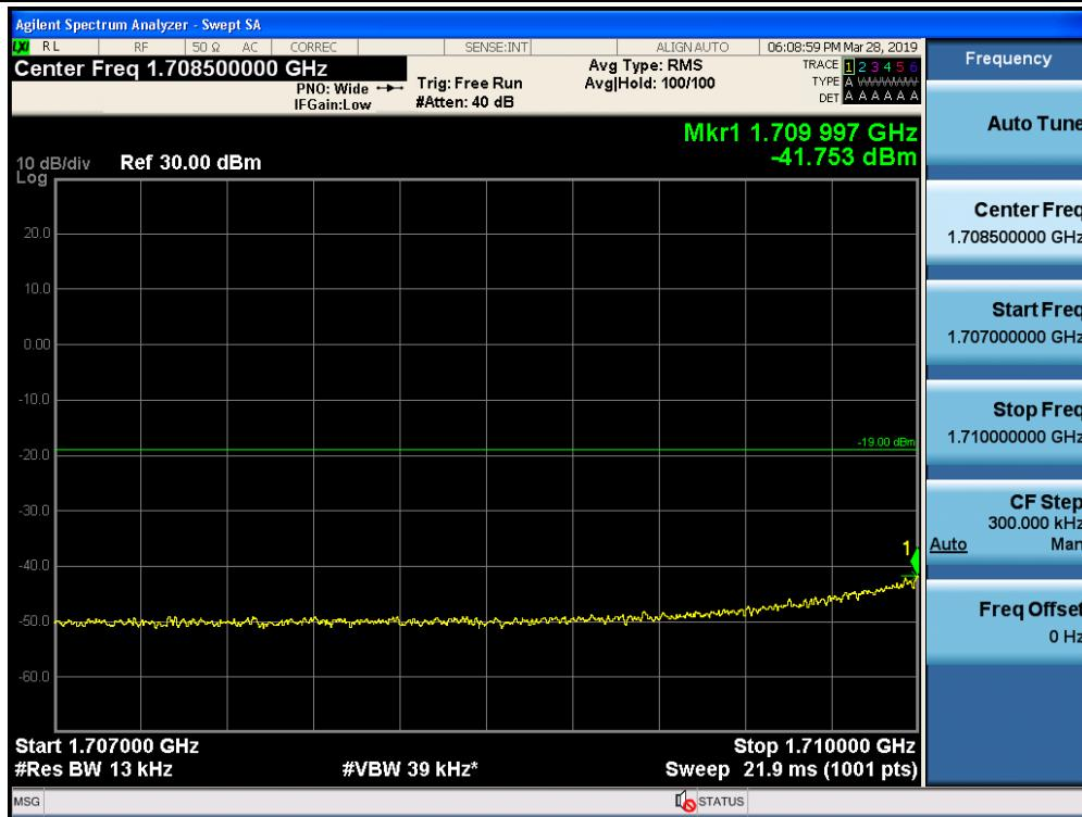
Out-of-Band Emissions / AWS-1 / Uplink / CDMA / Lower Edge / AGC threshold +10 dB
