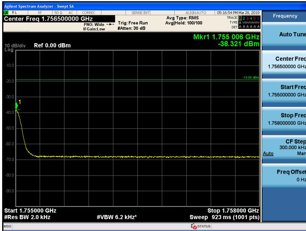
Out-of-Band Emissions / AWS-1 / Uplink / GSM / Lower Edge / AGC threshold
