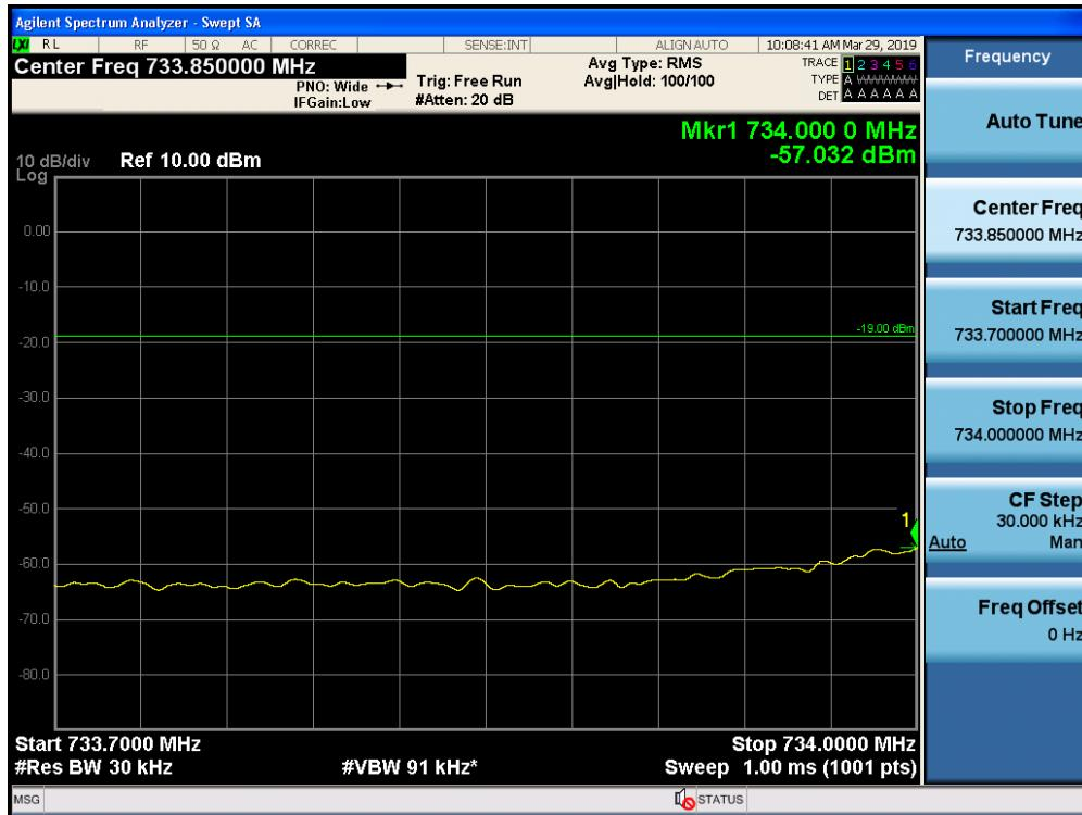
Out-of-Band Emissions / Lower 700 MHz / Downlink / LTE 5 MHz / Lower Edge / AGC threshold +10 dB
