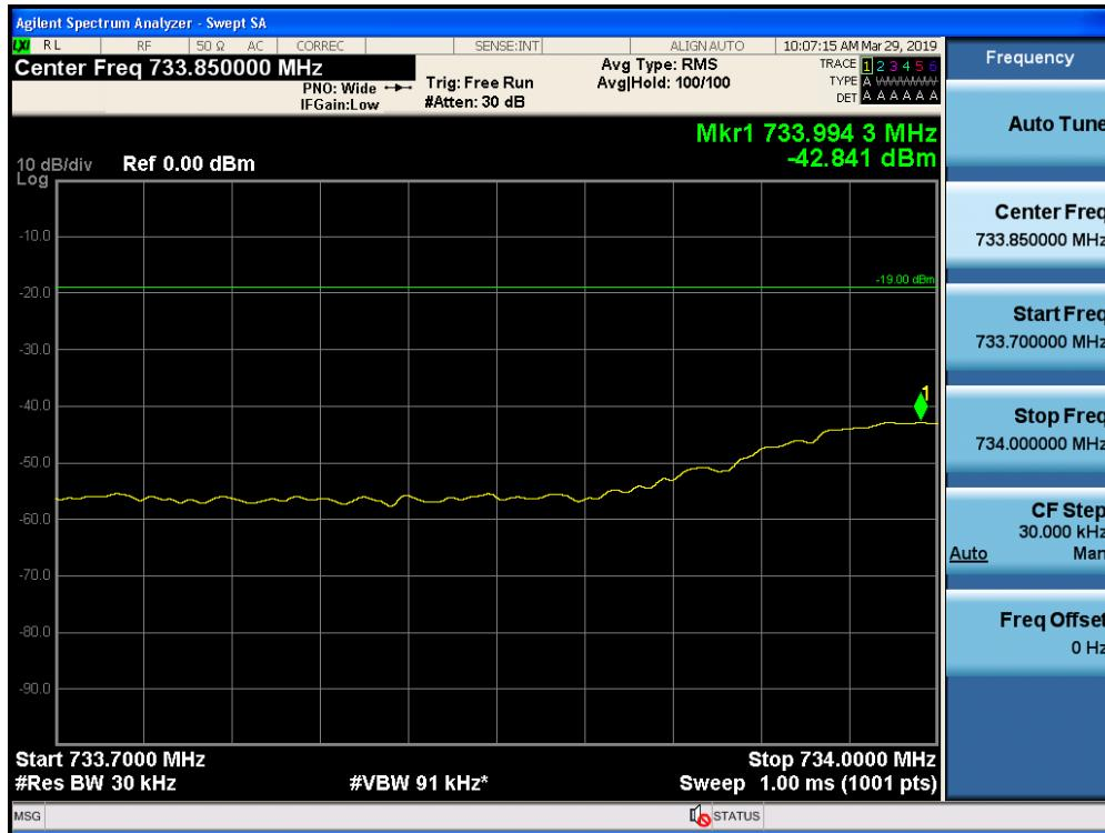
Out-of-Band Emissions / Lower 700 MHz / Downlink / LTE 5 MHz / Upper Edge / AGC threshold
