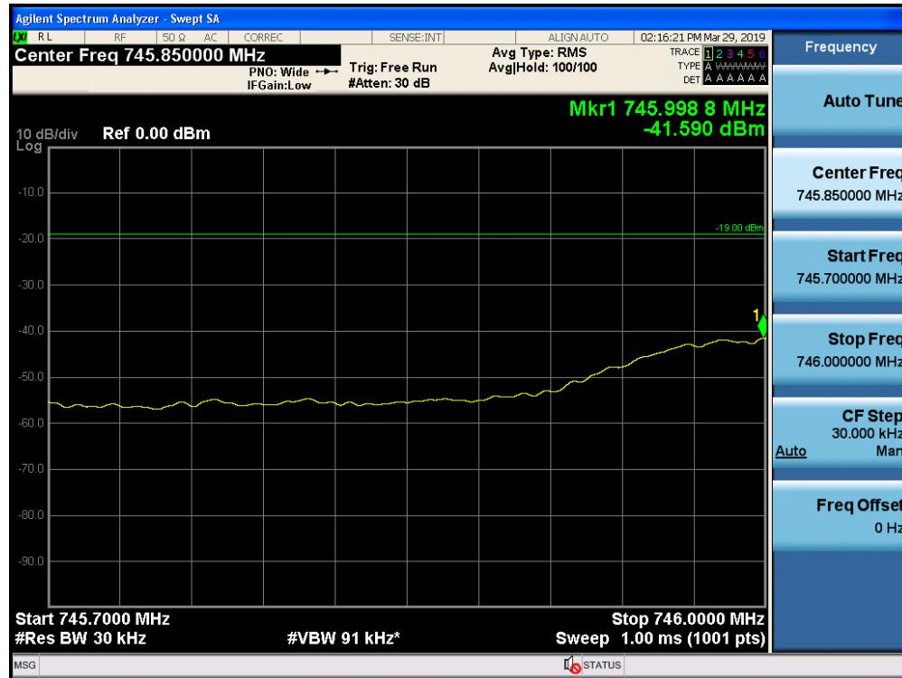
Out-of-Band Emissions / Upper 700 MHz / Downlink / GSM / Lower Edge / AGC threshold +10 dB
