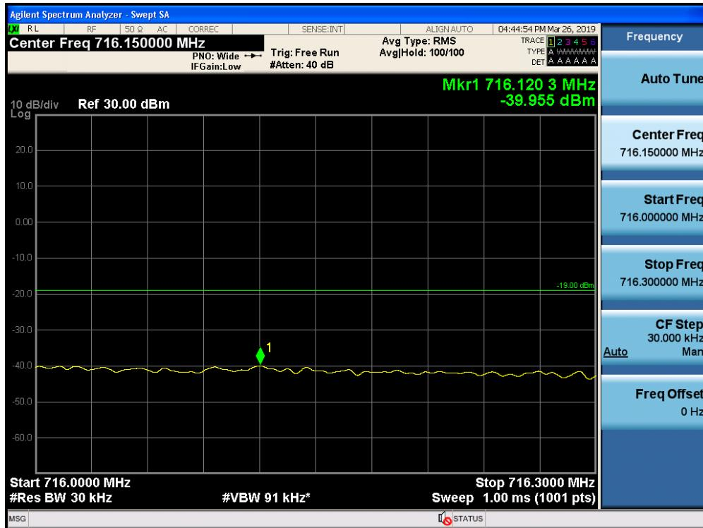
Out-of-Band Emissions / Lower 700 MHz / Uplink / CDMA / Lower Edge / AGC threshold
