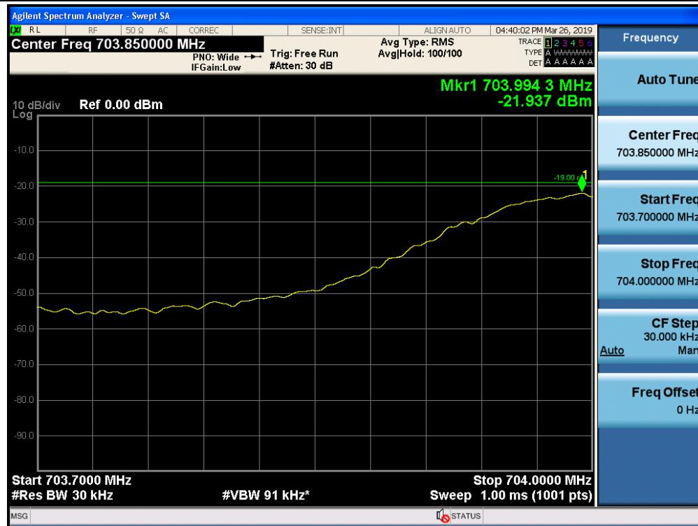
Out-of-Band Emissions / Lower 700 MHz / Uplink / GSM / Lower Edge / AGC threshold +10 dB
