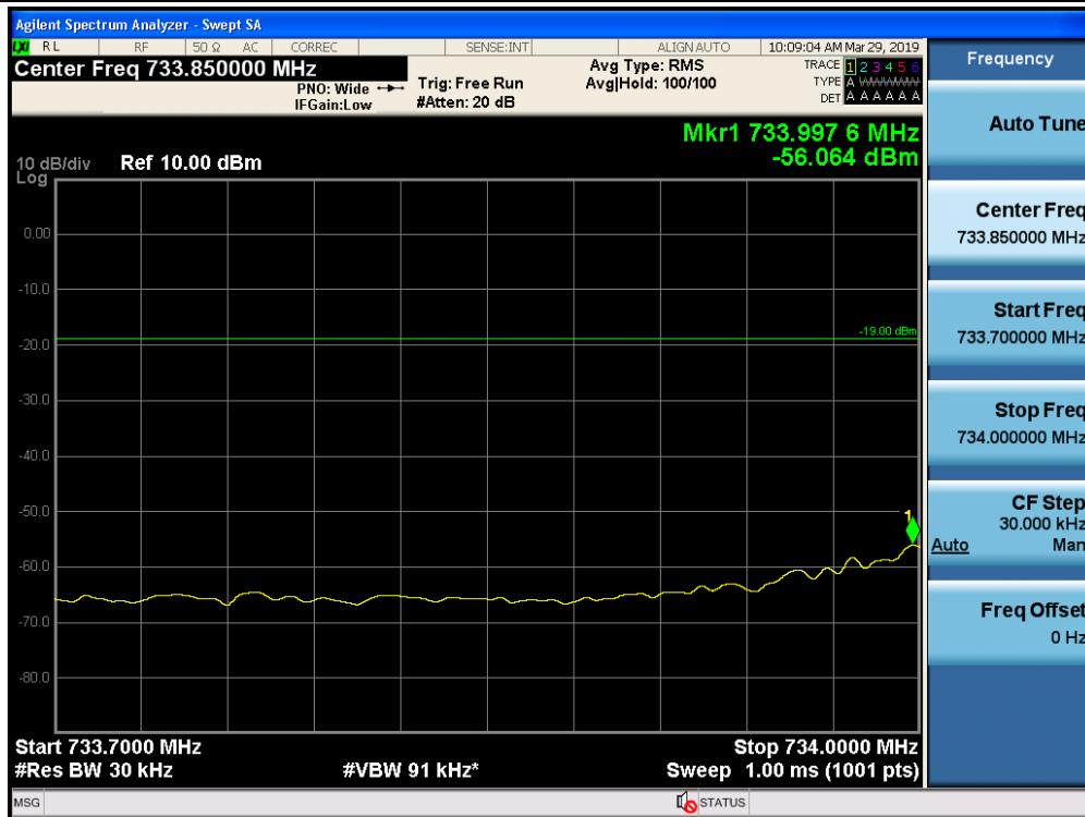
Out-of-Band Emissions / Lower 700 MHz / Downlink / CDMA / Upper Edge / AGC threshold
