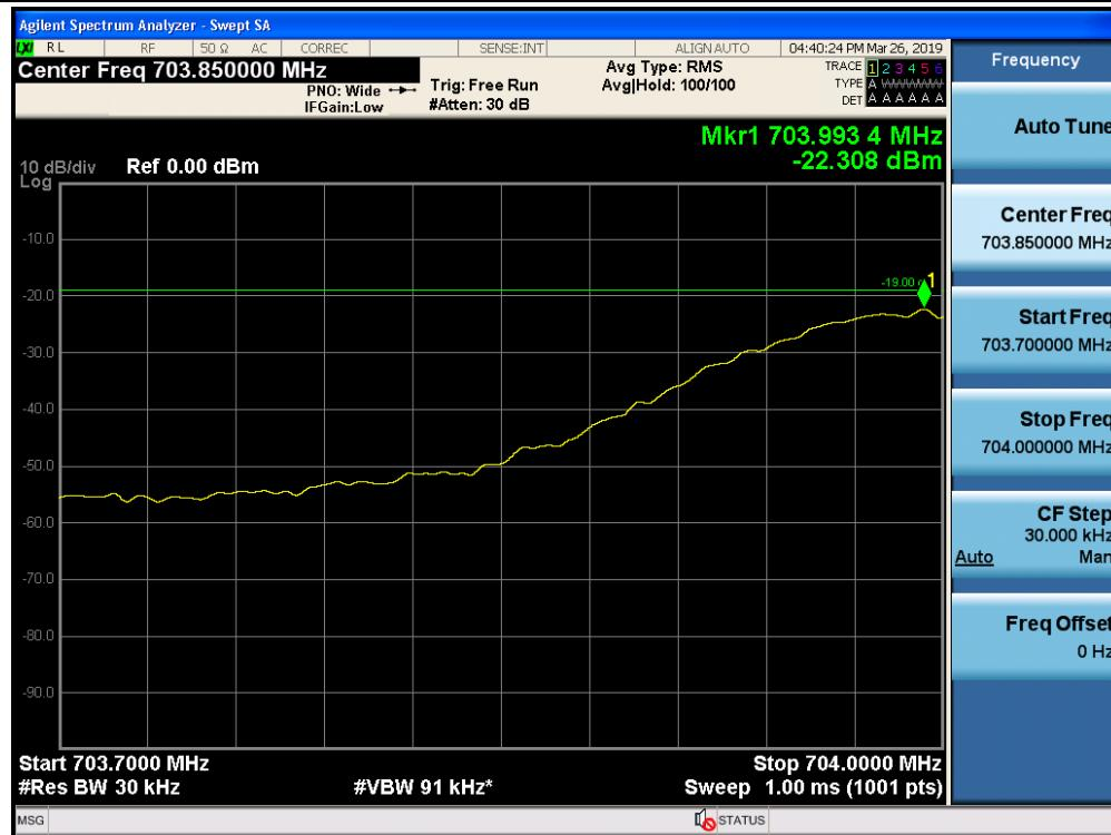
Out-of-Band Emissions / Lower 700 MHz / Uplink / LTE 5 MHz / Upper Edge / AGC threshold
