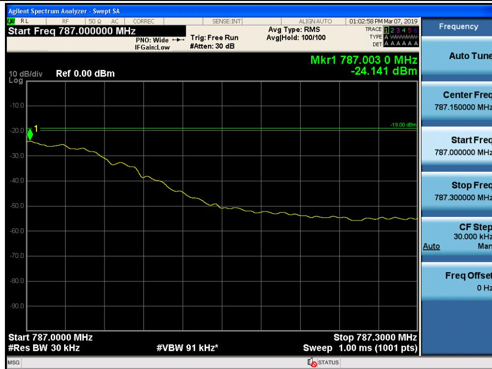
Out-of-Band Emissions / Upper 700 MHz / Uplink / GSM / Lower Edge / AGC threshold
