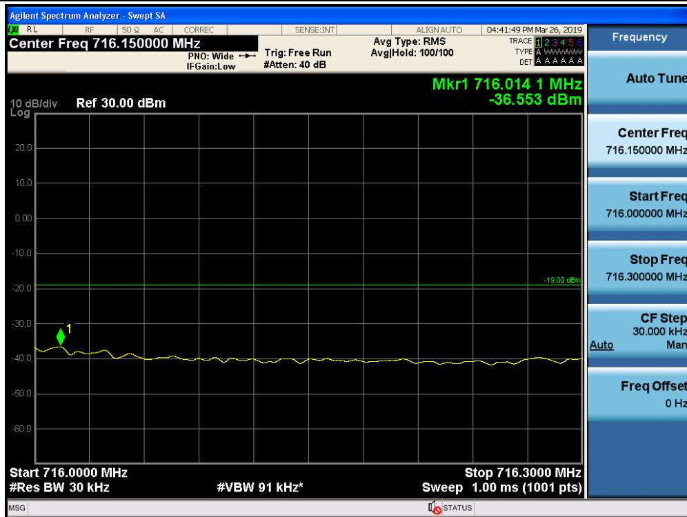
Out-of-Band Emissions / Lower 700 MHz / Uplink / LTE 5 MHz / Lower Edge / AGC threshold
