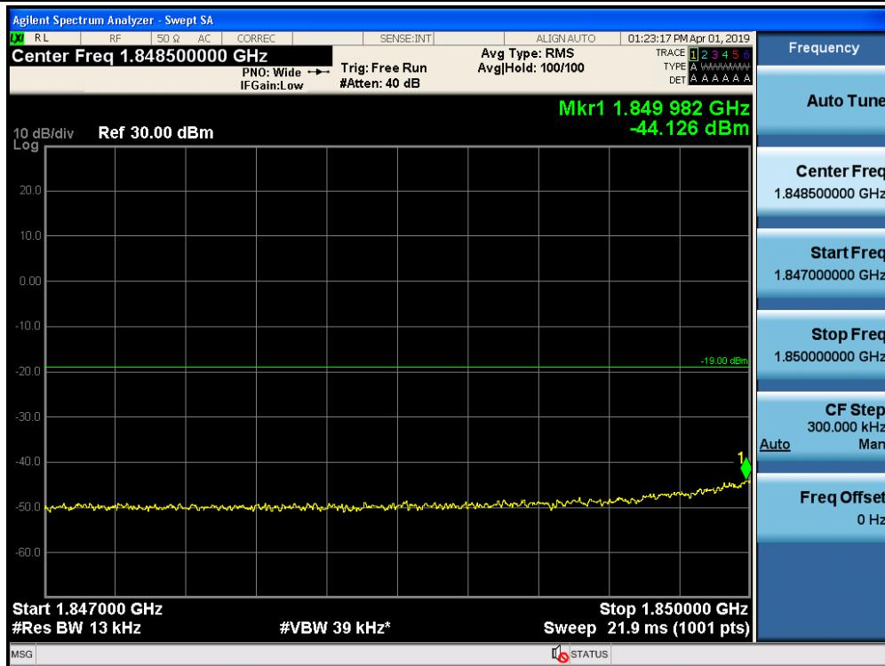
Out-of-Band Emissions / Lower 700 MHz / Downlink / GSM / Upper Edge / AGC threshold
