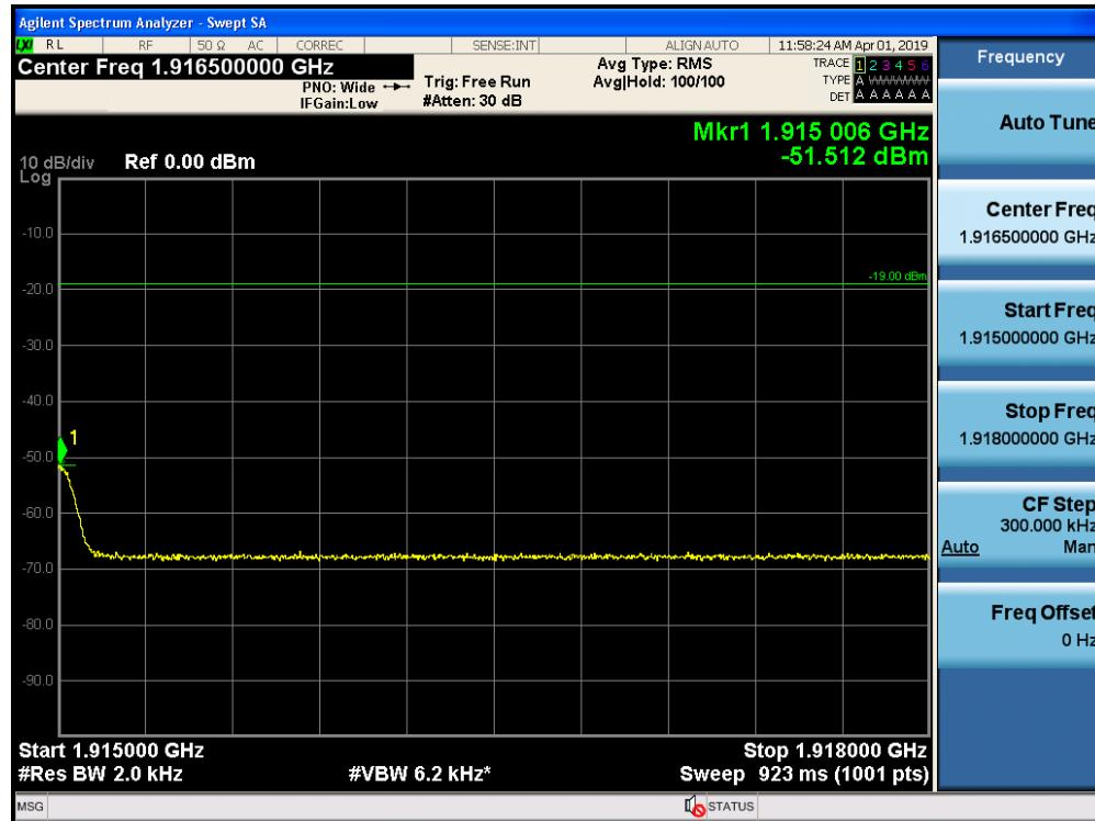
Out-of-Band Emissions / Broadband PCS / Uplink / GSM / Lower Edge / AGC threshold
