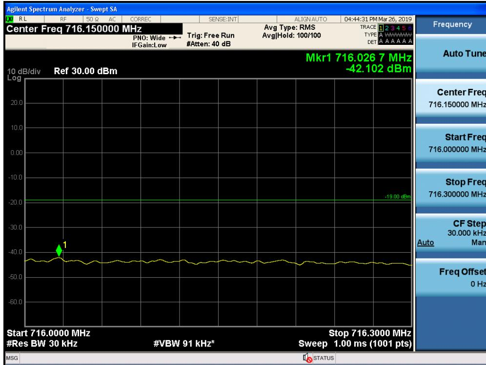
Out-of-Band Emissions / Lower 700 MHz / Uplink / CDMA / Upper Edge / AGC threshold +10 dB
