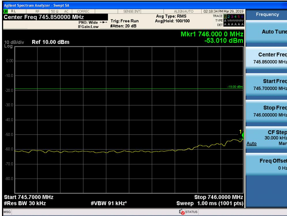
Out-of-Band Emissions / Upper 700 MHz / Downlink / LTE 5 MHz / Lower Edge / AGC threshold +10 dB
