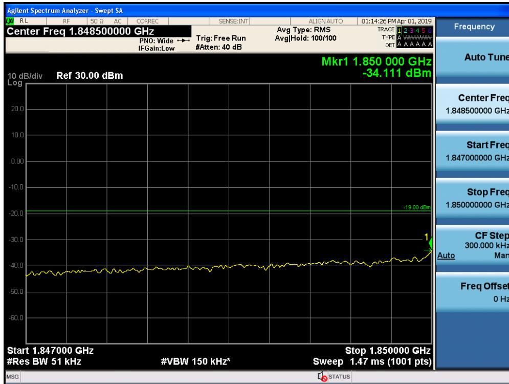
Out-of-Band Emissions / Broadband PCS / Uplink / LTE 5 MHz / Lower Edge / AGC threshold +10 dB
