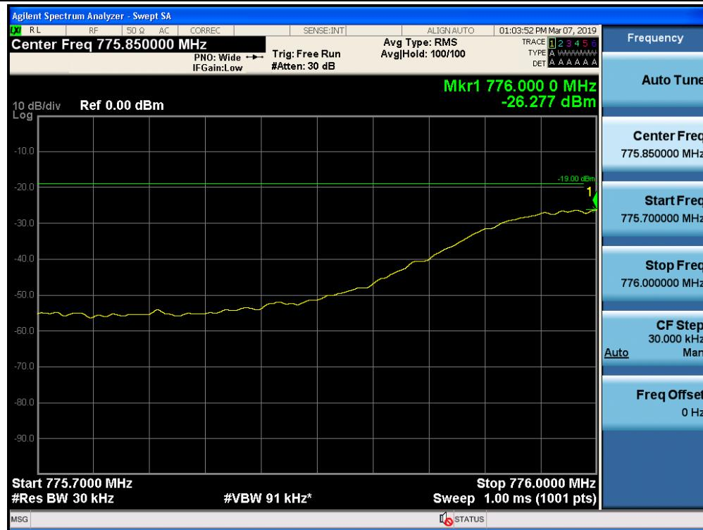
Out-of-Band Emissions / Upper 700 MHz / Uplink / LTE 5 MHz / Upper Edge / AGC threshold
