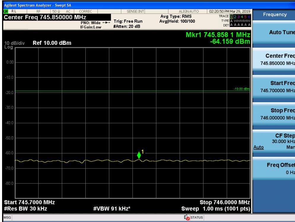
Out-of-Band Emissions / Cellular / Downlink / GSM / Upper Edge / AGC threshold
