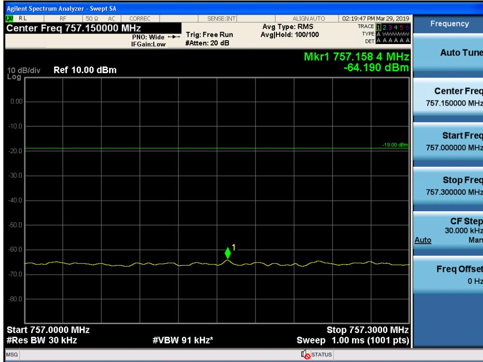
Out-of-Band Emissions / Upper 700 MHz / Downlink / CDMA / Lower Edge / AGC threshold
