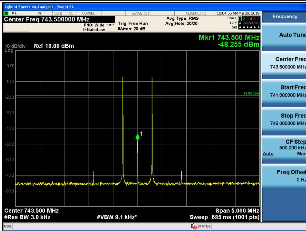
Intermodulation / Upper 700 MHz / Downlink / AGC threshold
