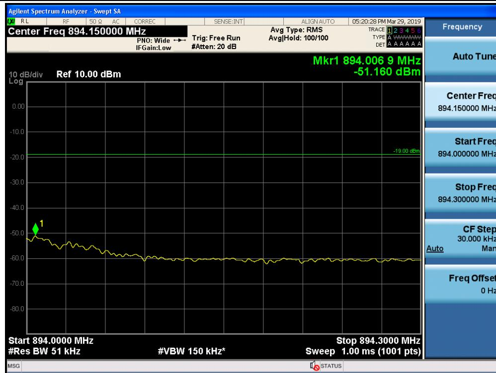
Out-of-Band Emissions / Cellular / Downlink / LTE 5 MHz / Upper Edge / AGC threshold +10 dB
