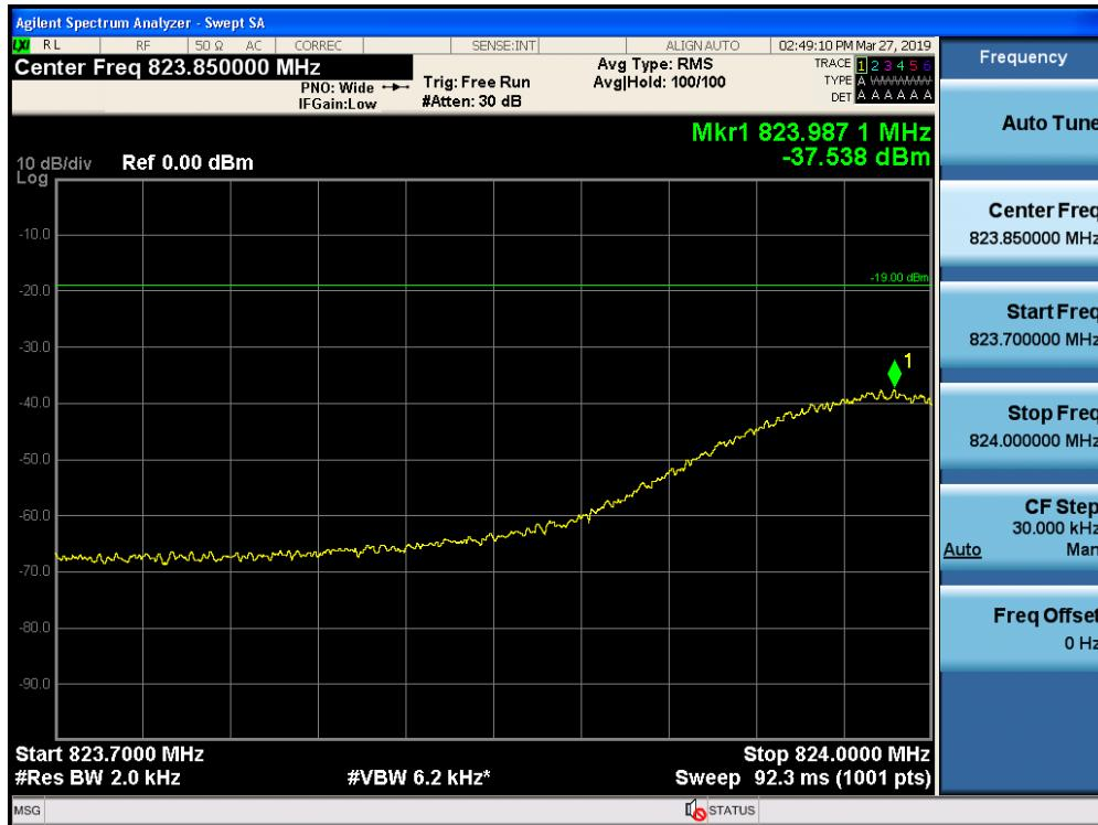
Out-of-Band Emissions / Cellular / Uplink / LTE 5 MHz / Upper Edge / AGC threshold
