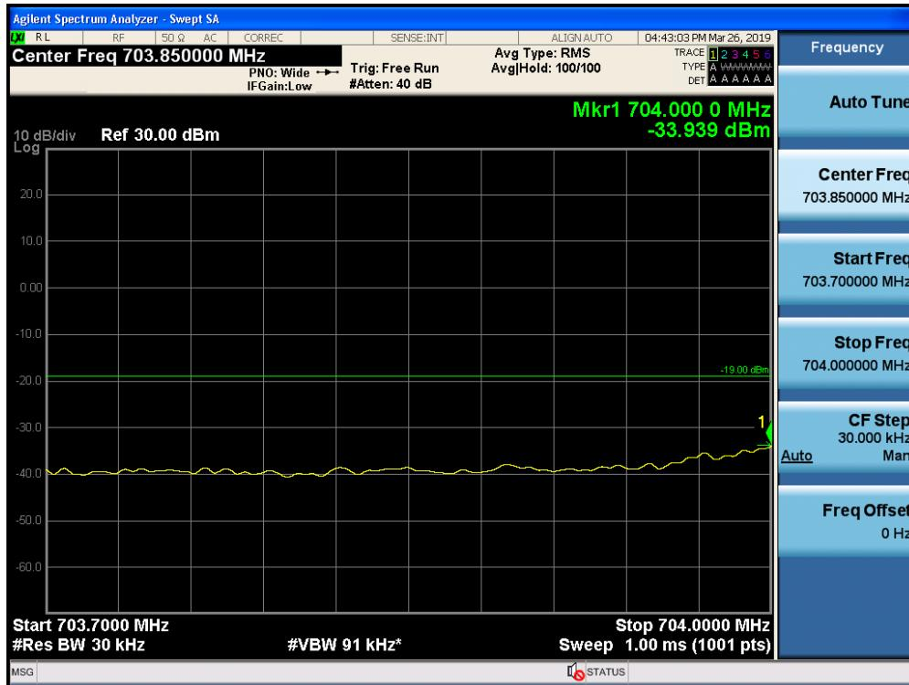
Out-of-Band Emissions / Lower 700 MHz / Uplink / LTE 5 MHz / Lower Edge / AGC threshold +10 dB
