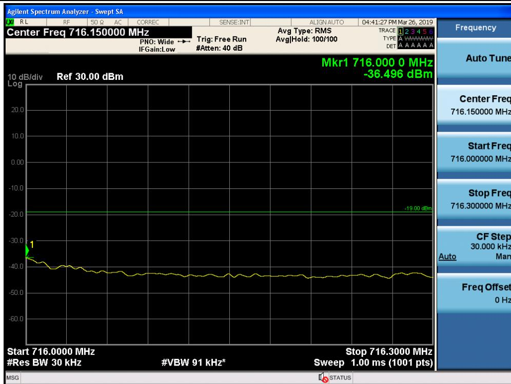
Out-of-Band Emissions / Lower 700 MHz / Uplink / LTE 5 MHz / Upper Edge / AGC threshold +10 dB
