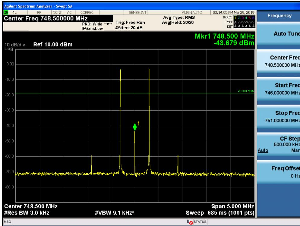
Intermodulation / Upper 700 MHz / Downlink / AGC threshold +10 dB
