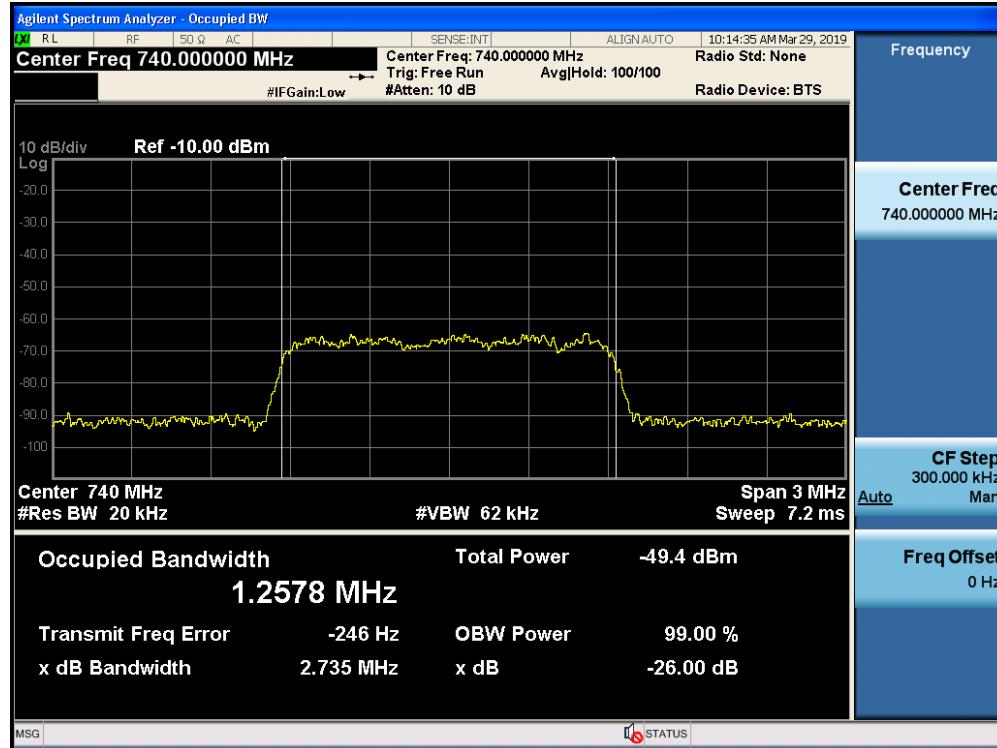
Occupied Bandwidth / Lower 700 MHz / Downlink / CDMA / Output
