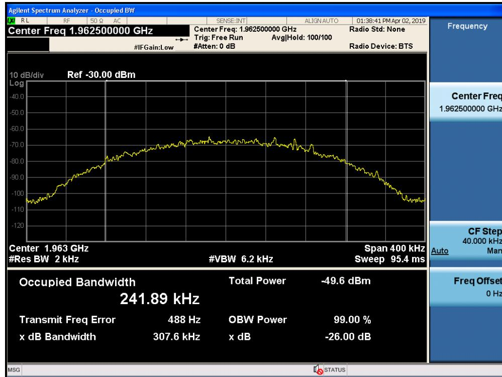
Occupied Bandwidth / Broadband PCS / Downlink / GSM / Output
