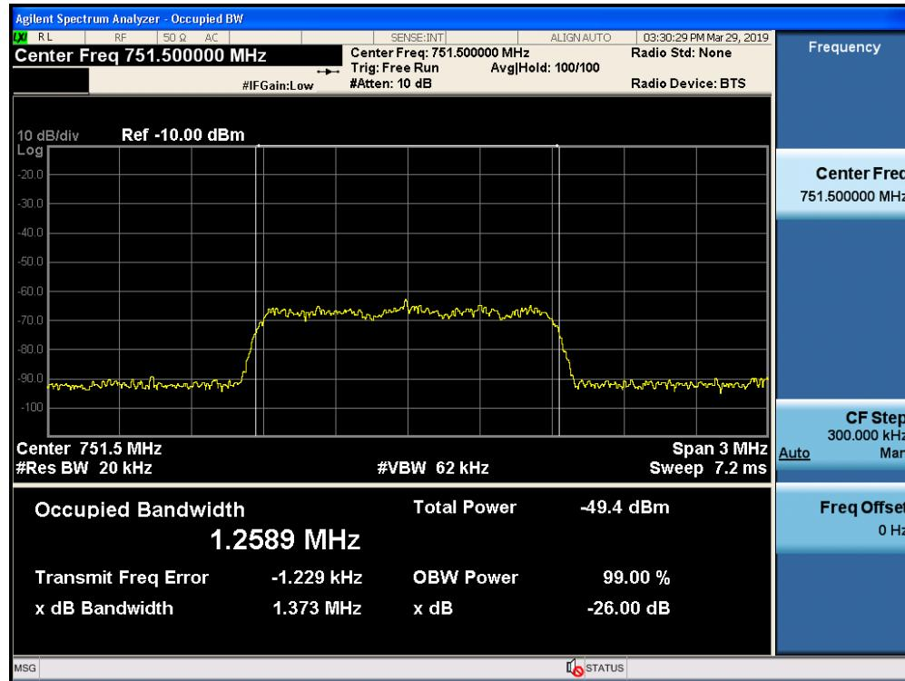
Occupied Bandwidth / Upper 700 MHz / Downlink / CDMA / Output
