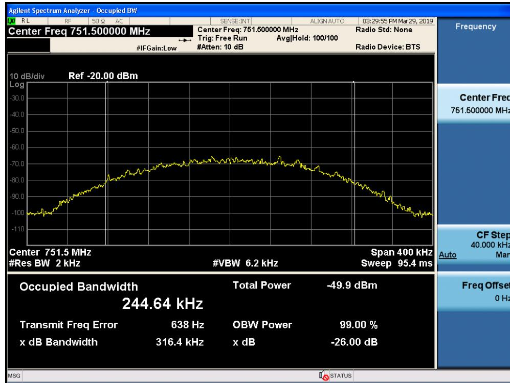
Occupied Bandwidth / Upper 700 MHz / Downlink / GSM / Output
