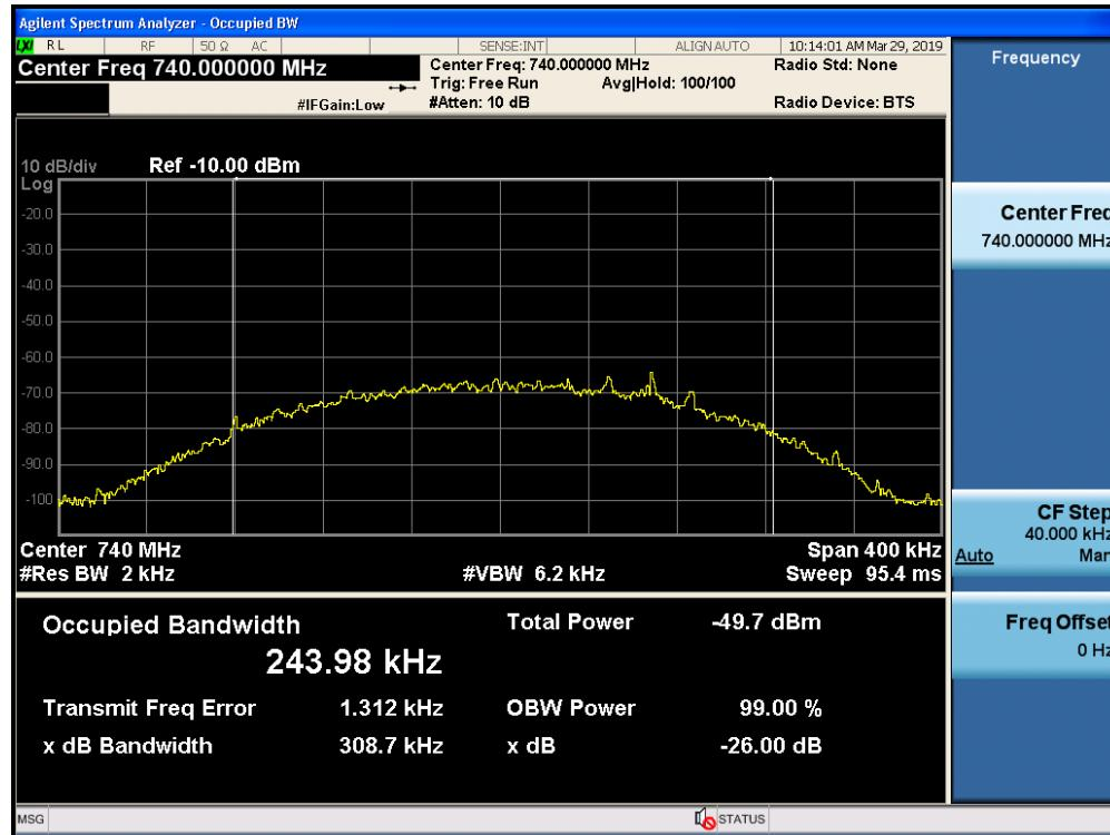
Occupied Bandwidth / Lower 700 MHz / Downlink / GSM / Output
