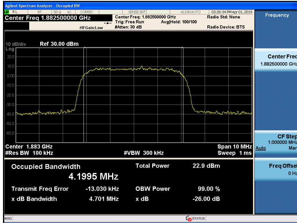
Occupied Bandwidth / Lower 700 MHz / Downlink / GSM / Input
