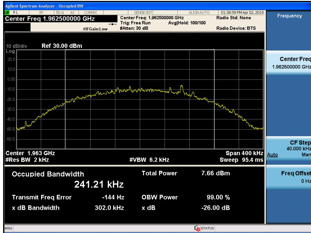
Occupied Bandwidth / Lower 700 MHz / Downlink / CDMA/ Input
