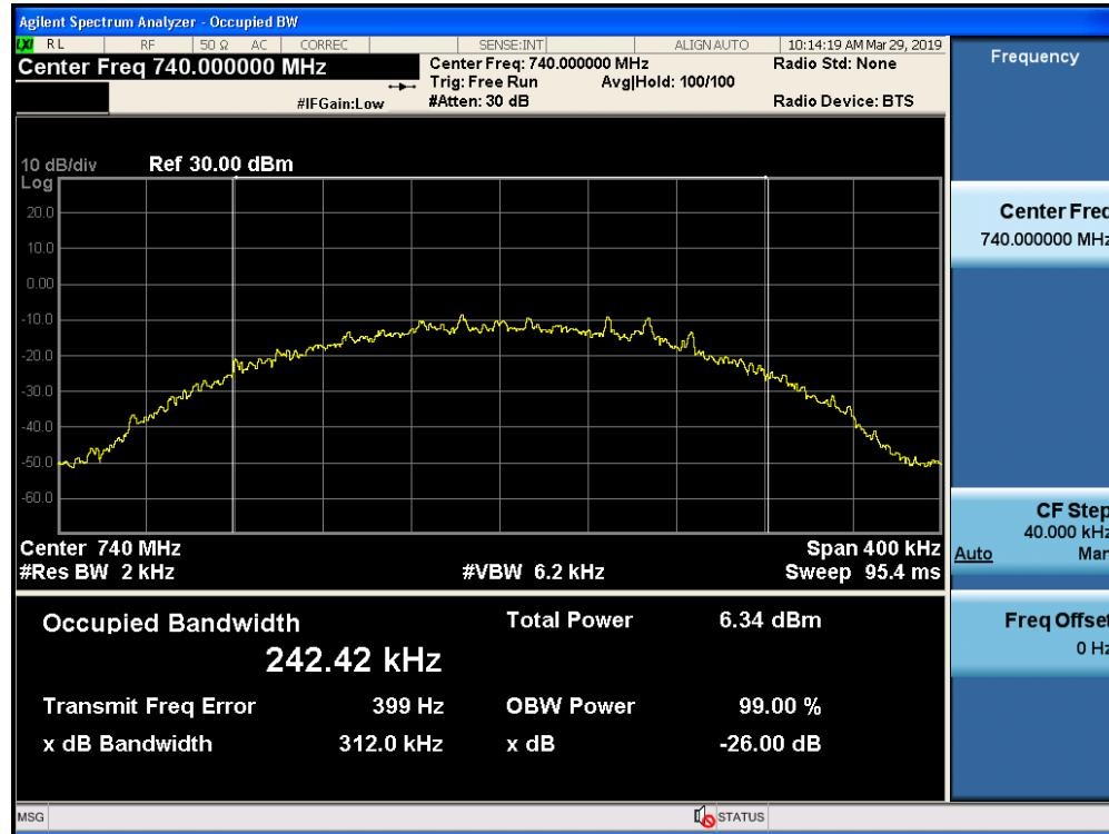
Occupied Bandwidth / Upper 700 MHz / Downlink / GSM / Input
