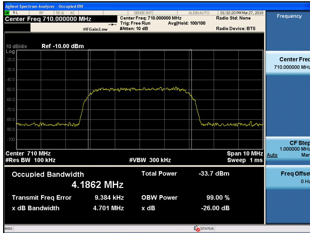
Occupied Bandwidth / Lower 700 MHz / Uplink / WCDMA / Output
