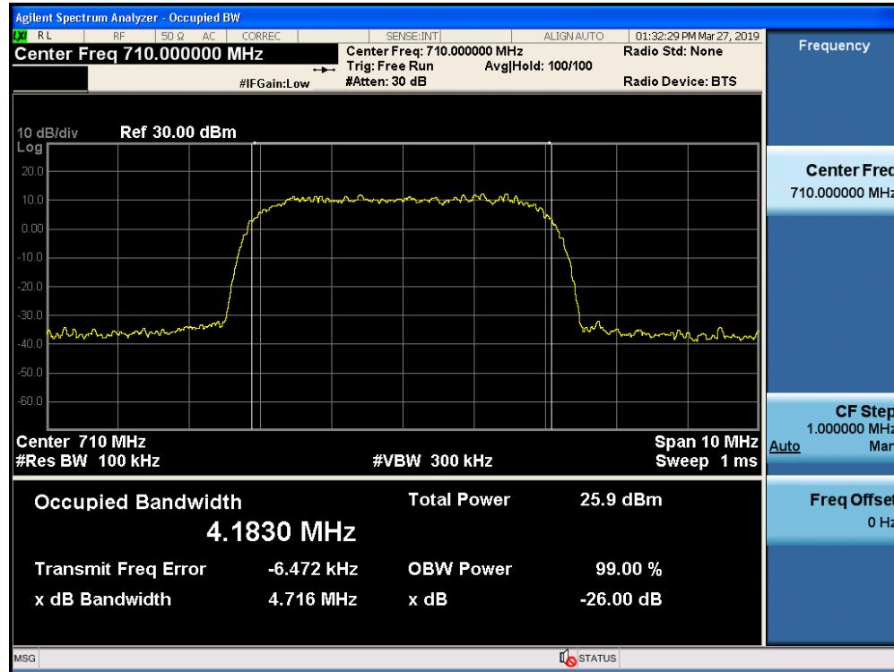
Occupied Bandwidth / Upper 700 MHz / Uplink / CDMA/ Input
