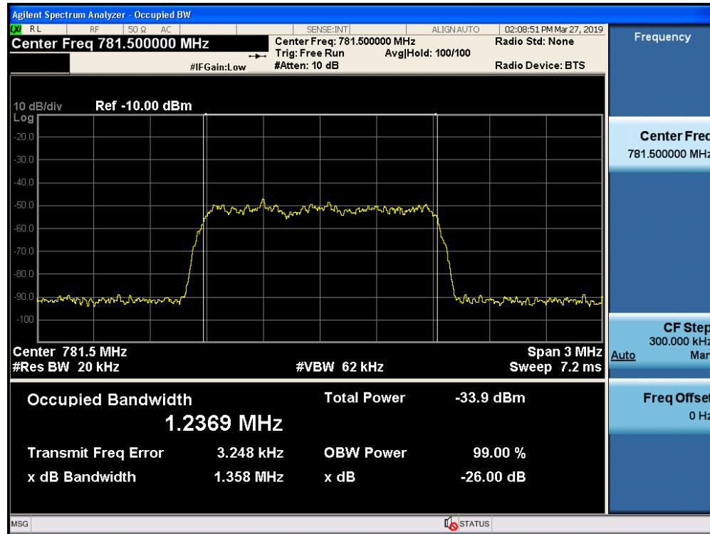
Occupied Bandwidth / Upper 700 MHz / Uplink / CDMA / Output
