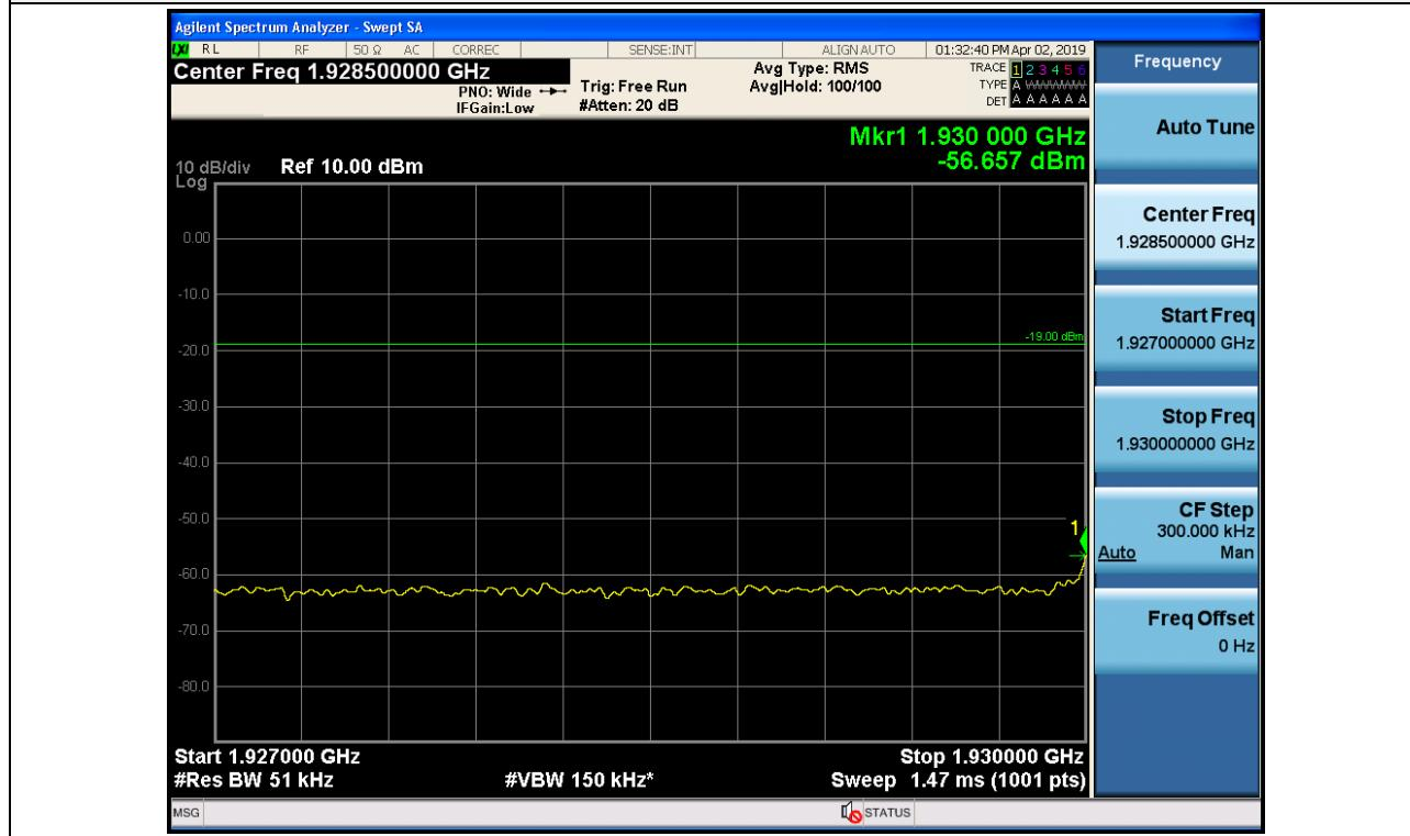
Out-of-Band Emissions / Broadband PCS / Downlink / LTE 5 MHz / Lower Edge / AGC threshold +10 dB
