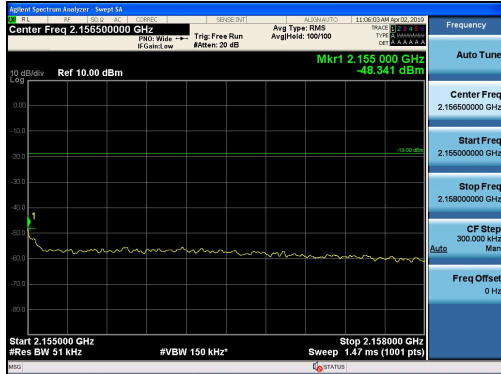
Out-of-Band Emissions / AWS-1 / Downlink / LTE 5 MHz / Upper Edge / AGC threshold +10 dB
