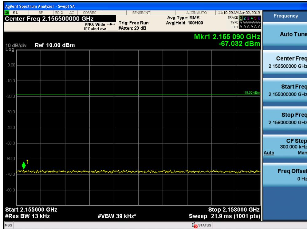
Out-of-Band Emissions / AWS-1 / Downlink / CDMA / Upper Edge / AGC threshold +10 dB
