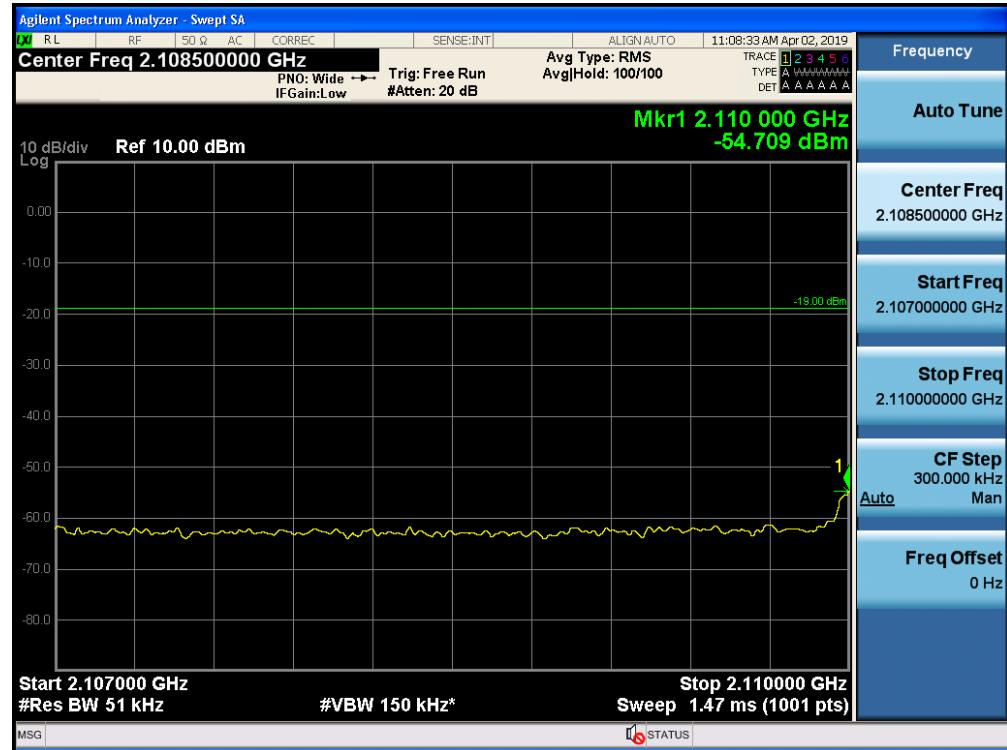
Out-of-Band Emissions / AWS-1 / Downlink / CDMA / Upper Edge / AGC threshold
