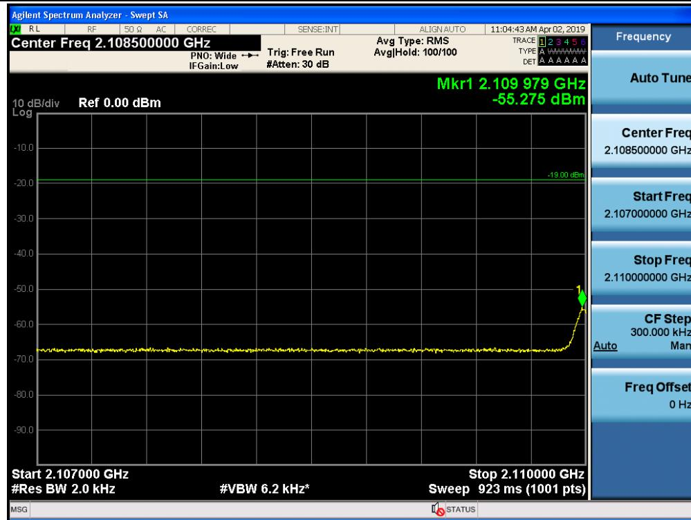
Out-of-Band Emissions / AWS-1 / Downlink / LTE 5 MHz / Upper Edge / AGC threshold
