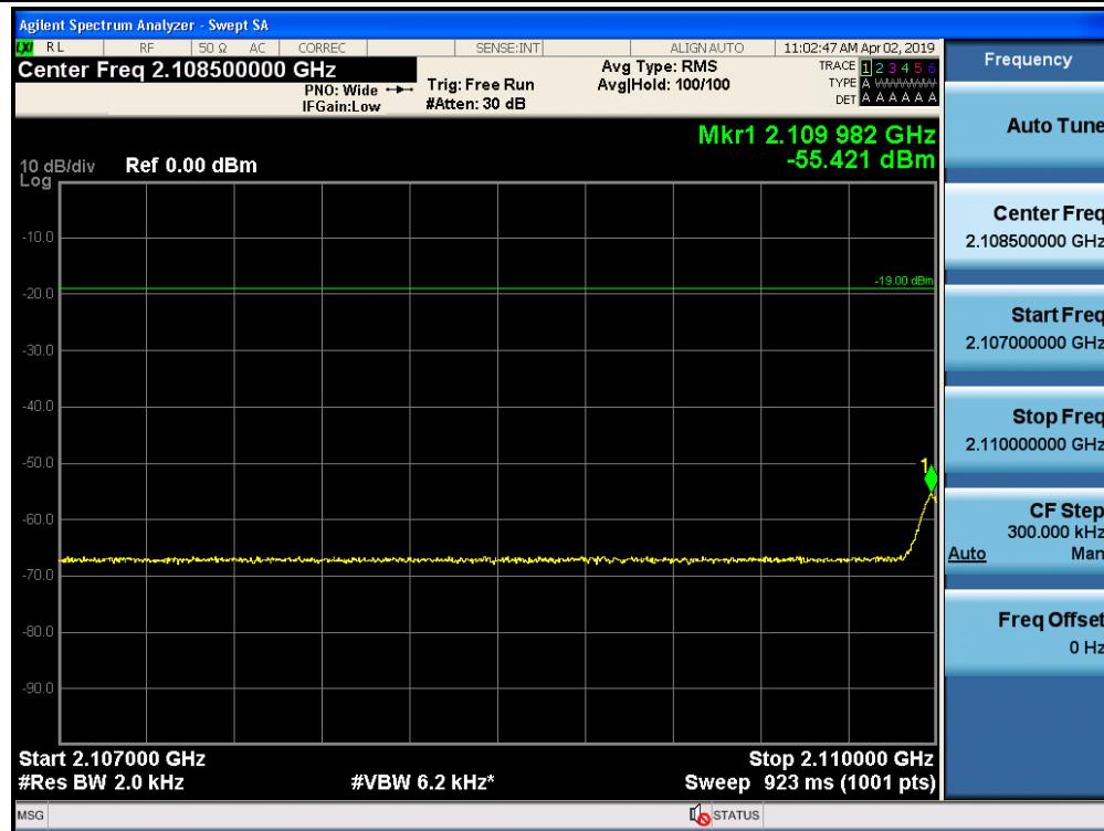
Out-of-Band Emissions / AWS-1 / Downlink / GSM / Lower Edge / AGC threshold +10 dB
