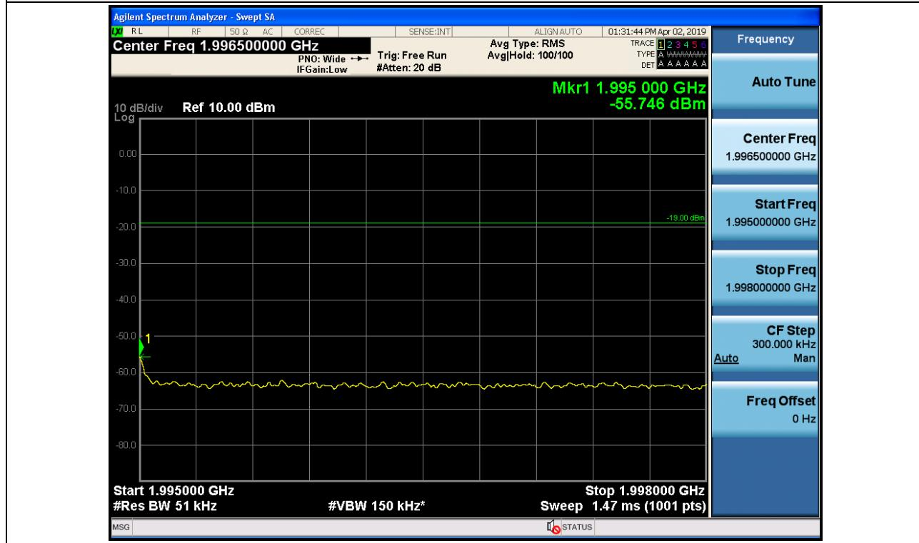
Out-of-Band Emissions / Broadband PCS / Downlink / LTE 5 MHz / Lower Edge / AGC threshold
