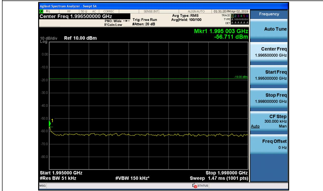
Out-of-Band Emissions / Broadband PCS / Downlink / LTE 5 MHz / Upper Edge / AGC threshold +10 dB
